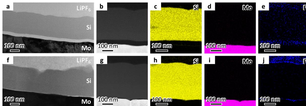
Fig. 4 Cross-sectional structures of the samples after 2nd discharge at  $V_d$  = (a)–(e) 2.0 V and (f)–(j) 0.6 V. (a) and (f) Bright-field TEM images, (b) and (g) HAADF-STEM images, and EDX mappings of (c) and (h) Si, (d) and (i) Mo, and (e) and (j) F.
