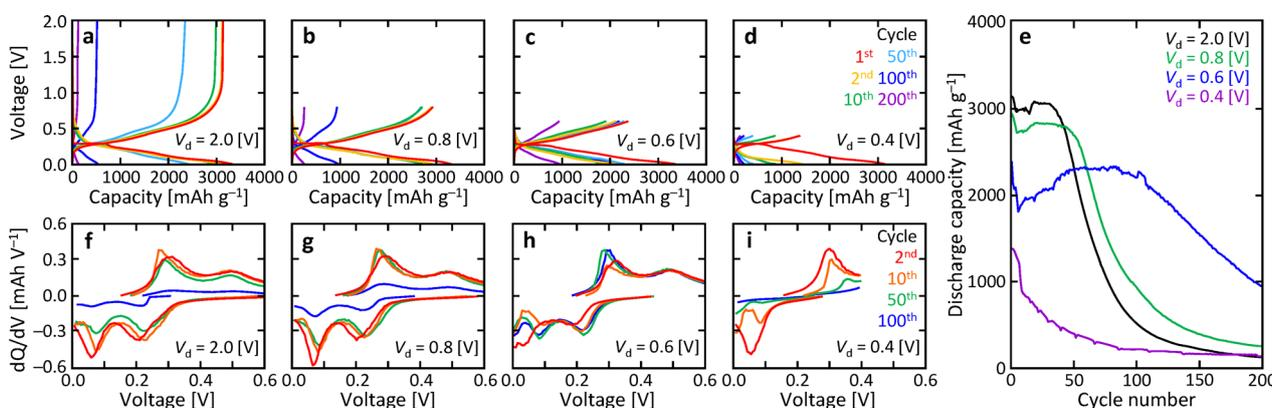
**Fig. 1** Delithiation cut-off voltage ( $V_d$ ) dependence of the anode properties. (a)–(d) Galvanostatic charge/discharge cycles at  $V_d$  = (a) 2.0 V, (b) 0.8 V, (c) 0.6 V, and (d) 0.4 V. (e) Cycle dependence of discharge capacities. (f)–(i)  $dQ/dV$  plots at  $V_d$  = (f) 2.0 V, (g) 0.8 V, (h) 0.6 V, and (i) 0.4 V.
