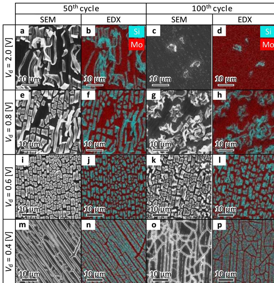
Fig. 2 SEM and EDX images of the sample surface after 50 and 100 charge/discharge cycles at different  $V_d$ : (a)–(d) 2.0 V, (e)–(h) 0.8 V, (i)–(l) 0.6 V, and (m)–(p) 0.4 V. In the EDX images, Si is shown in light blue and Mo in red.
