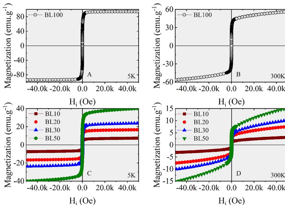
Fig. 16 Hysteresis loops of magnetization versus internal field intensity of BL100 record at 5 K (A) and 300 K (B) for a field cycle of  $0 \pm 50$  kOe. (C) and (D) Magnetic isotherms of the composites under similar conditions as BL100. Each isotherm has been corrected for demagnetization effects.
