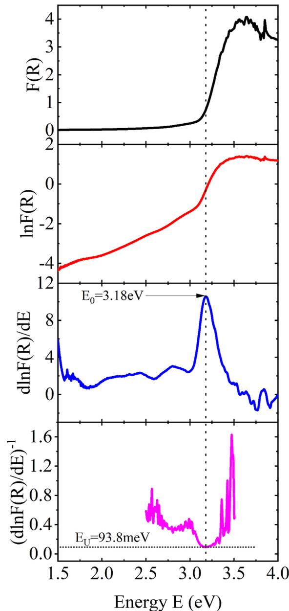
Fig. 12 Plots of  $F(R)$ ,  $\ln F(R)$ , the first-order derivative of  $\ln F(R)$  with respect to energy, and the inverse of this derivative for the estimation of the Urbach focus and Urbach energy,  $E_0$  and  $E_U$ .
