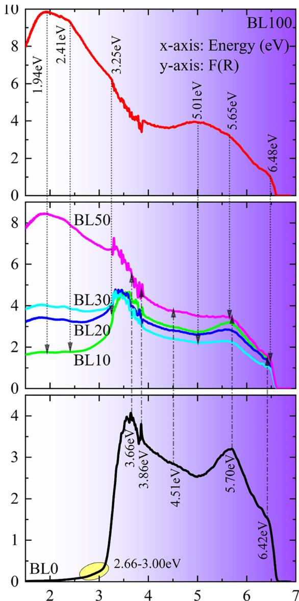
Fig. 9 Variation in  $F(R)$  plotted as a function of  $E$  in the energy range of 1.5 eV to 7 eV for  $(1-x)\text{BaTiO}_3:(x)\text{La}_{0.835}\text{Na}_{0.165}\text{MnO}_3$  ( $x = 0, 10, 20, 30, 50,$  and  $100$ ).
