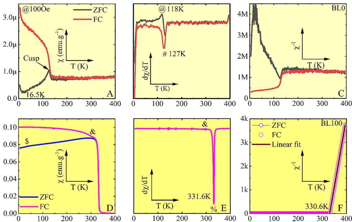
**Fig. 13** Temperature dependence of the magnetic susceptibility of BL0 (A) and BL100 (D) measured in zero-field cooled and field-cooled mode at a magnetization intensity of 100 Oe. The  $d\chi/dT$  (BL0:B and BL100:E) indicates the different inflection points in the susceptibility curve. The inverse susceptibility (BL0:C and BL100:F) is used to depict the typical magnetic nature of the specimens.
