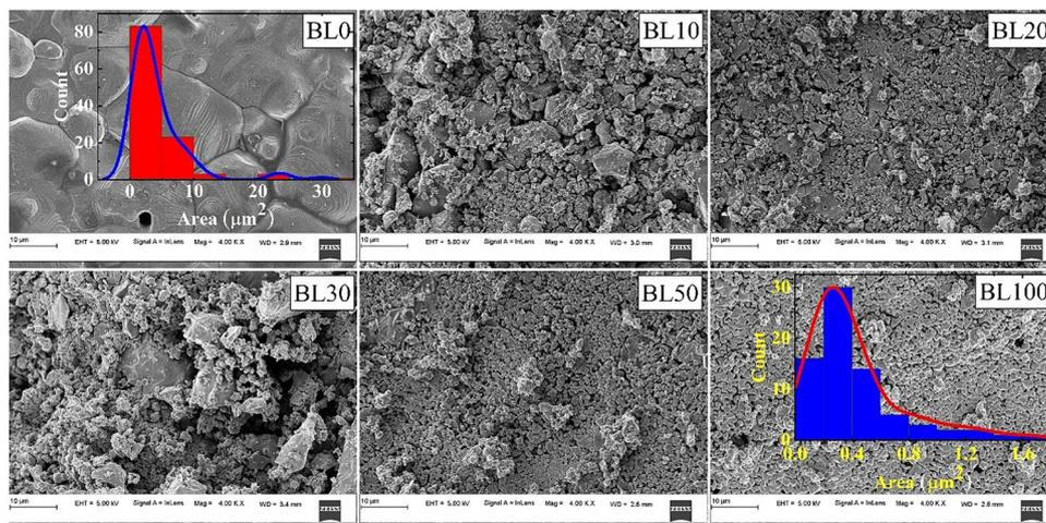
Fig. 4 FESEM micrographs of  $(1-x)\text{BTO}:x(\text{LNMO})$ ,  $x = 0, 10, 20, 30, 50$  and  $100$ , recorded at  $4.00\text{k}\times$  magnification. The histograms show the grain size distribution of BL0 and BL100 under lognormal distribution. The columns represent counts per scale; the overlaid curve is the kernel-smoothed representation of the respective distribution.
