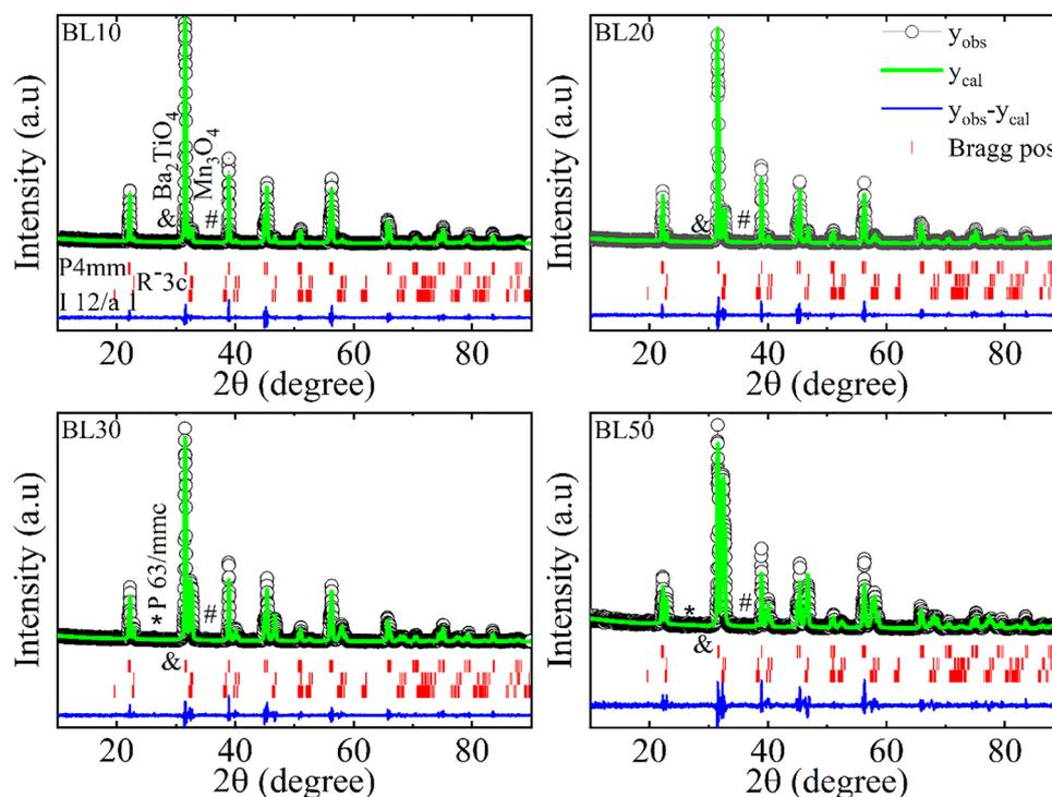
Fig. 3 Rietveld-refined powder XRD patterns of BL10, BL20, BL30 and BL50. The respective SG are indicated to the left of the Bragg positions.
