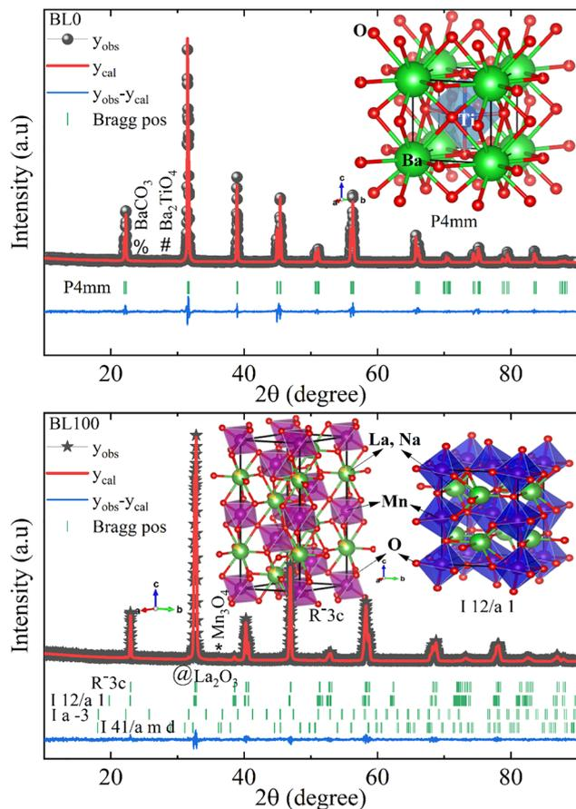
Fig. 2 Rietveld-refined powder XRD patterns of BL0 and BL100. Symbols (bubbles and asterisks) represent the observed data ( $y_{\text{obs}}$ ), the overlaid solid curve corresponds to the calculated profile ( $y_{\text{cal}}$ ), the vertical bars indicate the Bragg peak positions (Bragg pos) and the nearly horizontal line at the bottom represents the difference curve ( $y_{\text{obs}} - y_{\text{cal}}$ ). The respective SG are marked on the left of the Bragg positions.
