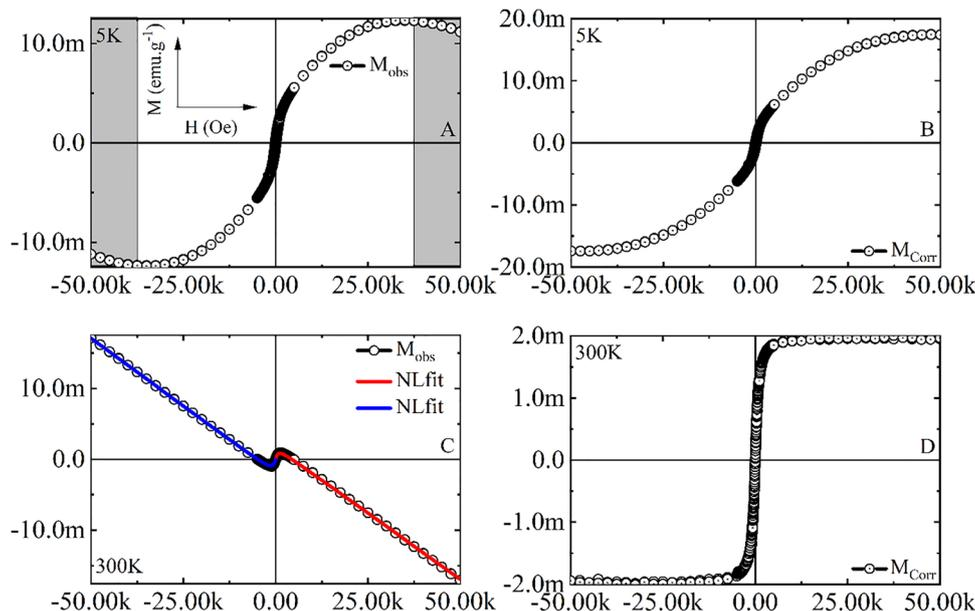
Fig. 15 Hysteresis loops of magnetization versus applied field intensity of BL0 record at 5 K (A) and 300 K (C) for a field cycle of  $0 \pm 50$  kOe. Each isotherm is corrected for high-field diamagnetic contributions ((B) and (D), respectively) using linear and nonlinear fitting.
