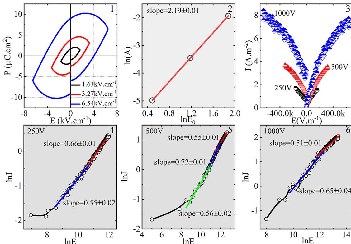
**Fig. 18** (1) Plot of electric polarization versus electric field under the bias voltages of 250 V (1.63 kV  $\text{cm}^{-1}$ ), 500 V (3.27 kV  $\text{cm}^{-1}$ ) and 1000 V (6.54 kV  $\text{cm}^{-1}$ ). (2) Log-log plot of the area under the loop versus  $E_0$ . (3). Variation in current density with applied potential. (4)–(6) Log-log plots of current density versus  $E$  to understand the various conduction mechanisms that drive current in the BL10 specimen.
