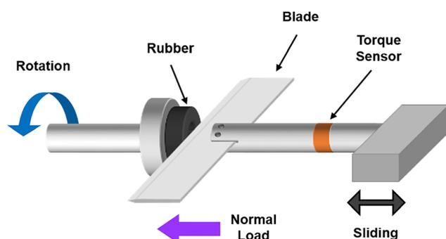
Fig. 2 Sketch of blade abrader.<sup>38–40</sup>
