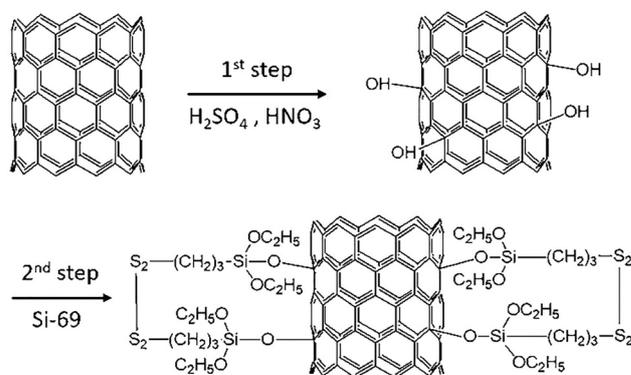
Fig. 1 Modification of CNTs with H<sub>2</sub>SO<sub>4</sub>, HNO<sub>3</sub>, and the silane coupling agent (Si-69).
