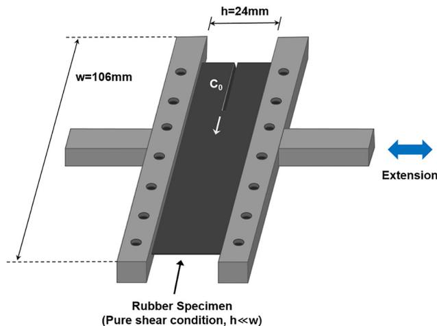
Fig. 3 Sketch of the crack growth experiment under pure shear conditions.<sup>41</sup>
