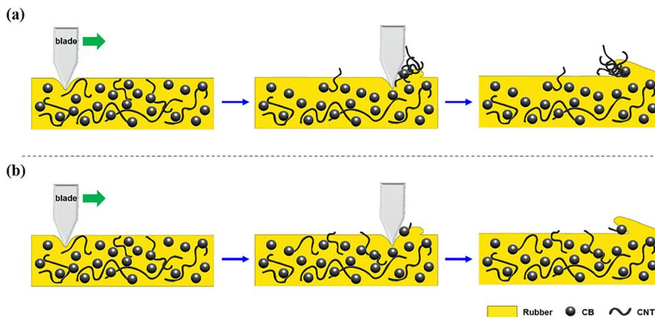
Fig. 8 Schematic representation of the abrasion behavior of SBR composites with (a) p-CNT and (b) T-CNT.
