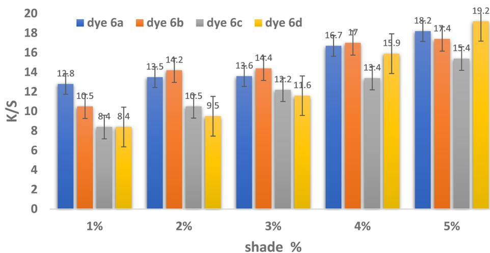
Fig. 5 Shade and color strength ( $K/S$ ) relationship for dyes **6a–d** (temperature = 130 °C, pH = 2 for dyes **6a–c** and pH = 4 in the case of dye **6d**, and duration = 60 min for dyes **6a, b, and d** and duration = 45 min for dye **6c**).
