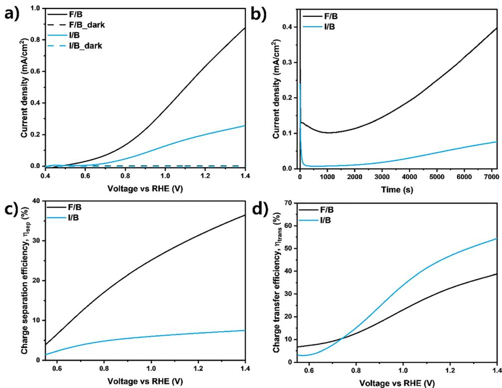
Fig. 5 (a)  $J-V$  curves obtained via linear sweep voltammetry (LSV) under illumination (solid lines) and in the dark (dotted lines), (b)  $J-t$  curves measured at 0.8 V<sub>RHE</sub>, (c) charge separation and (d) transfer efficiencies measured in the presence of hole scavenger (Na<sub>2</sub>SO<sub>3</sub>) in the electrolyte. Data for the F/B (black) and the I/B (blue) films.
