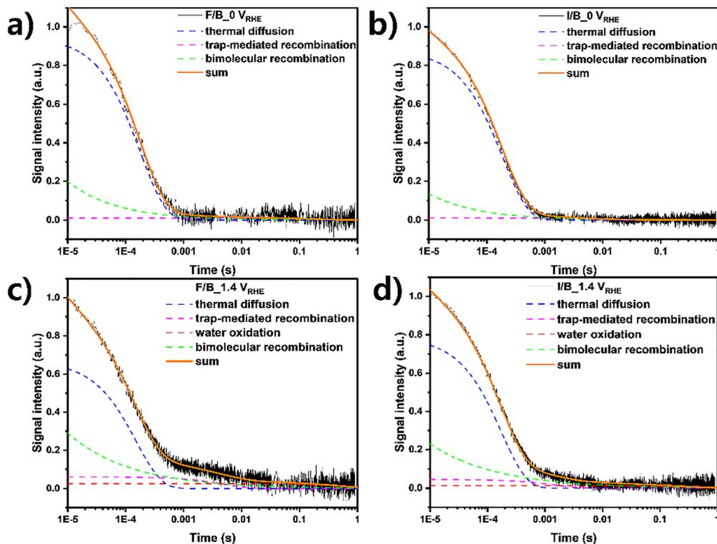
Fig. 10 NF-HD-TG responses of (a) the F/B, (b) the I/B at 0  $V_{\text{RHE}}$ , (c) the F/B, and (d) the I/B at 1.4  $V_{\text{RHE}}$  at the grating spacing ( $\Lambda$ ) of 30  $\mu\text{m}$  with fitting curves.
