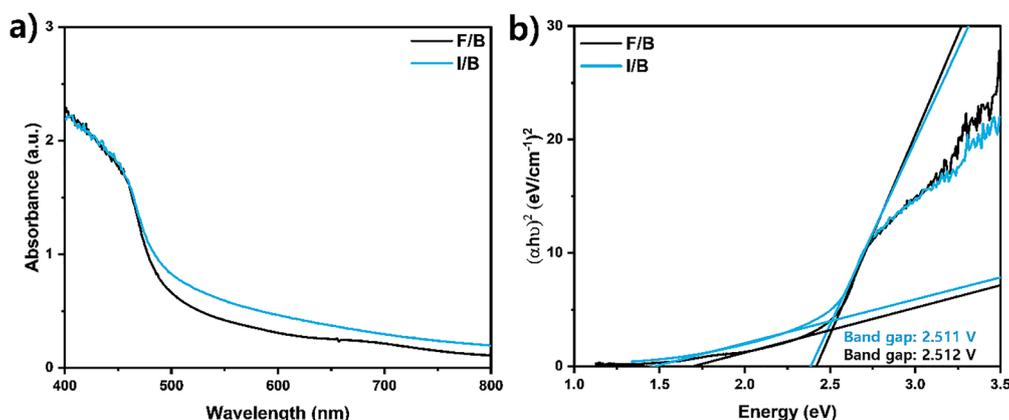
Fig. 3 (a) Absorption spectra obtained from UV-vis measurements in the 400–800 nm range, and (b) the Tauc plots of the F/B and the I/B films.
