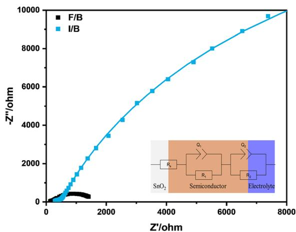
Fig. 8 The Nyquist plots of the F/B (black) and the I/B (blue), measured at 0.5 V<sub>RHE</sub>; the inset displays the equivalent circuit diagram used for fitting.
