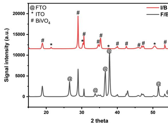
Fig. 1 XRD patterns of F/B (black) and I/B (red) films. The @ sign corresponds to the diffraction peaks arising from  $\text{SnO}_2$  of the FTO substrate (JCPDS No. 01-079-6887), the asterisk (\*) indicates the diffraction peaks of  $\text{In}_2\text{O}_3$  originating from the ITO substrate (JCPDS No. 01-089-4597) and the hash (#) corresponds to the  $\text{BiVO}_4$  (JCPDS No. 14-0688).
