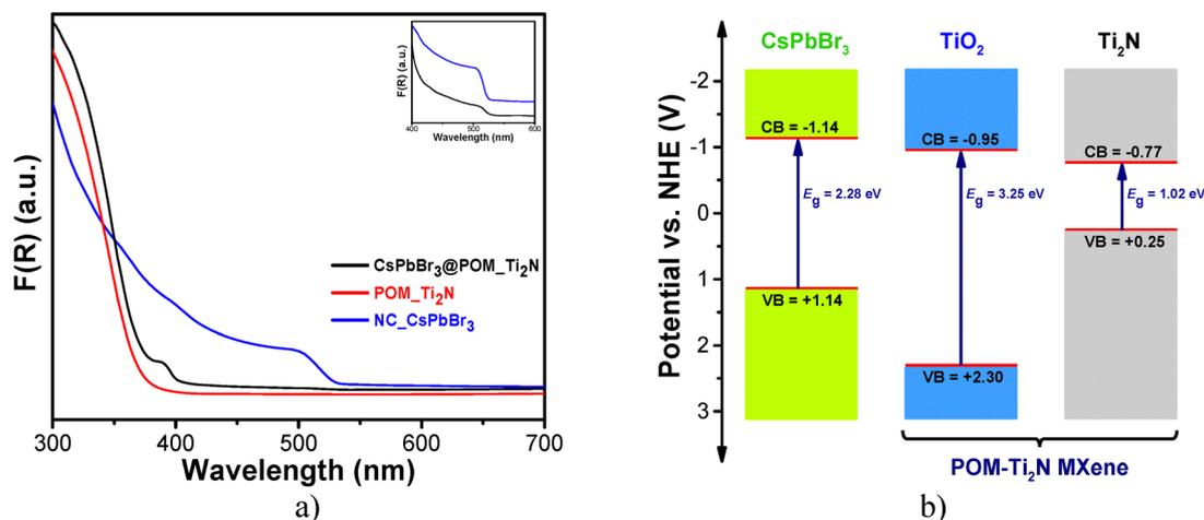
Fig. 3 (a) Diffuse reflectance UV-vis optical spectra of CsPbBr<sub>3</sub> NCs, the Ti<sub>2</sub>N MXene and the supported material. The inset shows a magnification in the characteristic range of the CsPbBr<sub>3</sub> NCs absorption. (b) Schematic energy band level diagram of each component of the CsPbBr<sub>3</sub>@POM-Ti<sub>2</sub>N composite. The respective CB and VB values, as well as the optical band gaps (all in eV), are extracted from the XPS and UV-vis measurements respectively.
