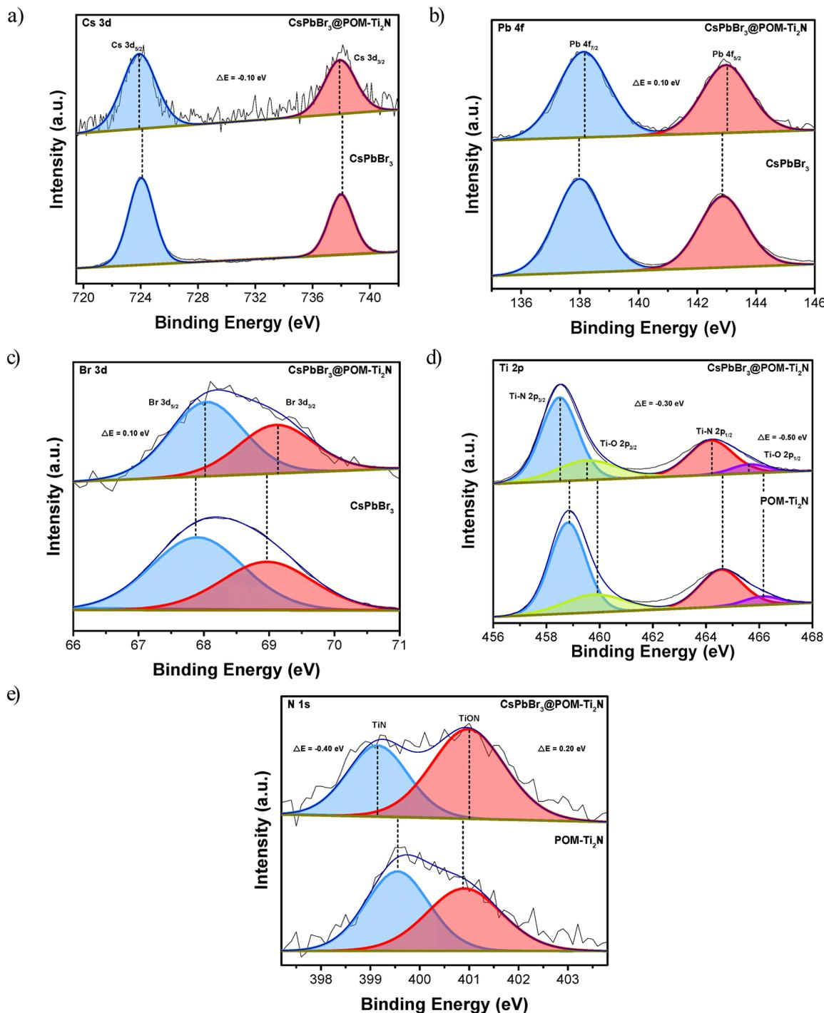
Fig. 5 XPS spectra of CsPbBr<sub>3</sub> NCs, POM-Ti<sub>2</sub>N (below), and NCs@POM-Ti<sub>2</sub>N composites (top): (a) Cs 3d spectra, (b) Pb 4f spectra, (c) Br 3d spectra, (d) Ti 2p spectra, and (e) N 1s spectra.
