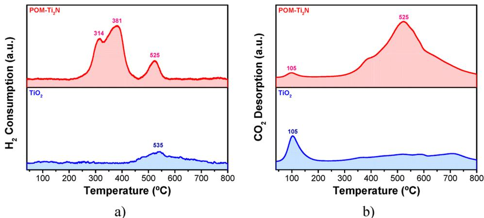
Fig. 6 (a)  $\text{H}_2$ -TPR analysis profiles of the tested materials: POM- $\text{Ti}_2\text{N}$  (red line) and  $\text{TiO}_2$  (blue line). (b)  $\text{CO}_2$ -TPD profiles obtained on POM- $\text{Ti}_2\text{N}$  (red line) and  $\text{TiO}_2$  (blue line) materials. In both studies, the ramp rate was  $10\text{ }^\circ\text{C min}^{-1}$ .
