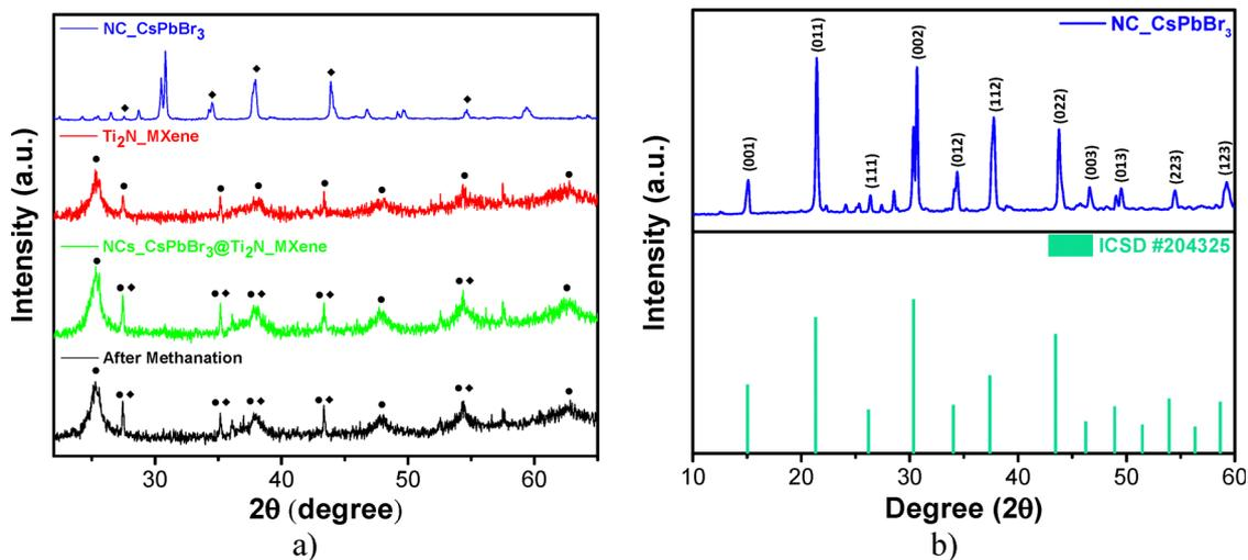
Fig. 1 (a) Comparative XRD patterns of CsPbBr<sub>3</sub> NCs (blue), POM–Ti<sub>2</sub>N MXene (red), NCs@POM–Ti<sub>2</sub>N before (green) and after the catalytic reaction (black), (b) CsPbBr<sub>3</sub> NCs compared with reference data from the ICSD #204325 data file.
