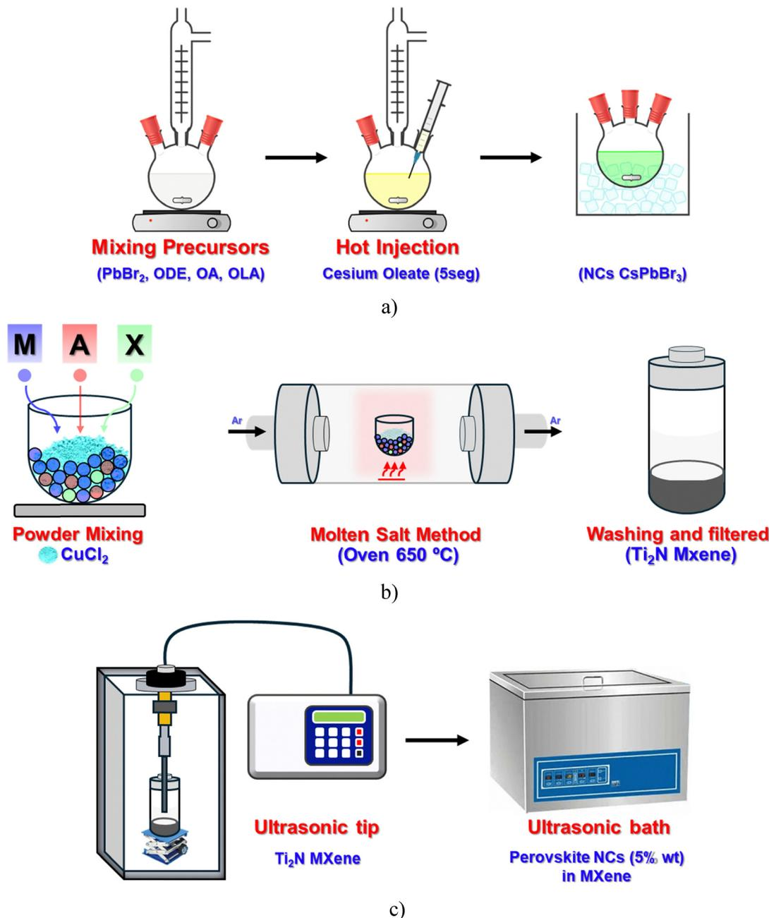
**Scheme 1** Synthetic procedure for the preparation of the catalyst. (a) Preparation of the  $\text{CsPbBr}_3$  NCs, (b) formation of the  $\text{Ti}_2\text{N}$  MXene from the MAX phase and (c) the impregnation process for the deposition of the  $\text{CsPbBr}_3$  NCs on the exfoliated  $\text{Ti}_2\text{N}$  MXene.
