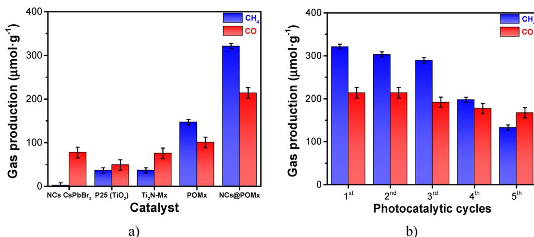
**Fig. 8** (a) Comparison of photocatalytic activity for different samples. (b) Recycling of the photocatalyst CsPbBr<sub>3</sub>(5 wt%)/POM-Ti<sub>2</sub>N MXene. Reaction conditions: photocatalyst (10 mg),  $P_{\text{H}_2} = 1.2$  bar,  $P_{\text{CO}_2} = 0.3$  bar, at 23 h reaction time, simulated sunlight irradiation (226 mW cm<sup>-2</sup>), and 200 °C.
