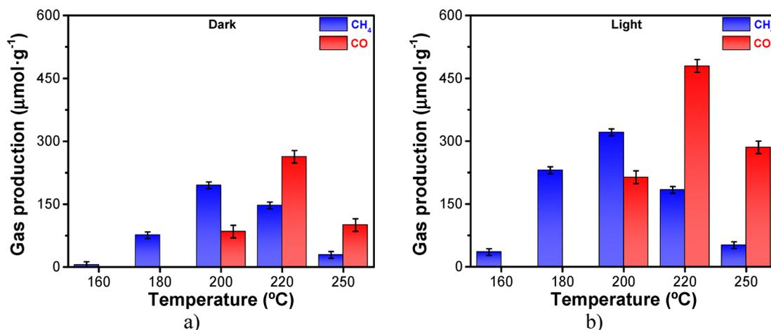
Fig. 7 Photocatalytic activity of  $\text{CsPbBr}_3(5\text{ wt\%})@POM\text{-Ti}_2\text{N}$  MXene under different conditions of temperature (a) in the dark and (b) under light irradiation. Reaction conditions:  $\text{CsPbBr}_3(5\text{ wt\%})@POM\text{-Ti}_2\text{N}$  MXene (10 mg),  $P_{\text{H}_2} = 1.2\text{ bar}$ ,  $P_{\text{CO}_2} = 0.3\text{ bar}$ , at 23 h reaction time, simulated sunlight irradiation ( $226\text{ mW cm}^{-2}$ ), and temperature as indicated.
