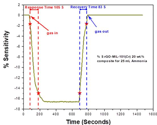
Fig. 13 Response and recovery times for ammonia gas using the rGO-20 wt% MIL-101(Cr) composite.
