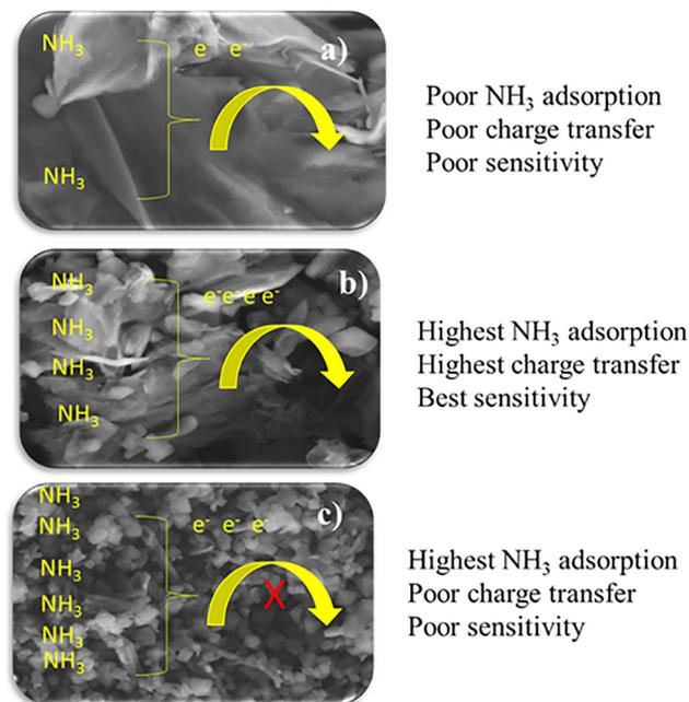
Fig. 15  $\text{NH}_3$  sensing mechanism using (a) the rGO-2.5 wt% MIL-101(Cr) composite, (b) the rGO-20 wt% MIL-101(Cr) composite and (c) the rGO-80 wt% MIL-101(Cr) composite.
