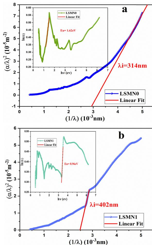
Fig. 8 Variation of  $(\alpha/\lambda)^2$  as a function of  $1/\lambda$  for the determination of the threshold wavelength ( $\lambda_i$ ) of LSMN0 and LSMN1. The inset shows  $\ln(\alpha)$  as a function of photon energy ( $h\nu$ ) for the determination of the Urbach energy ( $E_u$ ).
