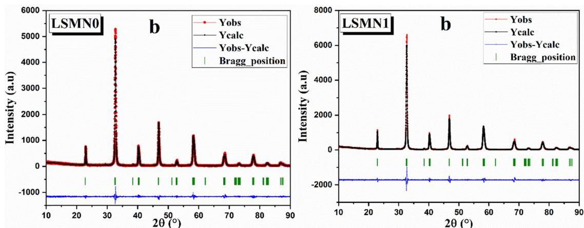
Fig. 1 (a) XRD patterns of LSMN0 and LSMN1 compounds indexed to the rhombohedral  $R\bar{3}c$  phase (Ref. Cod: 96-152-1757). The inset shows the most peak shift between the two samples. (b) Rietveld refinement profiles of LSMN0 and LSMN1.
