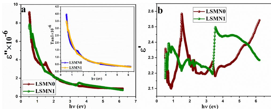
Fig. 13 (a) Imaginary part of the dielectric permittivity ( $\epsilon''$ ) versus photon energy ( $h\nu$ ) for LSMN0 and LSMN1. Inset: Loss tangent ( $\tan \delta$ ) versus  $h\nu$  for both samples. (b) Variation of the real part of the dielectric permittivity ( $\epsilon'$ ) versus  $h\nu$  for LSMN0 and LSMN1 ( $x = 0$  and  $x = 0.05$ ).
