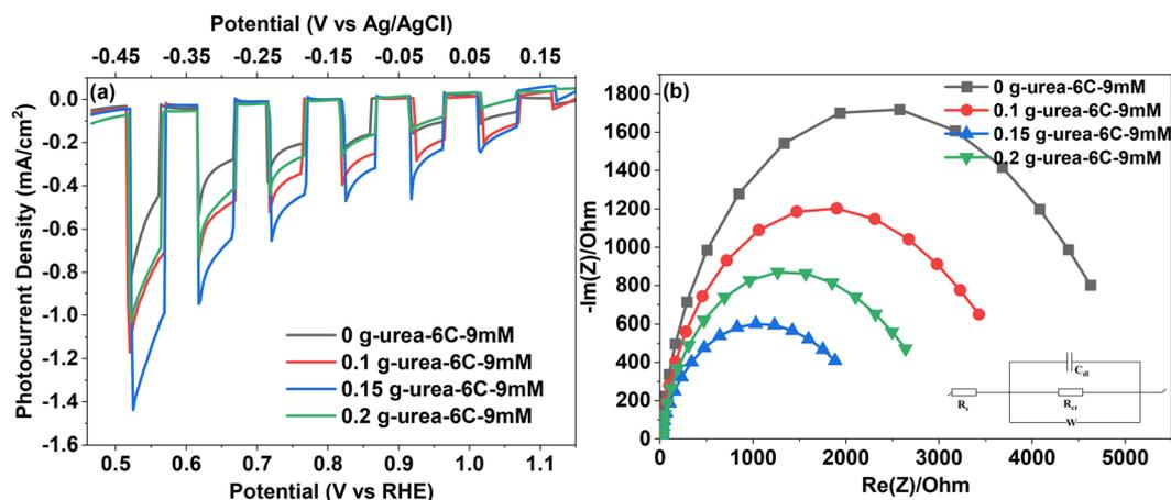
Fig. 8 (a) Photocurrent density-potential vs. RHE or Ag/AgCl ( $J$ - $V$ ) plots under chopped illumination conditions, (b) ESI Nyquist plots obtained at  $-0.45$  V vs. Ag/AgCl under one sun simulated light illumination.
