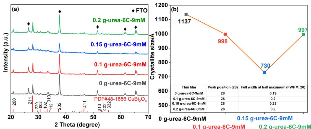
Fig. 1 (a) XRD patterns and (b) corresponding crystallite size of different  $\text{CuBi}_2\text{O}_4$  thin films deposited on an FTO substrate.
