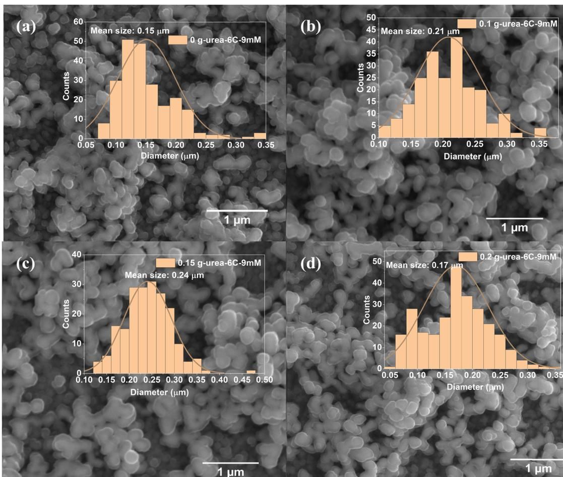
Fig. 2 SEM images of the top view and particle size distribution histograms of the resulting  $\text{CuBi}_2\text{O}_4$  thin films on FTO substrates: (a) 0 g-urea-6C-9mM; (b) 0.1 g-urea-6C-9mM; (c) 0.15 g-urea-6C-9mM; and (d) 0.2 g-urea-6C-9mM.
