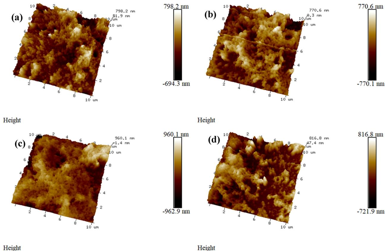
Fig. 4 AFM 3D perspectives of (a) 0 g-urea-6C-9mM, (b) 0.1 g-urea-6C-9mM, (c) 0.15 g-urea-6C-9mM, and (d) 0.2 g-urea-6C-9mM.
