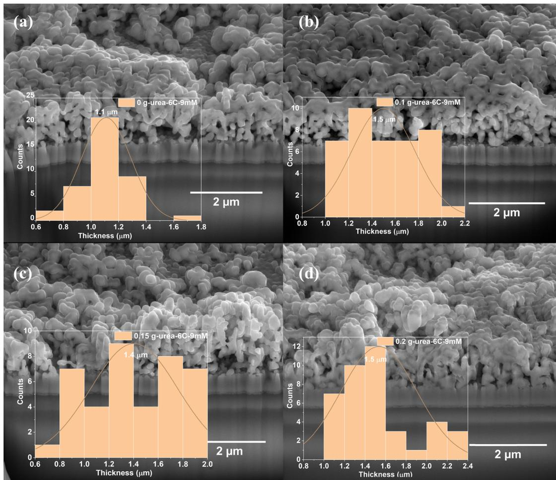
Fig. 3 SEM images of cross-section views and thickness histograms of the resulting  $\text{CuBi}_2\text{O}_4$  thin films on FTO substrates: (a) 0 g-urea-6C-9mM; (b) 0.1 g-urea-6C-9mM; (c) 0.15 g-urea-6C-9mM; and (d) 0.2 g-urea-6C-9mM.
