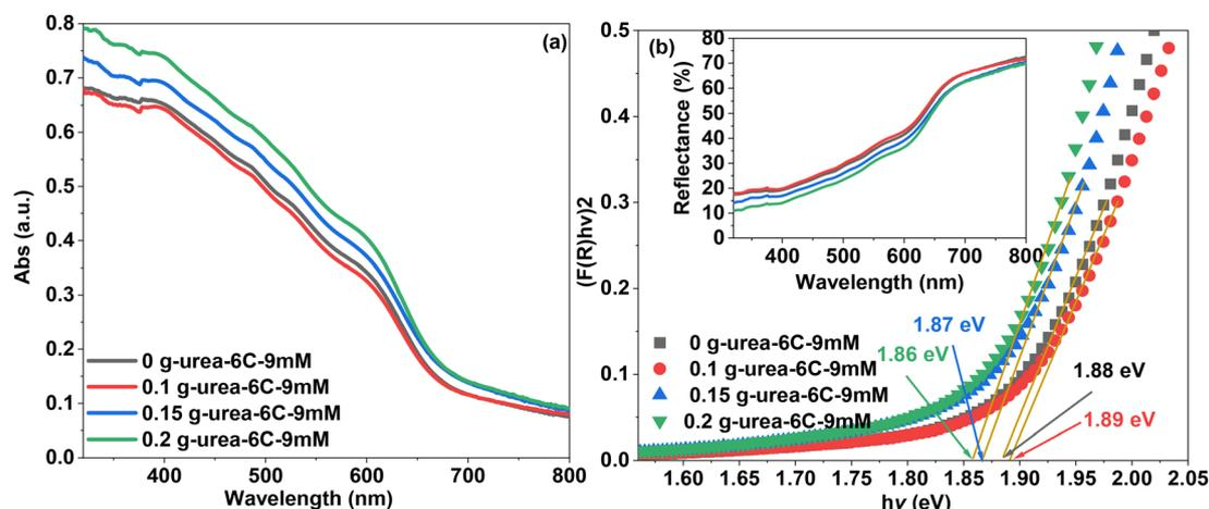
Fig. 6 (a) UV-visible absorbance spectra of the  $\text{CuBi}_2\text{O}_4$  thin films and (b) the corresponding predicted band gap values from the Kubelka–Munk function,<sup>53</sup> with the UV-visible diffuse reflectance spectra (DRS) shown in the inset.
