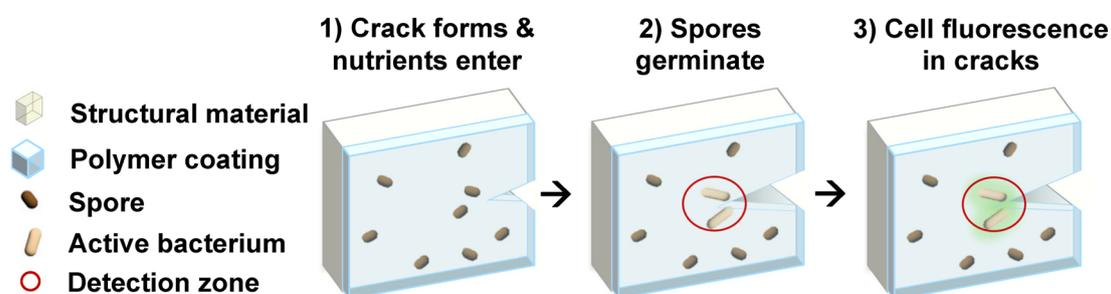
Fig. 1 Schematic of crack detection mechanism for a structural material based on a spore-polymer coating. When the structural material undergoes plastic deformation or initiation of a ductile fracture process, the coating cracks, allowing nutrients to enter and leading to spore germination. The spores then germinate into vegetative cells that fluoresce, enabling crack detection *via* fluorescence imaging.
