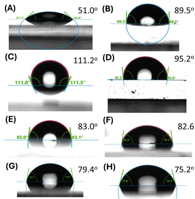
Fig. 6 Contact angle measurements on different epoxy coating surfaces. (A) epoxy, (B) epoxy + GO (0.01 wt%), (C) epoxy + Eu-PMHS-GO (0.001 wt%), (D) epoxy + Eu-PMHS-GO (0.005 wt%), (E) epoxy + Eu-PMHS-GO (0.01 wt%), (F) epoxy + Eu-PMHS-GO (0.05 wt%), (G) epoxy + Eu-PMHS-GO (0.1 wt%), and (H) epoxy + Eu-PMHS-GO (0.5 wt%).
