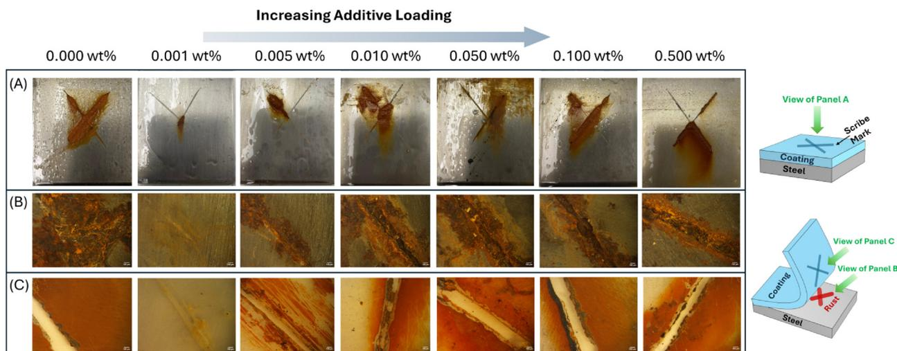
Fig. 8 Photographic images of scratched epoxy-coated carbon steels after immersion in seawater for 90 days. The weight percent loadings of **Eu-PMHS-GO** are indicated. Panel A: top surface of the intact coating around the scribe mark; panel B: exposed steel (around the scribe mark) after coating removal; panel C: adhesive side of the peeled coating (around the scribe mark).
