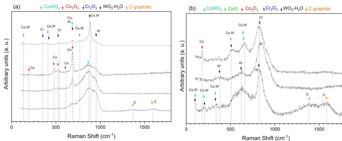
Fig. 9 Raman spectra of (a) SW (Stellite6–WC–Ni) and (b) SCW (Stellite6–WC–Ni–Cr<sub>3</sub>C<sub>2</sub>) coatings tested at 300 °C.
