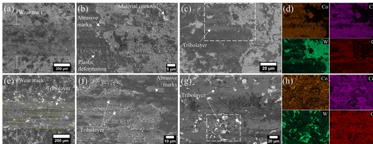
Fig. 8 Top view of the wear track of (a)–(c) Stellite6–WC–Ni coating and (e)–(g) Stellite6–Cr<sub>3</sub>C<sub>2</sub>–WC–Ni coating tested at 300 °C sliding for 20 000 cycles. EDS-mapping of (d) SW and (h) SCW coatings.
