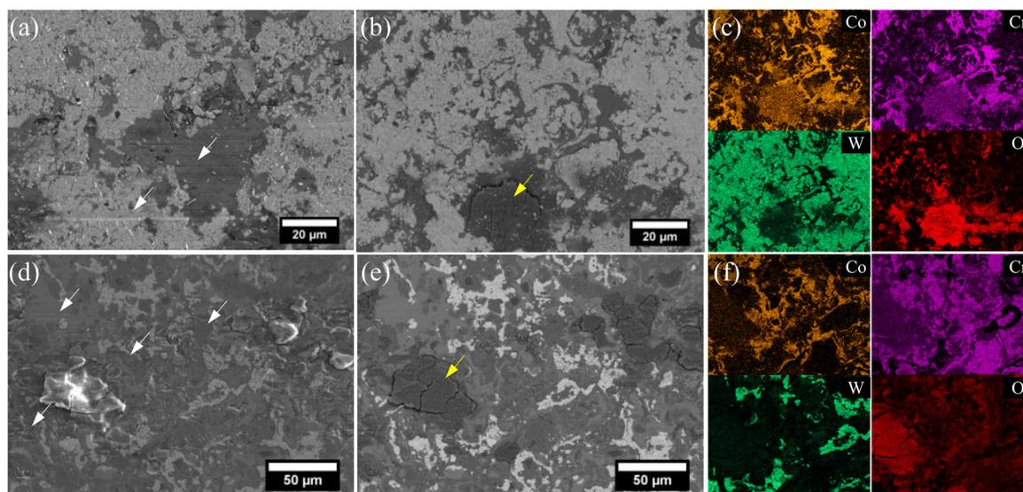
Fig. 7 Top view of the wear track of (a)–(c) Stellite6–WC–Ni coating and (d) and (e) Stellite6–Cr<sub>3</sub>C<sub>2</sub>–WC–Ni coating tested at RT for 5000 cycles. White arrows highlight the abrasive marks and yellow arrows the formation of tribolayers. EDS-mapping of (c) SW and (f) SWC coatings.
