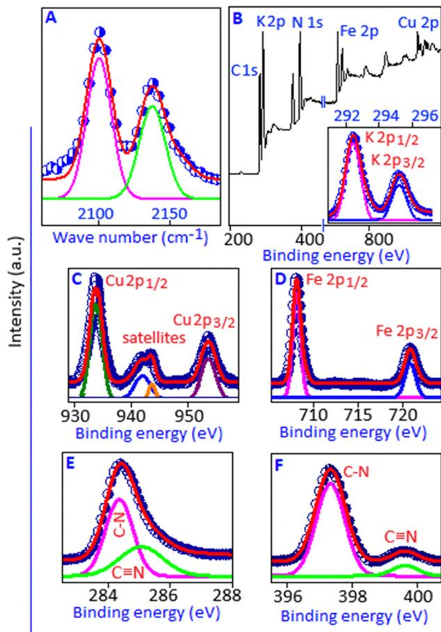
Fig. 4 (A) Raman spectrum of the cyano group, in the range of 1800–2400  $\text{cm}^{-1}$ , with the peak positions at 2095 and 2140  $\text{cm}^{-1}$ . (B) XPS survey spectrum of potassium copper ferrocyanide confirming the presence of K, Cu, Fe, C, and N. Inset: high-resolution K 2p spectrum. (C)–(F) High-resolution XPS spectrum of Cu 2p, Fe 2p, C 1s and N 1s.
