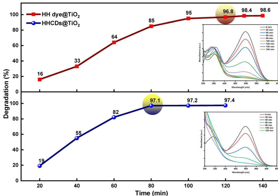
Fig. 15 Time evolution of CR degradation using HH dye@TiO<sub>2</sub> and HHCDs@TiO<sub>2</sub> under visible light irradiation, showing 96.8% degradation at 120 min for HH dye@TiO<sub>2</sub> and 97.1% degradation at 80 min for HHCDs@TiO<sub>2</sub>. The insets display the corresponding UV-vis spectral changes documenting the photocatalytic process.
