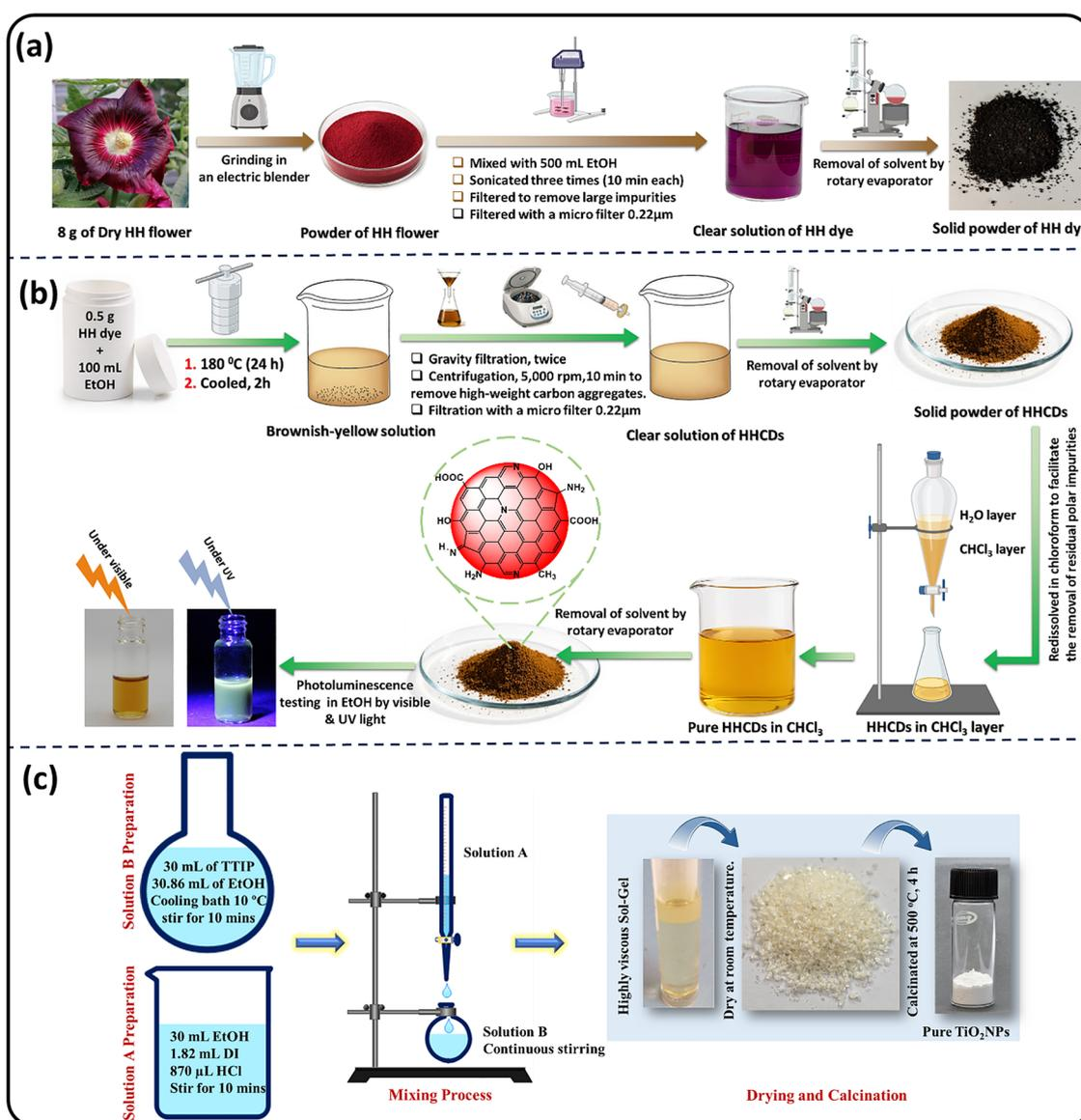
**Scheme 1** (a) The stepwise extraction process of the HH dye, (b) the hydrothermal synthesis procedure of the HHCDs from the HH dye, and (c) the sol-gel synthesis process of pure TiO<sub>2</sub> nanoparticles, including hydrolysis, condensation, gelation, drying, and calcination steps.
