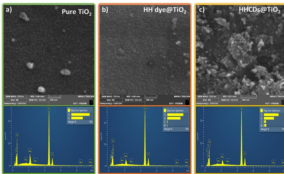
Fig. 8 FE-SEM images and corresponding EDX spectra of (a) pure  $\text{TiO}_2$  nanoparticles, (b) HH dye@ $\text{TiO}_2$ , and (c) HHCDs@ $\text{TiO}_2$  nanocomposites, showing morphological changes and elemental composition variations.
