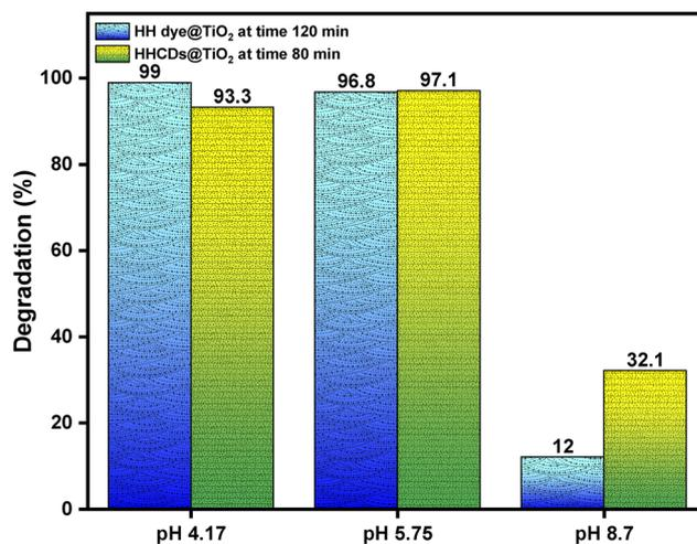
Fig. 16 pH-dependent photocatalytic degradation of the CR dye using HH dye@TiO<sub>2</sub> and HHCDs@TiO<sub>2</sub> under visible light irradiation (initial dye concentration: 10 ppm; optimal catalyst dosage; irradiation times: 120 min for HH dye@TiO<sub>2</sub> and 80 min for HHCDs@TiO<sub>2</sub>, respectively).
