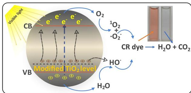
Fig. 18 Proposed mechanistic pathways for CR degradation by modified TiO<sub>2</sub> nanocomposites.
