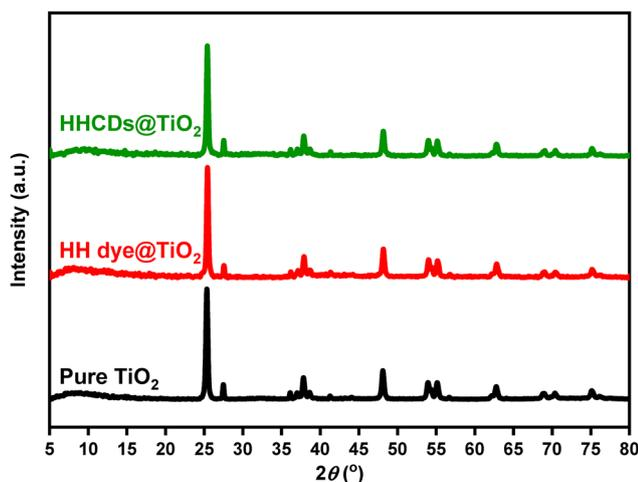
Fig. 7 XRD patterns comparing unmodified TiO<sub>2</sub> nanoparticles with HH dye@TiO<sub>2</sub> and HHCDs@TiO<sub>2</sub> nanocomposites, demonstrating the intact crystalline structure after surface modification.
