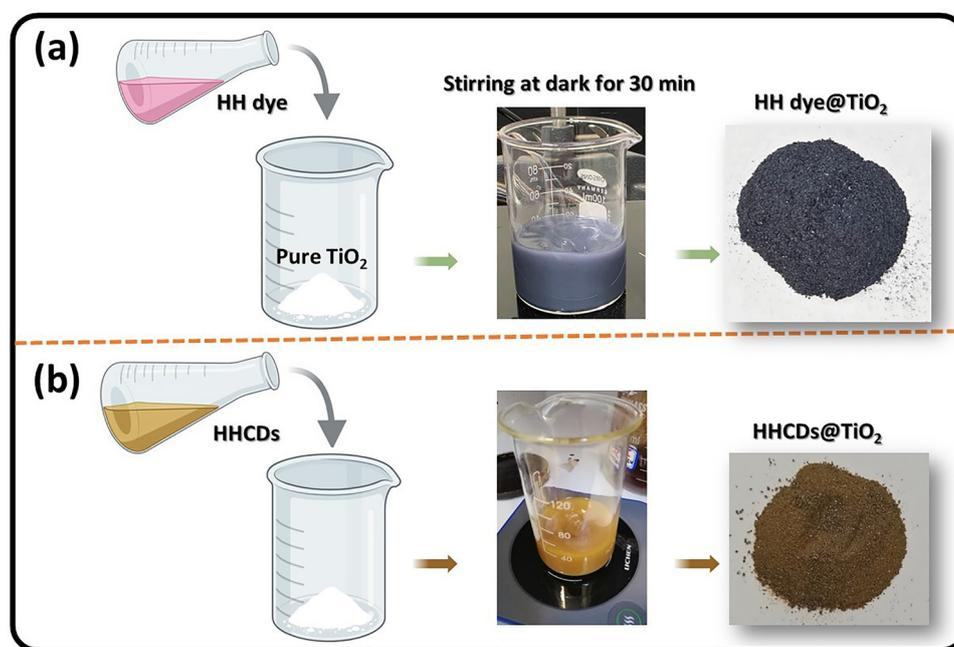
Scheme 2 Illustration of the fabrication process and the photographs of the resulting (a) HH dye@TiO<sub>2</sub> and (b) HHCDs@TiO<sub>2</sub> nanocomposites.
