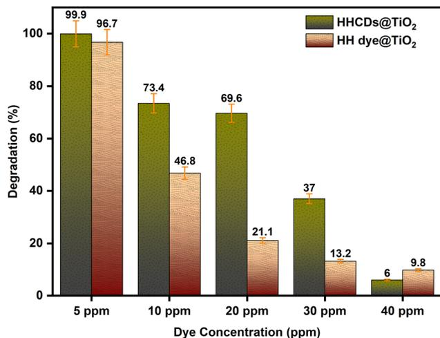
Fig. 13 Photodegradation efficiency of HH dye@TiO<sub>2</sub> and HHCDs@TiO<sub>2</sub> as a function of initial CR concentration under visible-light irradiation (60 min, unadjusted pH, optimum catalyst dosages).
