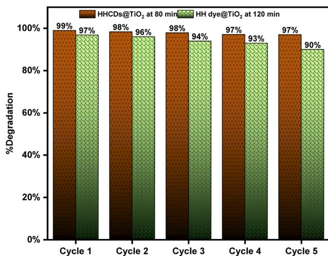
Fig. 17 Cyclic stability test of the HH dye@TiO<sub>2</sub> and HHCDs@TiO<sub>2</sub> photocatalysts for CR degradation over five consecutive uses under visible light irradiation.
