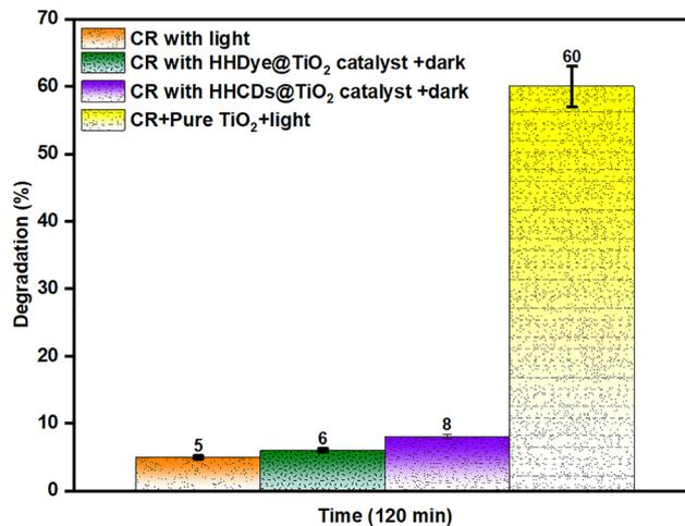
Fig. 14 Comparative analysis of CR (10 ppm) degradation efficiency after 120 minutes under four experimental conditions: visible light only, HH dye@TiO<sub>2</sub> in darkness, HHCDs@TiO<sub>2</sub> in darkness, and pure TiO<sub>2</sub> under visible light at unadjusted pH.
