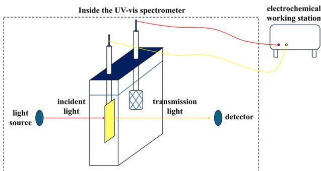
Fig. 9 Scheme of *in situ* transmittance testing system.
