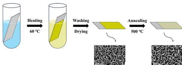
Fig. 1 Scheme of preparation route for the  $\text{WO}_3$  films.
