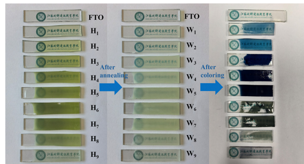
Fig. 11 Optical images of as-prepared H_2WO_4 /FTO, WO_3 /FTO samples and WO_3 /FTO samples after coloring.
