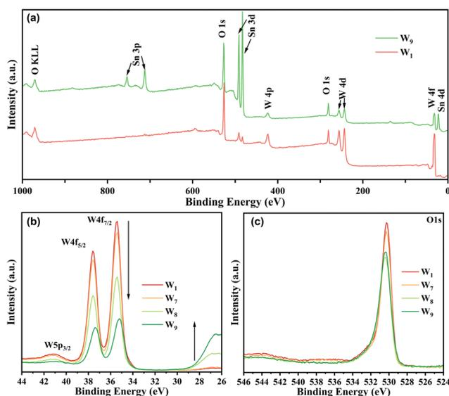
Fig. 6 (a) Survey scan XPS spectra of  $W_1$  and  $W_9$ , and the high-resolution XPS spectra for (b) W 4f and (c) O 1s of  $W_1$ ,  $W_7$ ,  $W_8$  and  $W_9$ .
