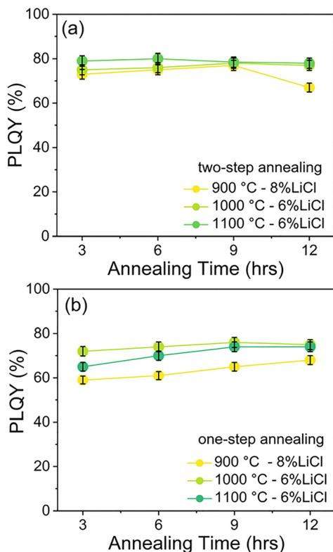
Fig. 4 Dependence of PLQY (under the 940 nm excitation) of 1540 nm emission in  $\text{YPO}_4:\text{Yb}^{3+}/\text{Er}^{3+}$  synthesized at different annealing times as a function of (a) two-step, (b) one-step synthesis using LiCl flux.
