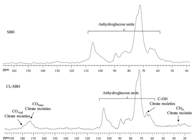
Fig. 4 Solid-state CP/MAS <sup>13</sup>C NMR spectra of the sweet basil seed hydrogel (SBH) before and after crosslinking (CL-SBH-3).
