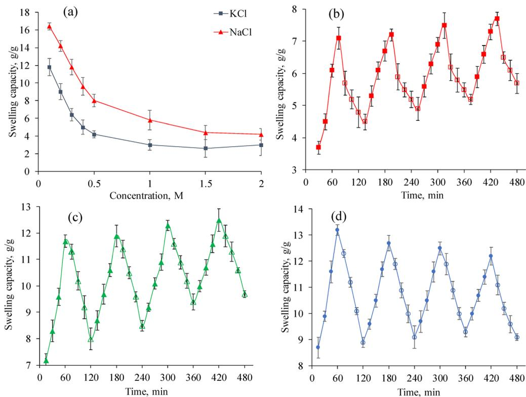
Fig. 7 Equilibrium swelling of the CL-SBH with varying NaCl and KCl concentrations (a); swelling-deswelling cycles at pH levels of 7.4 and 1.2 (b); in DW and normal saline (c); and in DW and ethanol (d).
