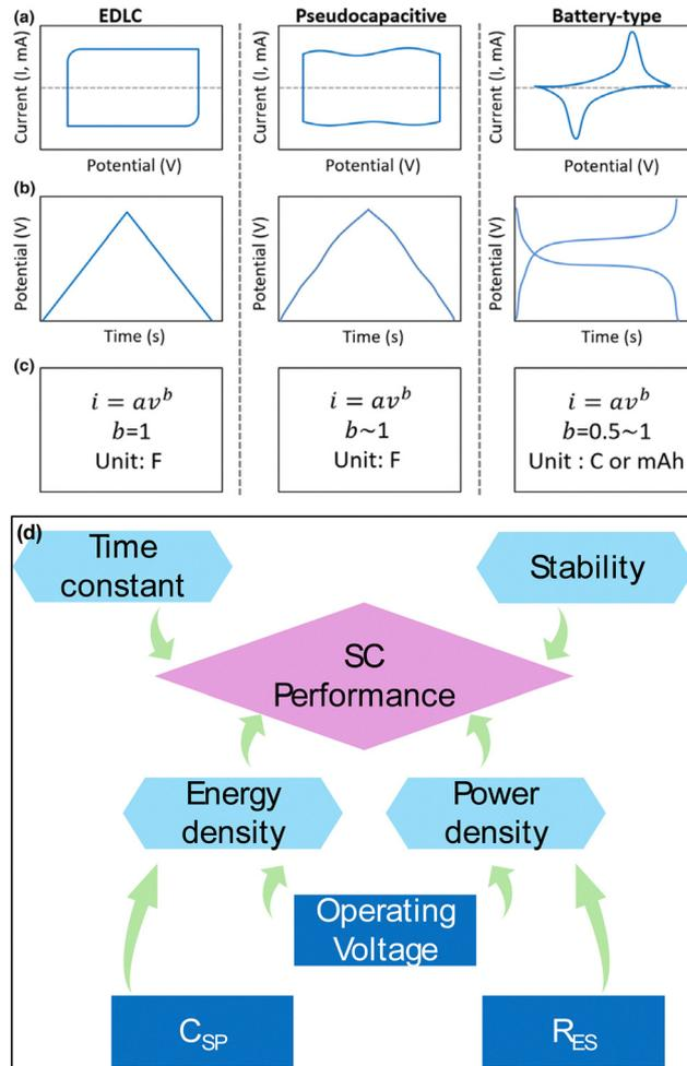
Fig. 1 (a)–(c) Categories of supercapacitors based on their energy storage mechanism. Reproduced with permission.<sup>37</sup> (d) Representation of key parameters affecting SC performance.
