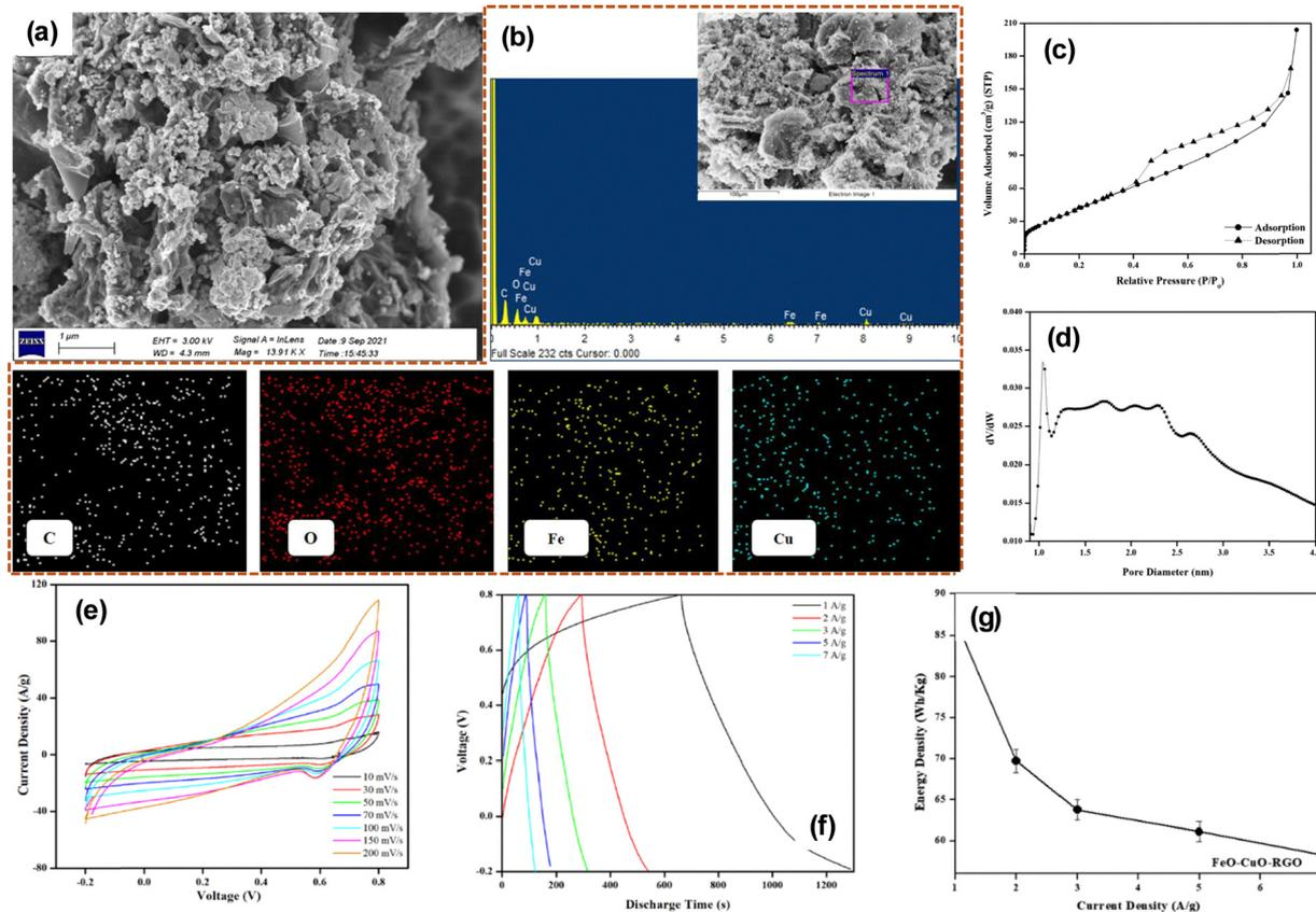
Fig. 8 (a) SEM image and (b) EDS of FeO-CuO-RGO. (c) N<sub>2</sub> adsorption/desorption curve and (d) average pore diameter circulation (e) CV curves (f) GCD curves (g) specific capacitance vs. current density plot of FeO-CuO-RGO. Reproduced with permission.<sup>173</sup>
