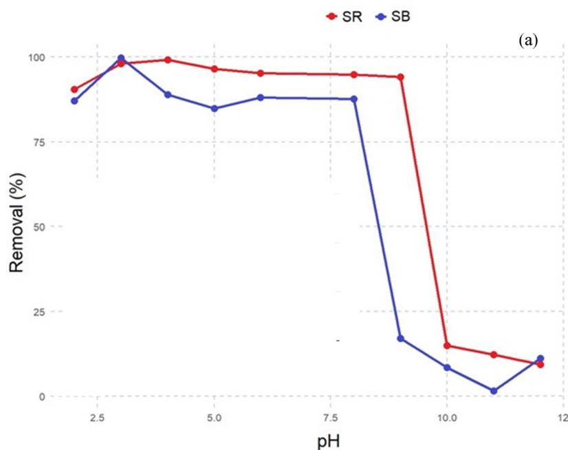
Fig. 3 (a) Effect of pH on the removal efficiency of the two treated dyes at a concentration of 75 mg L<sup>-1</sup> by 0.05 g of SE-CP and (b) point of zero charge (PZC) of the SE-CP biomaterial.
