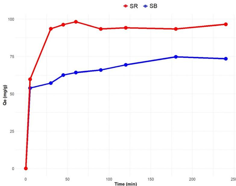
Fig. 5 Effect of the contact time on biosorption performance of the SE-CP biomaterial at a concentration of  $75 \text{ mg L}^{-1}$  and  $\text{pH} = 4$  for SR and  $\text{pH} = 3$  for SB at room temperature.
