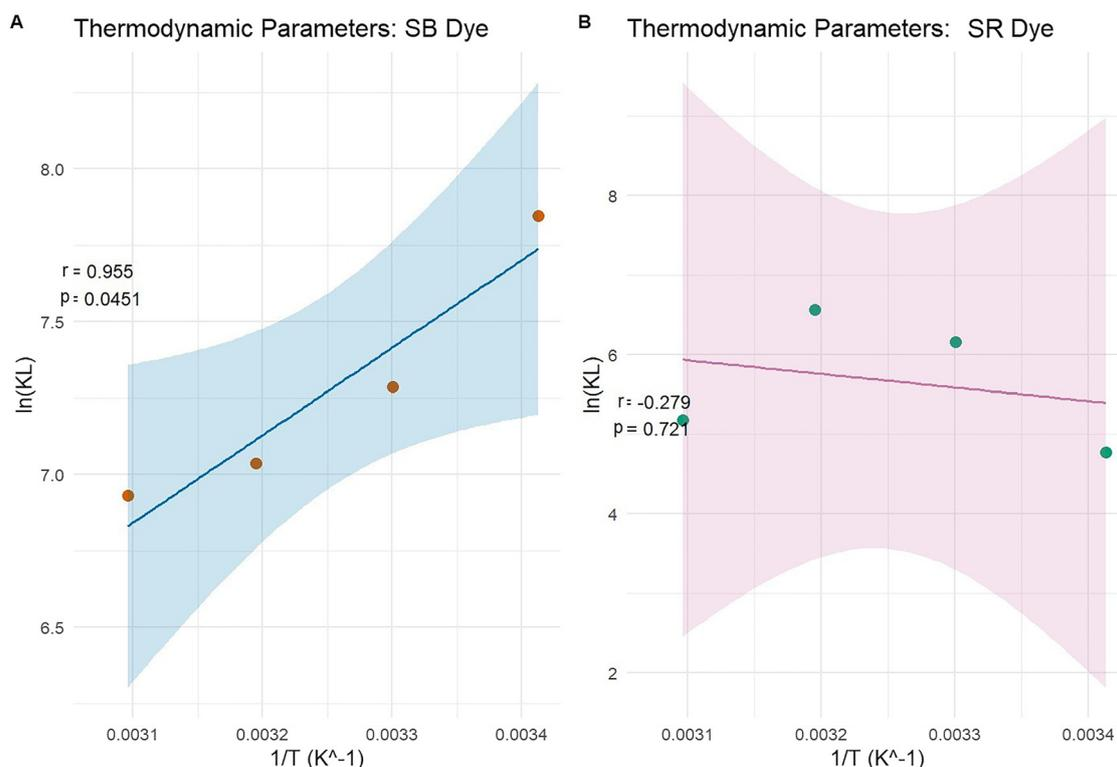
**Fig. 8** Adsorption data modeling using the Van't Hoff equation for the two studied dyes.
