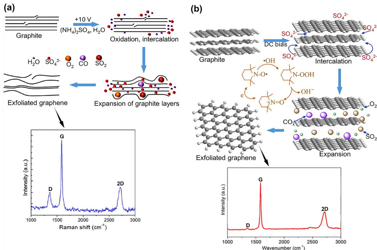
**Fig. 1** Schematic illustrations of graphite electrochemical exfoliation mechanisms: (a) standard electrochemical exfoliation. Reproduced with permission from ref. 20, Copyright 2014, American Chemical Society. (b) Radical-assisted electrochemical exfoliation reproduced with permission from ref. 7, Copyright 201, American Chemical Society.
