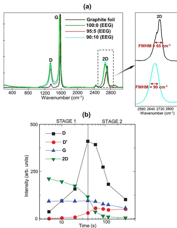
Fig. 6 (a) Average Raman spectra of EEG samples prepared with various concentrated  $\text{H}_2\text{SO}_4\text{:H}_3\text{PO}_4$  intercalant blends for an 800 s intercalation, compared with the spectrum of the pristine graphite. Reproduced with permission from ref. 46, Copyright 2025, Elsevier B.V. (b) Evolution of the D, D', G, and 2D band intensities with increasing defect concentration in graphene. Reproduced with permission from ref. 15, Copyright 2013, American Physical Society.
