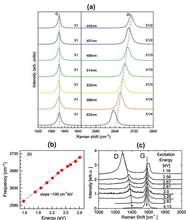
**Fig. 3** (a) Raman spectra of monolayer graphene (1LG) measured at multiple excitation energies, and (b) dispersion of the 2D peak position as a function of excitation energy. Reproduced with permission from ref. 29, Copyright 2018, The Royal Society of Chemistry. (c) Raman spectra of graphite recorded using various laser excitations. Reproduced with permission from ref. 34, Copyright 1998, Elsevier Science B.V.
