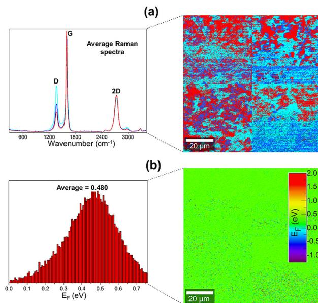
Fig. 7 Large-area Raman mapping of EEG samples: (a) true-component Raman intensity distribution images with corresponding average Raman spectra for samples prepared using different  $\text{H}_2\text{SO}_4:\text{H}_3\text{PO}_4$  intercalation blends during 800 s intercalation; (b) spatial maps showing the corresponding Fermi-level shifts. Reproduced with permission from ref. 46, Copyright 2025, Elsevier B.V.
