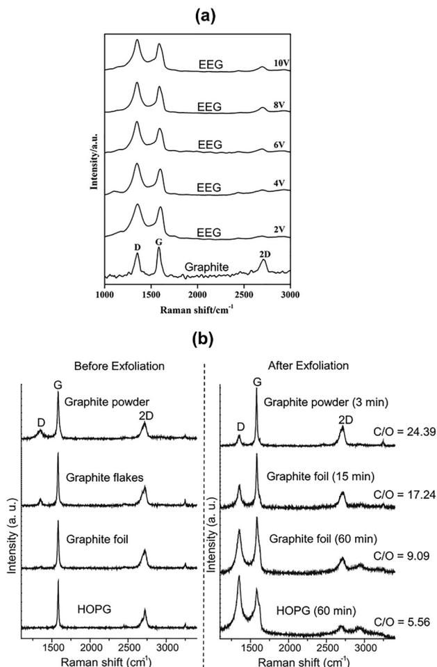
Fig. 2 (a) Raman spectra of graphite and graphene prepared at different potentials. Reproduced with permission from ref. 22, Copyright 2015, The Royal Society of Chemistry. (b) Raman spectra of EEG exfoliated from graphite powder (3 min), graphite foil (15 and 60 min), and HOPG (60 min), compared to their respective unexfoliated materials. Reproduced with permission from ref. 24, Copyright 2015, Elsevier Ltd.
