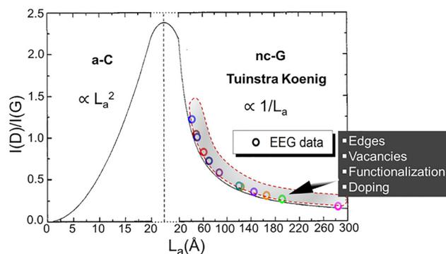
**Fig. 4** Variation of the  $I(\text{D})/I(\text{G})$  intensity ratio as a function of in-plane crystallite size ( $L_a$ ). Reproduced with permission from ref. 36. Copyright 2000, The American Physical Society. The shaded region over the EEG data points indicates defect-related contributions. The EEG data points were extracted from Raman spectra provided in Table S1, as reported by various research groups.
