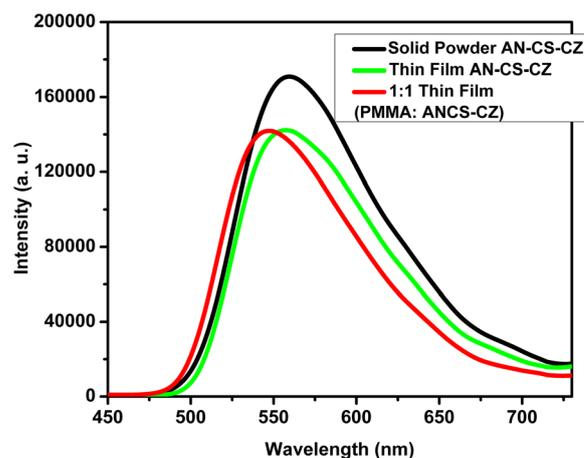
Fig. 7 Fluorescence spectra of **AN-CS-CZ**: powdered sample (black), drop-cast thin film (green), and 1:1 PMMA-compound film (red). All spectra were recorded with identical excitation and instrument settings.
