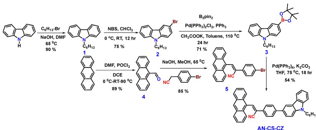
Scheme 1 Synthetic scheme for the target compound **AN-CS-CZ**.
