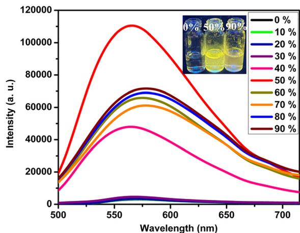
Fig. 3 Emission spectra of AN-CS-CZ in ACN/water mixtures with different  $f_w$  (Con.  $3 \times 10^{-5}$  M;  $\lambda_{ex} = 385$  nm). The inset contains digital photos taken under a UV 365 nm lamp.
