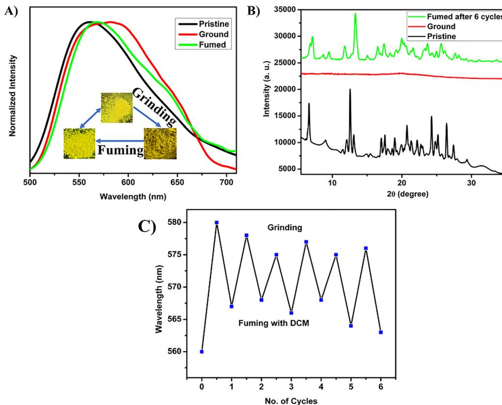
Fig. 5 (A) Normalized emission spectra of **AN-CS-CS** in the pristine state, after mechanical grinding, and following solvent fuming. The inset displays the corresponding photographs under 365 nm UV illumination. (B) Powder X-ray diffraction (PXRD) patterns of **AN-CS-CS** in different states and (C) reversibility plot of **AN-CZ-CS** after undergoing MFC for > 5 cycles.
