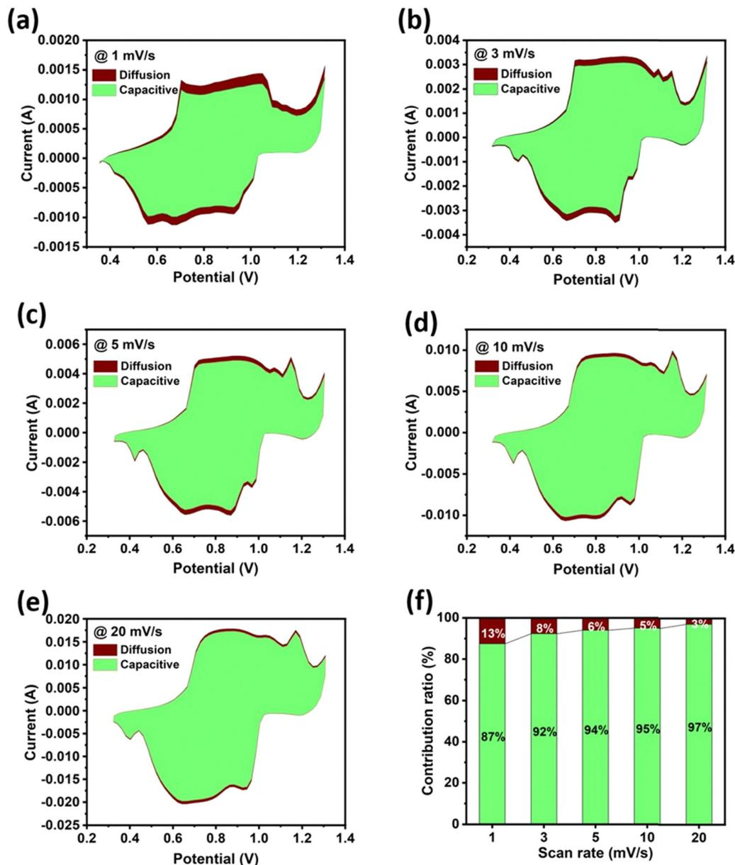
Fig. 10 Examination of charge storage characteristics using CV analysis (Dunn's approach): (a)  $1 \text{ mV s}^{-1}$ , (b)  $3 \text{ mV s}^{-1}$ , (c)  $5 \text{ mV s}^{-1}$ , (d)  $10 \text{ mV s}^{-1}$ , (e)  $20 \text{ mV s}^{-1}$ , and (f) percentage comparison of capacitive and diffusion-controlled contributions under different scan rates.
