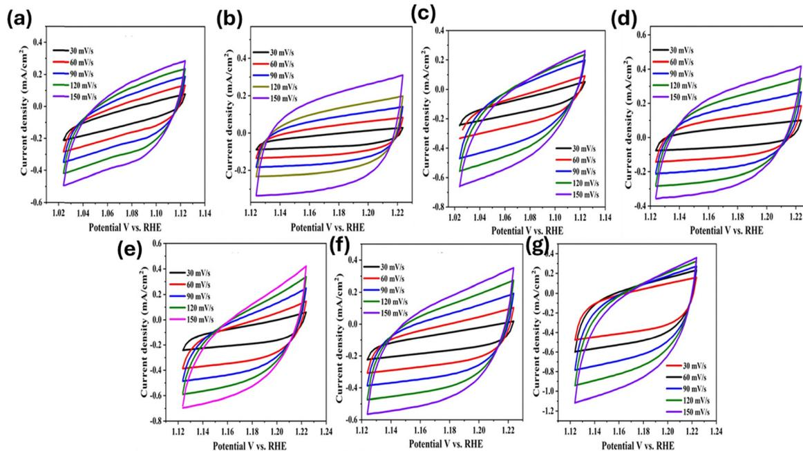
Fig. 6 (a)–(g) CV analysis of the electrodes: K1 as CNT–Ni, K2 as CNT–Cu, K3 as CNT–Ag, K4 as CNT–Ni–Cu, K5 as CNT–Ni–Ag, K6 as CNT–Cu–Ag and K7 as CNT–Ni–Cu–Ag, at different scan rates.
