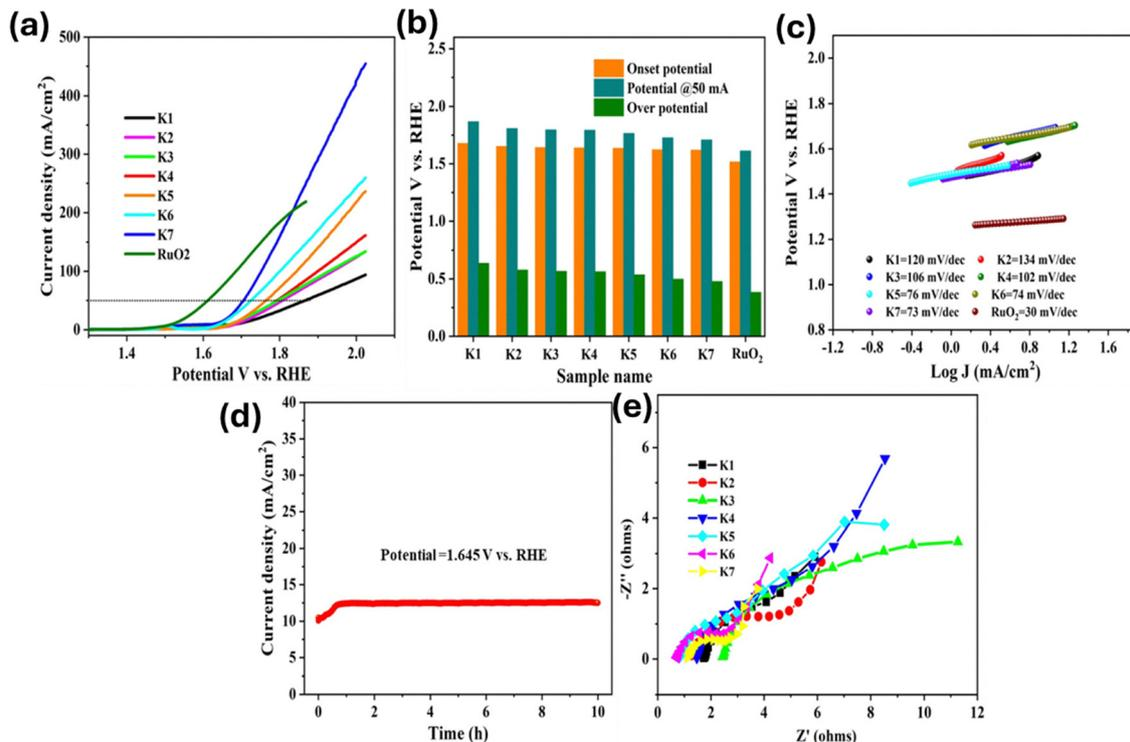
Fig. 5 OER analysis using 1 M KOH: (a) polarization curves of K1–K7 and RuO<sub>2</sub>. (b) Comparison of onset potential, the potential required to reach 50 mA cm<sup>-2</sup> current density, and overpotential for K1–K7 and RuO<sub>2</sub>. (c) Corresponding Tafel slopes. (d) Chronoamperometry analysis of K7, and (e) EIS analysis of K1–K7 NPs.
