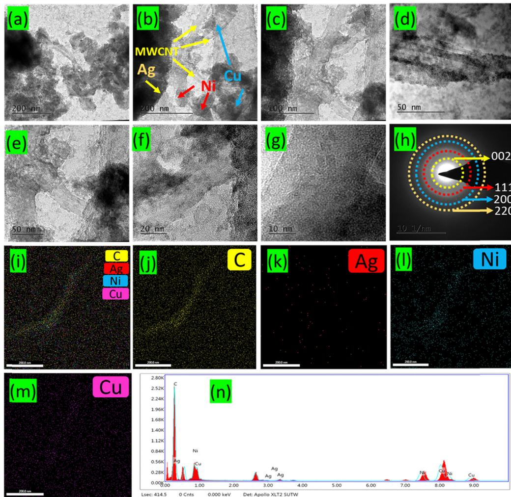
Fig. 3 (a)–(g) HR-TEM images of CNT–Ni–Cu–Ag with different magnifications, (h) the corresponding SAED pattern, (i)–(m) the corresponding elemental mapping images and (n) EDS spectrum of the CNT–Ni–Cu–Ag nanocomposites.
