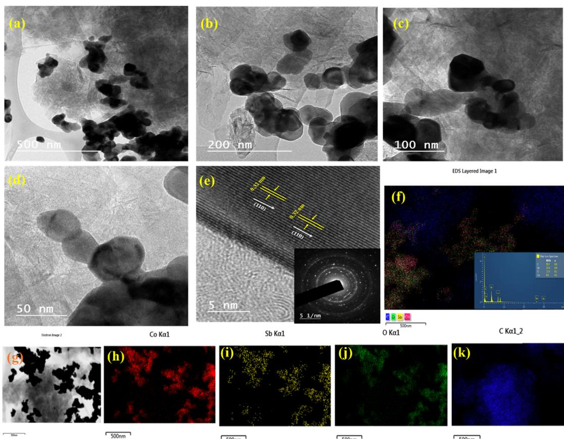
Fig. 5 HR-TEM micrographs of  $\text{CoSb}_2\text{O}_6/\text{rGO}_{15}$  at different magnifications: (a) 500 nm, (b) 200 nm, (c) 100 nm, (d) 50 nm, and (e) 5 nm; inset: SAED pattern of  $\text{CoSb}_2\text{O}_6/\text{rGO}_{15}$ . (f) Layered EDS image at a scale of 500 nm for  $\text{CoSb}_2\text{O}_6/\text{rGO}_{15}$ . (g) Electronic image of  $\text{CoSb}_2\text{O}_6/\text{rGO}_{15}$  showing the presence of (h) cobalt, (i) antimony, (j) oxygen, and (k) carbon.
