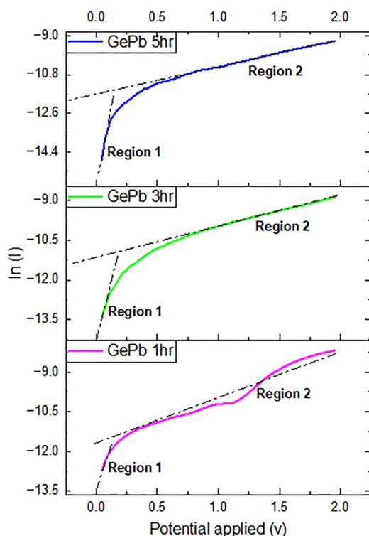
Fig. 10 Plot of  $\ln(I)$  against the applied potential  $V$  for the GePb based p-i-n junctions annealed for 1 h, 3 h, and 5 h.
