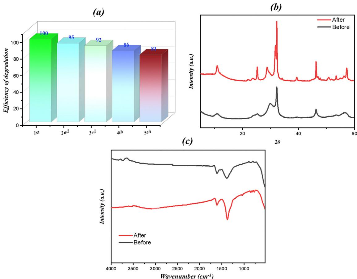
Fig. 13 (a) Photocatalytic reusability of the  $x = 0.7$  composite for RhB degradation over five consecutive cycles; (b) XRD patterns and (c) FTIR spectra of the  $x = 0.7$  composite before and after degradation cycles.
