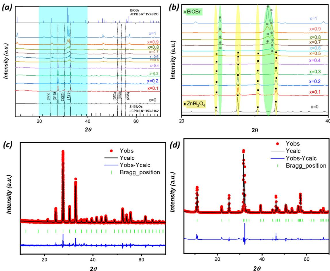
Fig. 2 (a) XRD patterns of the synthesized samples; (b) zoom out of the  $2\theta$  value from 20 to 40; (c) the Rietveld refinement results for the cubic  $\text{ZnBi}_2\text{O}_4$  phase and (d) the Rietveld refinement results for the tetragonal BiOBr phase.
