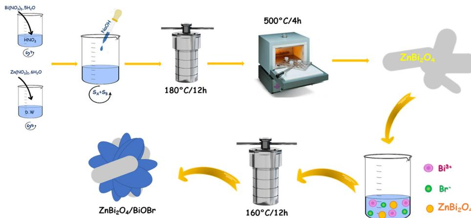
Fig. 1 Synthesis process of the  $\text{ZnBi}_2\text{O}_4/\text{BiOBr}$  composite.
