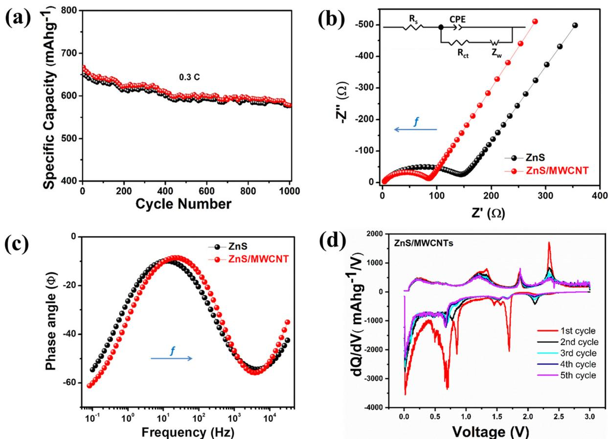
Fig. 5 (a) Long-term cycling stability of ZnS/MWCNTs for 500 cycles at 0.3C. (b) Electrochemical impedance spectra (Nyquist plot) of the pristine ZnS and ZnS/MWCNT heterostructure. (c) Bode angle plot vs frequency of the pristine ZnS and ZnS/MWCNT heterostructure electrodes. (d) (dQ/dV) plot of the ZnS/MWCNT heterostructure electrode.
