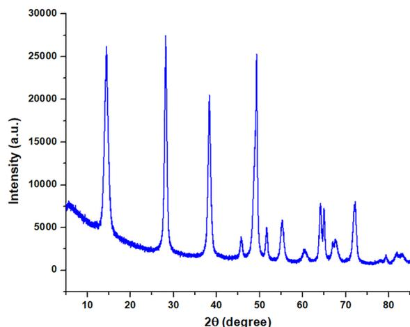
Fig. 4 X-ray diffraction analysis of the synthesized Ni- $\gamma\text{Al}_2\text{O}_3$  nanocatalyst.
