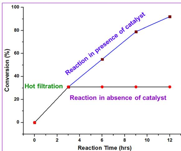
Fig. 11 Hot-filtration test of Ni- $\gamma$ -Al<sub>2</sub>O<sub>3</sub> catalyst using **1a** (1 mmol), K<sub>4</sub>[Fe(CN)<sub>6</sub>] $\cdot$ 3H<sub>2</sub>O (0.2 mmol), K<sub>2</sub>CO<sub>3</sub> (1.2 mmol), Ni- $\gamma$ -Al<sub>2</sub>O<sub>3</sub> (6 mol%), DMF (3 mL) at 120 °C under ambient conditions.
