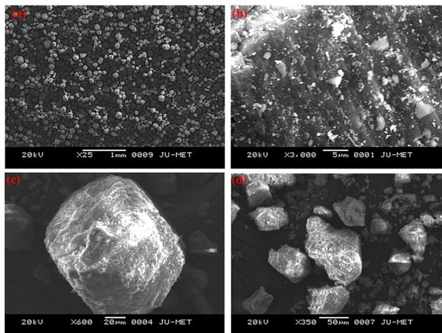
Fig. 6 Scanning electron microscopy (SEM) images (a)–(d) of synthesized Ni- $\gamma$ Al<sub>2</sub>O<sub>3</sub> nanocatalysts.
