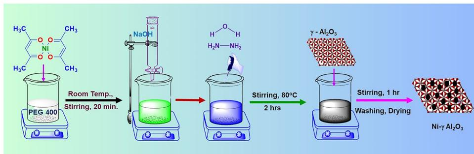
Fig. 2 Schematic representation for the synthesis of Ni- $\gamma$ -Al<sub>2</sub>O<sub>3</sub> nanocatalyst.
