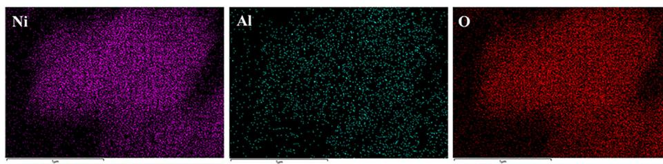
Fig. 8 Elemental mapping images of the synthesized Ni- $\gamma$ Al<sub>2</sub>O<sub>3</sub> nanocatalyst.
