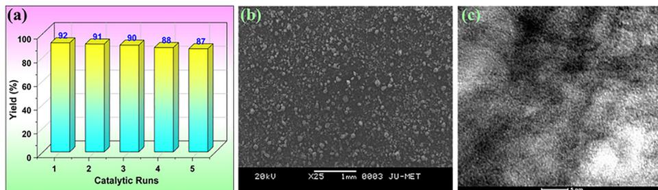
Fig. 10 (a) Recycling test of Ni- $\gamma$ -Al<sub>2</sub>O<sub>3</sub> catalyst, (b) SEM image of Ni- $\gamma$ -Al<sub>2</sub>O<sub>3</sub> (after recycled 5 times), and (c) TEM image of Ni- $\gamma$ -Al<sub>2</sub>O<sub>3</sub> (after recycled 5 times).
