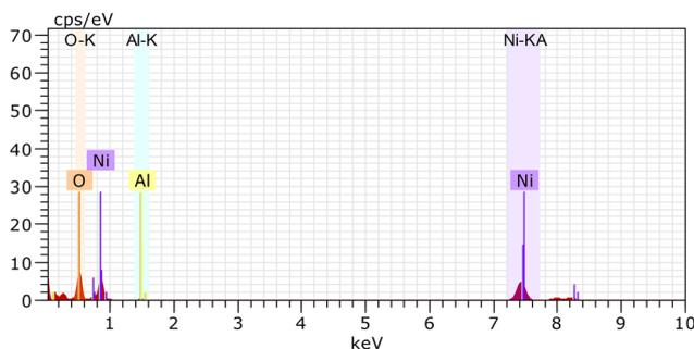
Fig. 7 Energy dispersive X-ray spectroscopy analysis of Ni- $\gamma$ Al<sub>2</sub>O<sub>3</sub> nanocatalyst.
