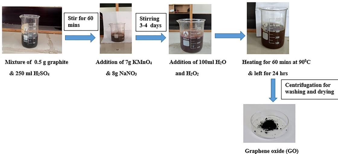
Scheme 2 Synthetic route for graphene oxide (GO).
