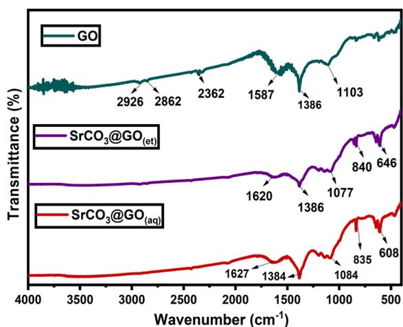
Fig. 3 FTIR spectra of GO, SrCO<sub>3</sub>@GO<sub>(aq)</sub> and SrCO<sub>3</sub>@GO<sub>(et)</sub>.
