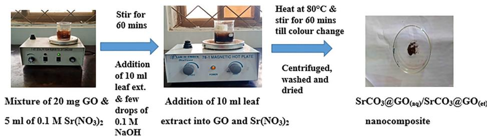
Scheme 3 *M. oleifera*-mediated bio-synthesis of SrCO<sub>3</sub>@GO<sub>(aq)</sub> and SrCO<sub>3</sub>@GO<sub>(et)</sub> nanocomposites.
