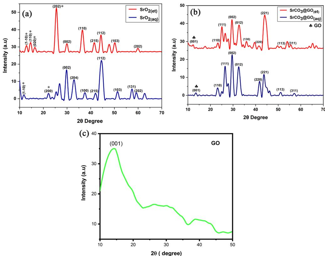
Fig. 1 (a) XRD patterns of  $\text{SrO}_2(\text{aq})$  and  $\text{SrO}_2(\text{et})$  NPs. (b) XRD patterns of  $\text{SrCO}_3@\text{GO}(\text{aq})$  and  $\text{SrCO}_3@\text{GO}(\text{et})$ . (c) XRD pattern of graphene oxide.
