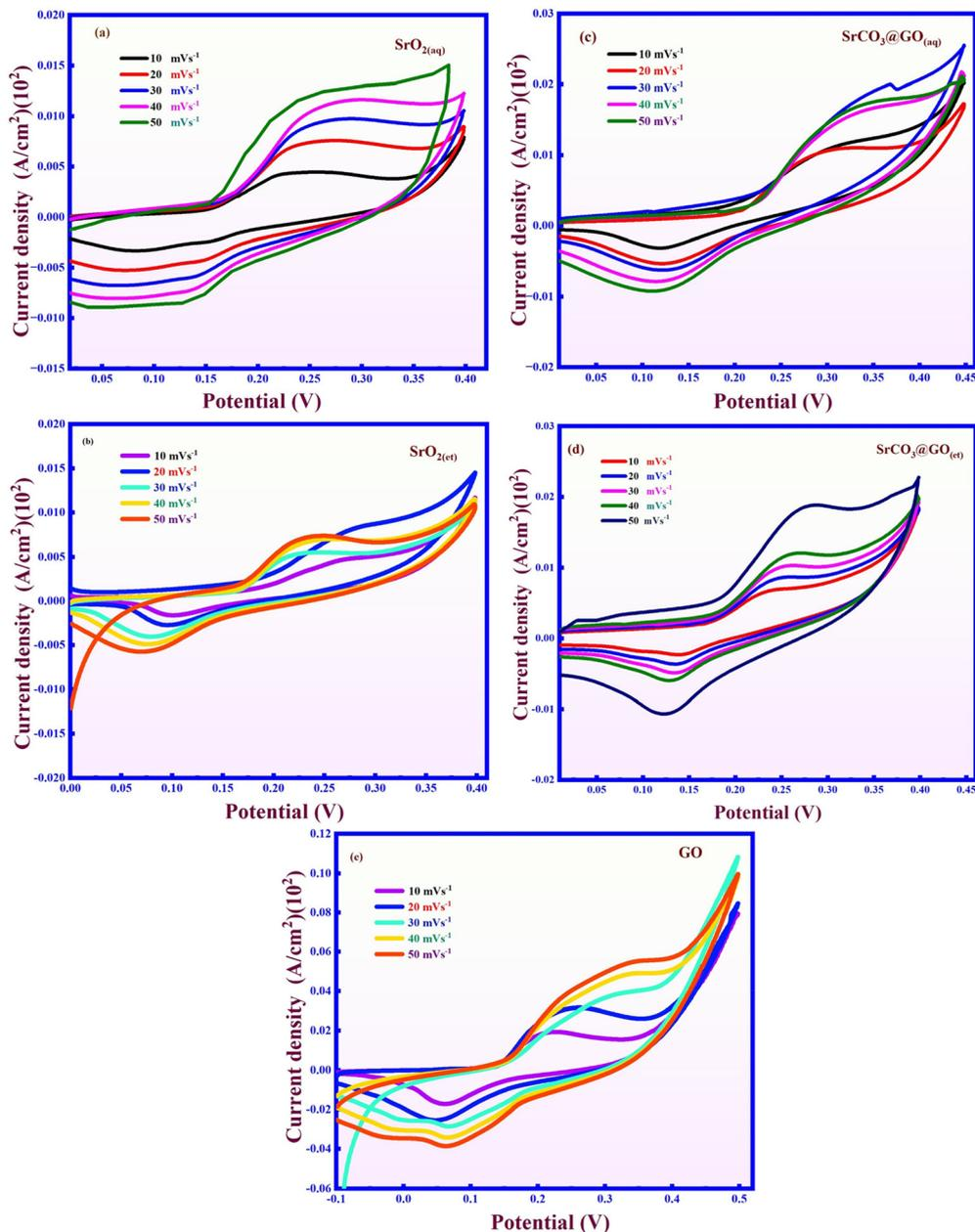
Fig. 10 Cyclic voltammograms spectra of (a)  $\text{SrO}_{2(\text{aq})}$ , (b)  $\text{SrO}_{2(\text{et})}$ , (c)  $\text{SrCO}_3@\text{GO}_{(\text{aq})}$ , (d)  $\text{SrCO}_3@\text{GO}_{(\text{et})}$ , and (e) GO.
