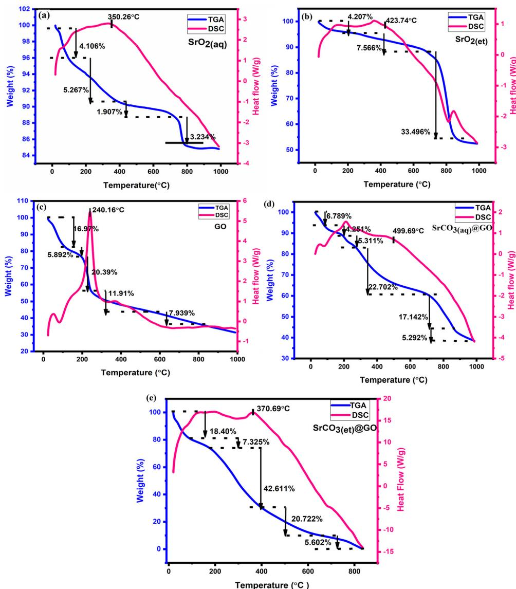
Fig. 9 (a) TGA/DSC curves of  $\text{SrO}_2(\text{aq})$ . (b) TGA/DSC curves of  $\text{SrO}_2(\text{et})$ . (c) TGA/DSC curves of GO. (d) TGA/DSC curves of  $\text{SrCO}_3@GO(\text{aq})$ . (e) TGA/DSC curves of  $\text{SrCO}_3@GO(\text{et})$ .
