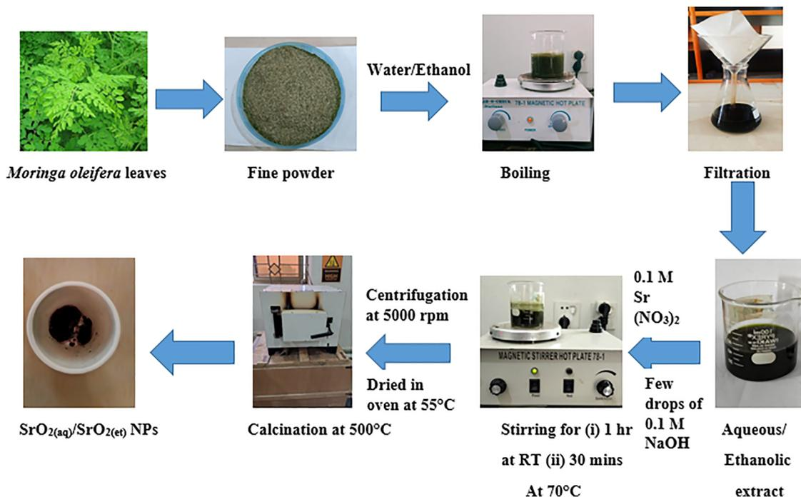
Scheme 1 *Moringa oleifera*-mediated biosynthesis of  $\text{SrO}_{2(\text{aq})}$  and  $\text{SrO}_{2(\text{et})}$  NPs.
