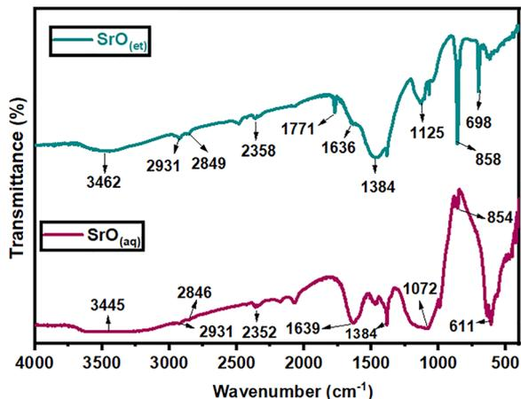
Fig. 2 FTIR spectra of *M. oleifera*-mediated SrO<sub>(aq)</sub> and SrO<sub>(et)</sub> NPs.
