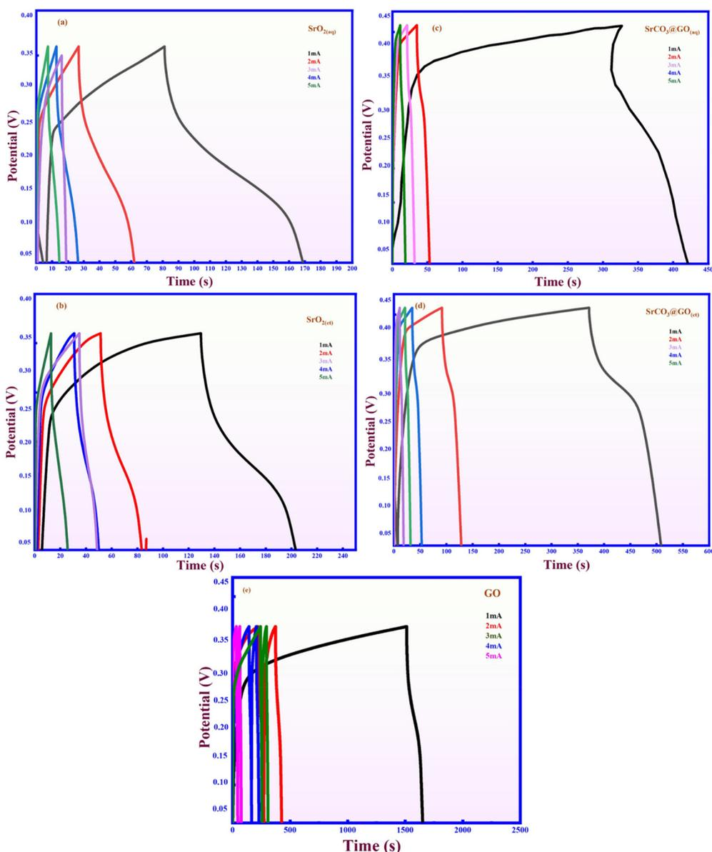
Fig. 11 Galvanostatic charging and discharging (GCD) behavior of (a)  $\text{SrO}_{2(\text{aq})}$ , (b)  $\text{SrO}_{2(\text{et})}$ , (c)  $\text{SrCO}_3@\text{GO}_{(\text{aq})}$ , (d)  $\text{SrCO}_3@\text{GO}_{(\text{et})}$ , and (e) GO.
