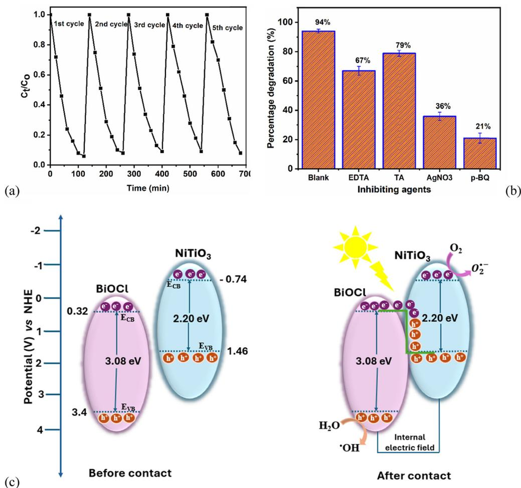
Fig. 4 (a) Reusability plot of the BiOCl/NiTiO<sub>3</sub> heterostructured photoanode for 5 mg L<sup>-1</sup> CPX degradation under PEC application, (b) scavenger studies of ROS in the PEC system on the BiOCl/NiTiO<sub>3</sub> heterostructured photoanode, and (c) Z-scheme behaviour of the BiOCl/NiTiO<sub>3</sub> heterostructured photoanode.
