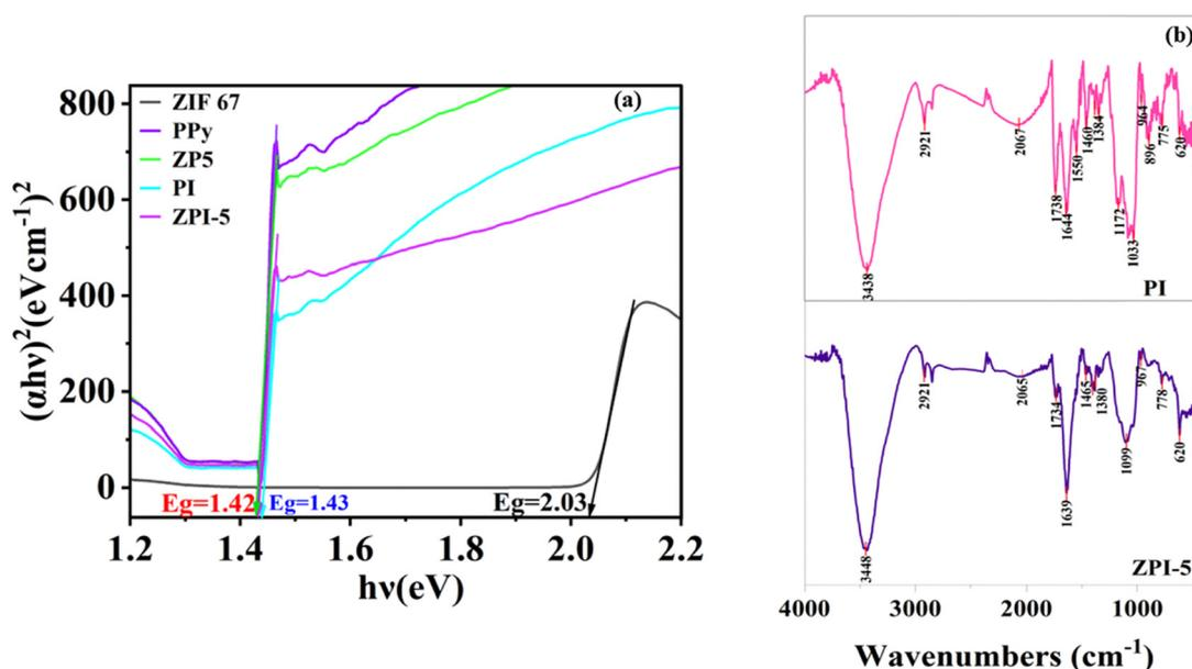
Fig. 17 (a) Tauc plot and optical bandgap of the composites and inks. (b) FTIR spectra of the PI and ZPI-5 ink composites.
