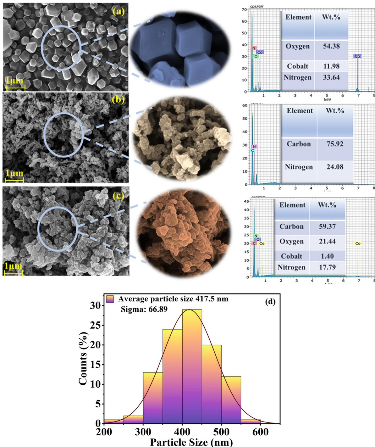
Fig. 6 SEM images of (a) ZIF-67, (b) PPy, and (c) the ZIF-67/PPy composite showing surface morphology, and (d) particle size distribution of ZIF-67.
