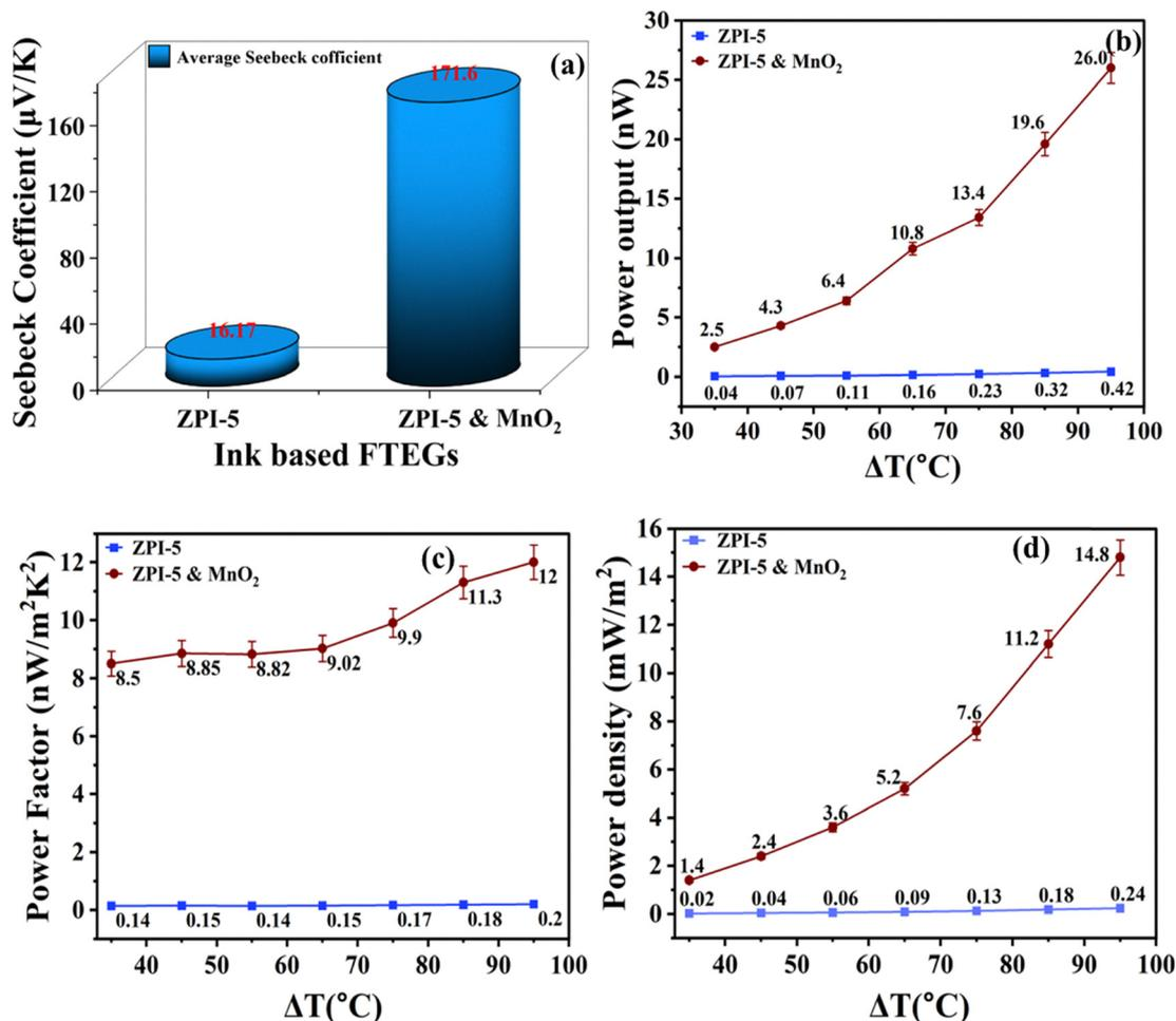
Fig. 18 Comparison of (a) Seebeck coefficient, (b) power output, (c) power factor, and (d) power density between ZPI-5 and ZPI-5 & MnO<sub>2</sub> FTEGs.
