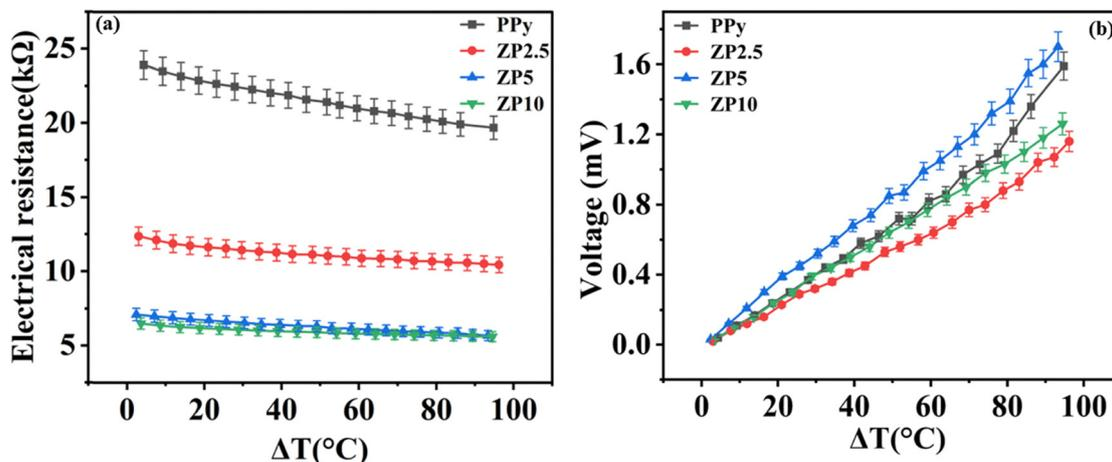
Fig. 12 (a) Resistivity vs.  $\Delta T$  and (b)  $\Delta V$  vs.  $\Delta T$  curves of ink-based FTEGs.
