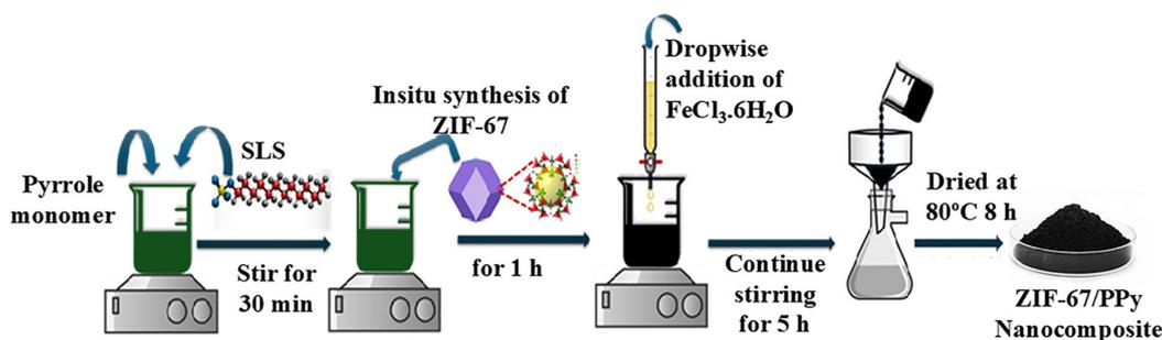
Fig. 2 Synthetic route of the ZIF-67/PPy composites showing *in situ* polymerization of pyrrole on ZIF-67 surfaces to form conductive hybrids.
