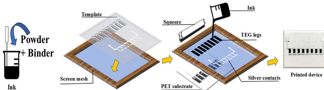
Fig. 3 Formulation process of the ZIF-67/PPy-based ink and fabrication steps for the flexible thermoelectric generator (FTEG) device.
