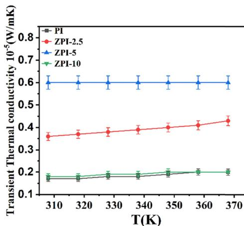
Fig. 11 Transient thermal conductivity of PPy and ZPI-based FTEGs.
