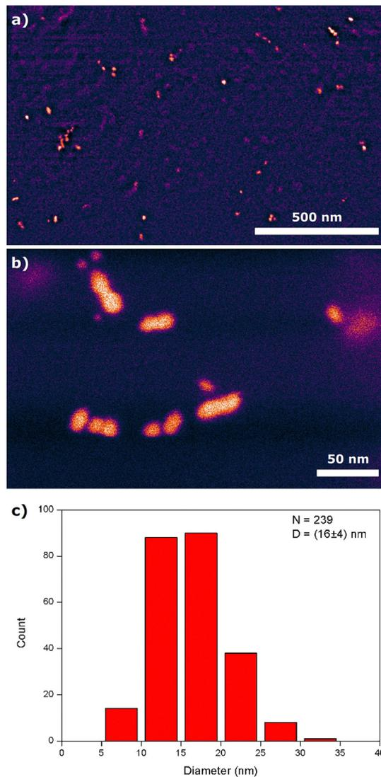
Fig. 3 High-resolution SEM images (backscattered signal, false colour) of sample S3: (a) magnification 100 000 $\times$ ; (b) magnification 500 000 $\times$ . (c) Size distribution of Au NPs in sample S3, based on high-resolution SEM images comprising 239 Au NPs in total.
