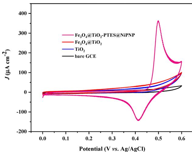
Fig. 14 Cyclic voltammograms of the bare GCE,  $\text{TiO}_2$  nanostructure/GCE,  $\text{Fe}_3\text{O}_4@ \text{TiO}_2$  core-shell/GCE, and  $\text{Fe}_3\text{O}_4@ \text{TiO}_2$ -PTES@NiPNP hybrid/GCE in 0.1 M NaOH at a scan rate of  $100 \text{ mV s}^{-1}$ .
