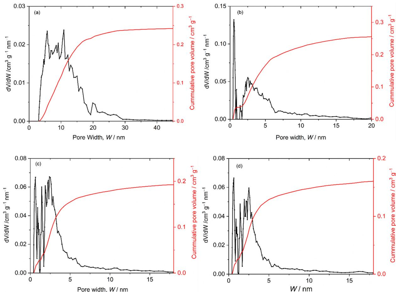
Fig. 11 Pore width distribution plots for (a)  $\text{Fe}_3\text{O}_4$ , (b)  $\text{Fe}_3\text{O}_4@\text{TiO}_2$ , (c)  $\text{Fe}_3\text{O}_4@\text{TiO}_2$ -CPTES nanostructures and (d) the immobilized nickel-PNP pincer complex obtained using a non-local density functional theory (NLDFT) kernel based on the adsorption models for argon on zeolites/silica at 87 K with cylindrical pores (see text for notation).
