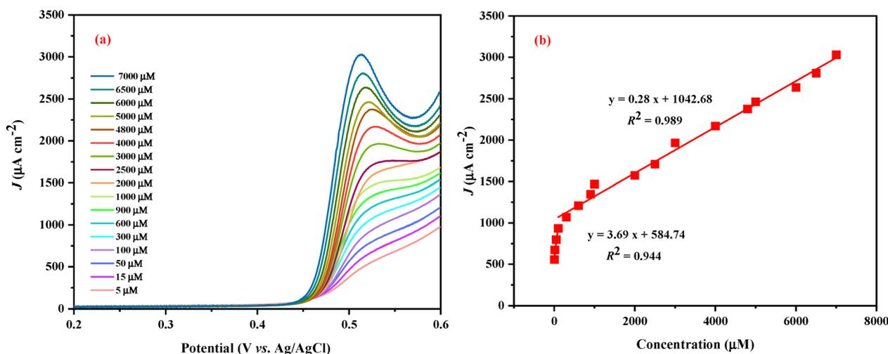
Fig. 17 (a) DPV diagrams of the  $\text{Fe}_3\text{O}_4@TiO_2\text{-PTES@NiPNP/GCE}$  with Nafion at different Fe glucose concentrations in 0.1 M NaOH; (b) its corresponding calibration curve (for 5–2500  $\mu\text{M}$ , the  $J$  values were acquired at +0.525 V).
