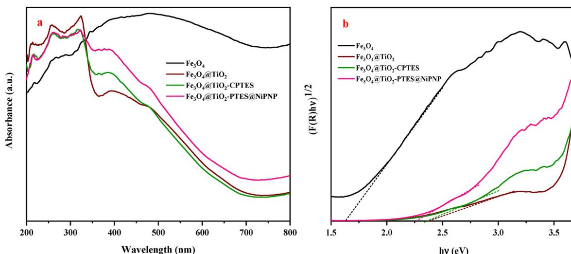
Fig. 3 (a) UV-vis DRS spectra and (b) Tauc plots of  $\text{Fe}_3\text{O}_4$ ,  $\text{Fe}_3\text{O}_4@\text{TiO}_2$ ,  $\text{Fe}_3\text{O}_4@\text{TiO}_2\text{-CPTES}$ , and  $\text{Fe}_3\text{O}_4@\text{TiO}_2\text{-PTES@NiPNP}$ .
