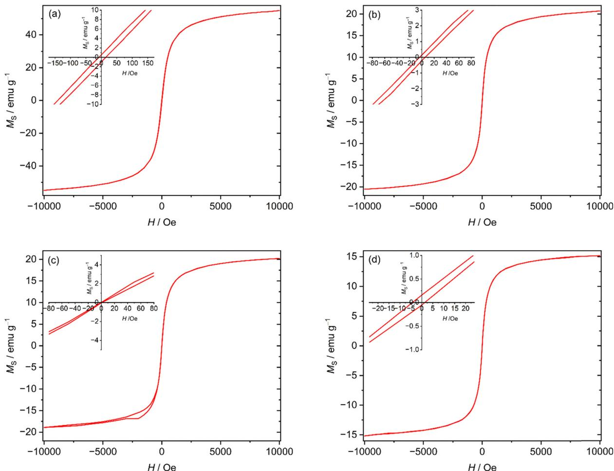
Fig. 12 Magnetization plots for the  $\text{Fe}_3\text{O}_4$ ,  $\text{Fe}_3\text{O}_4@TiO_2$ ,  $\text{Fe}_3\text{O}_4@TiO_2$ -CPTES nanostructures and the material with immobilized nickel-PNP pincer complex measured at room temperature (a)–(d), respectively. Insets: Zoomed-in view to display hysteresis loops.
