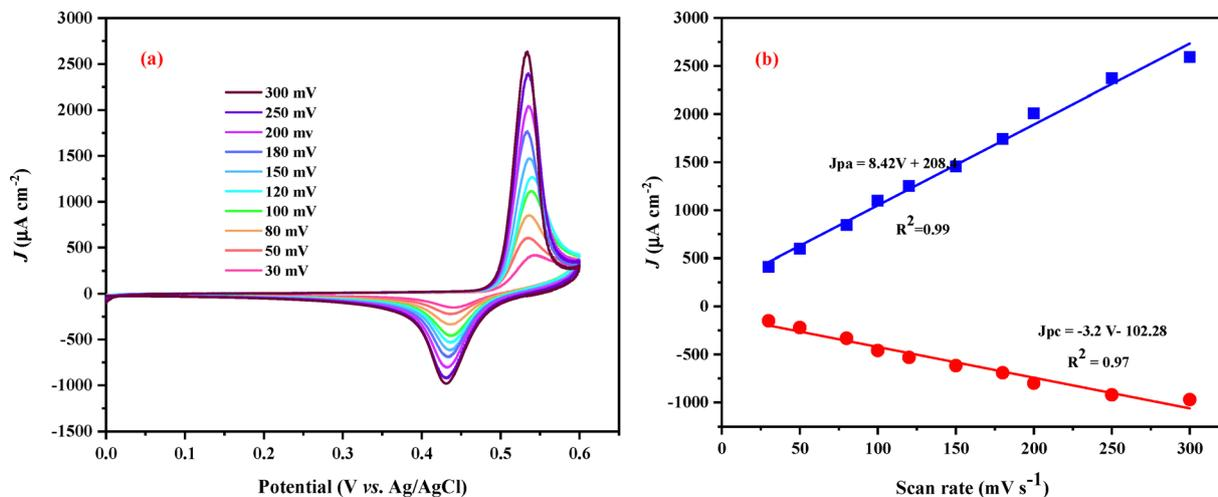
Fig. 16 (a) Cyclic voltammograms of the  $\text{Fe}_3\text{O}_4@TiO_2\text{-PTES@NiPNP/GCE}$  with Nafion in the presence of 0.1 mM glucose and 0.1 M NaOH at different scan rates of 30–300  $\text{mV s}^{-1}$ . (b) the linear plots of Ni(III)/Ni(II) redox peak current density vs. scan rates.
