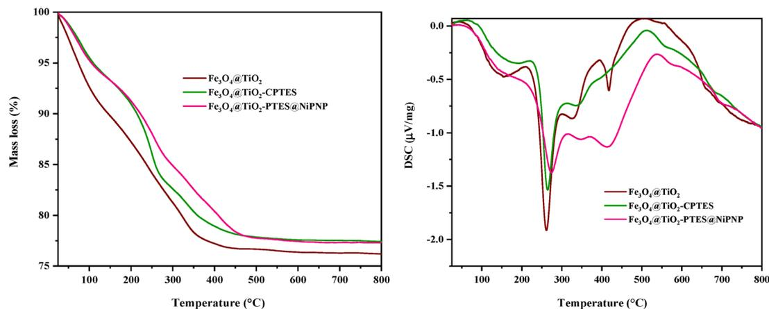
Fig. 4 (a) Thermogravimetric and (b) differential scanning calorimetry curves of  $\text{Fe}_3\text{O}_4$ ,  $\text{Fe}_3\text{O}_4@TiO_2$ ,  $\text{Fe}_3\text{O}_4@TiO_2\text{-CPTES}$ , and  $\text{Fe}_3\text{O}_4@TiO_2\text{-PTES@NiPNP}$ .
