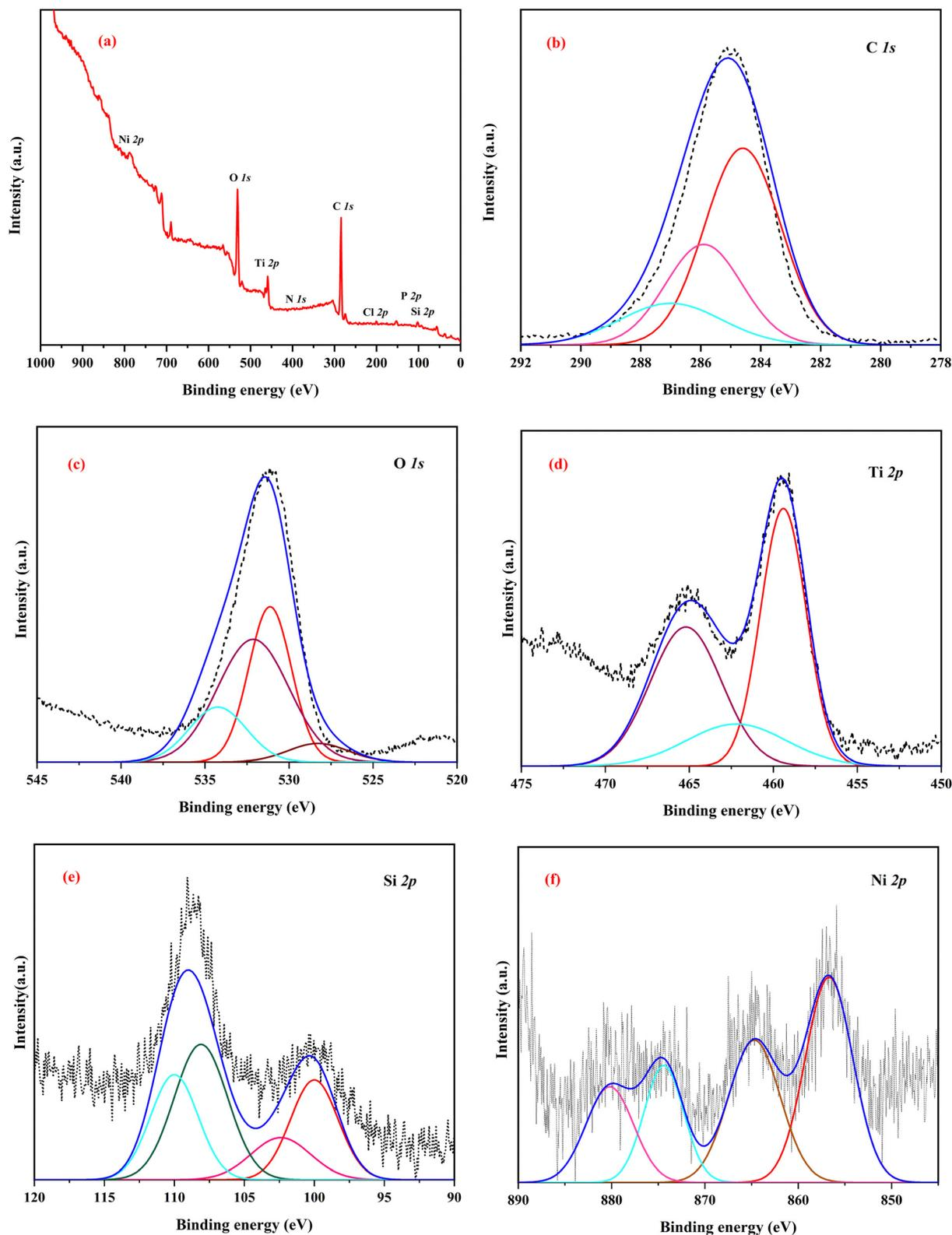
Fig. 9 (a) XPS survey spectra of  $\text{Fe}_3\text{O}_4@TiO_2\text{-PTES@NiPNP}$ . High-resolution XPS spectra of (b) C 1s, (c) O 1s, (d) Ti 2p, (e) Si 2p, and (f) Ni 2p.
