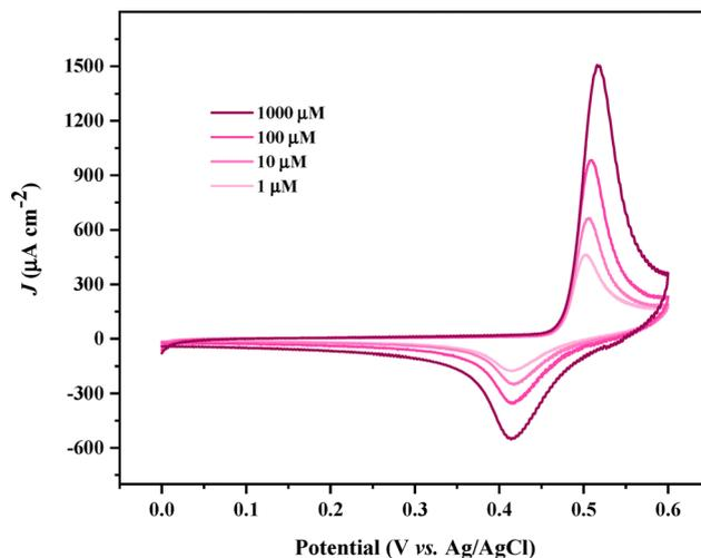
Fig. 15 Cyclic voltammograms of the  $\text{Fe}_3\text{O}_4@ \text{TiO}_2$ -PTES@NiPNP/GCE with Nafion in the presence of different concentrations of glucose (1, 10, 100, and 1000  $\mu\text{M}$ ) and 0.1 M NaOH at a scan rate of  $100 \text{ mV s}^{-1}$ .
