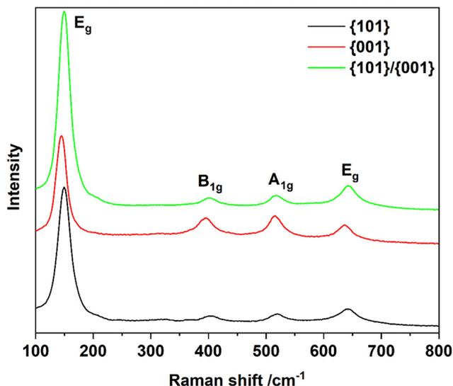
Fig. 3 Raman spectra of the synthesized TiO<sub>2</sub> samples.
