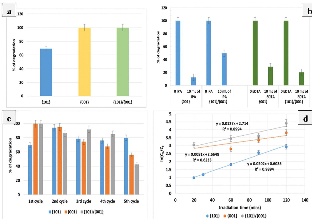
Fig. 6 (a) CR degradation percentage, (b) scavenging analysis, (c) reusability, and (d) kinetics of the photocatalytic degradation of the synthesized TiO<sub>2</sub> samples.
