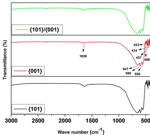
Fig. 2 FT-IR spectra of the synthesized TiO<sub>2</sub> samples.
