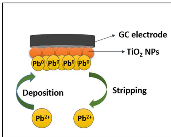
Fig. 9 Sensing mechanism of the {001}-modified TiO<sub>2</sub> sensor for Pb<sup>2+</sup> ion detection.
