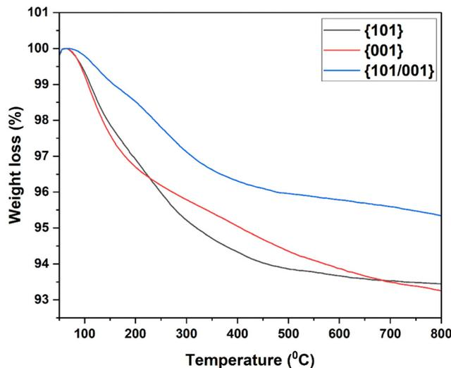
Fig. 4 Thermal weight loss of the synthesized TiO<sub>2</sub> samples.
