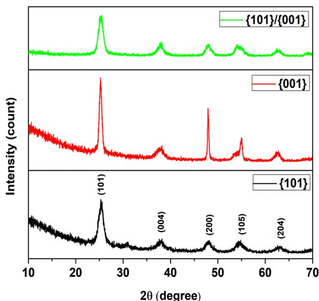
Fig. 1 XRD diffractogram of the synthesized TiO<sub>2</sub> samples.
