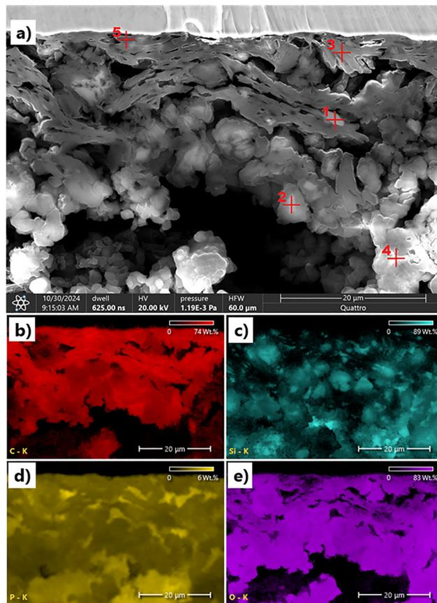
Fig. 6 (a) SEM cross-sectional image of Si/Gr anode after cycling (horizontal field width  $\approx 60 \mu\text{m}$ ). EDS maps of the distributions of (b) carbon, (c) silicon, (d) phosphorus, and (e) oxygen.
