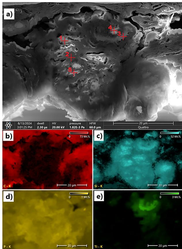
Fig. 5 (a) SEM cross-sectional image of Si-Tit/Gr anode after cycling (horizontal field width  $\approx 60 \mu\text{m}$ ). EDS maps of the distributions of (b) carbon, (c) silicon, (d) phosphorus, and (e) titanium.
