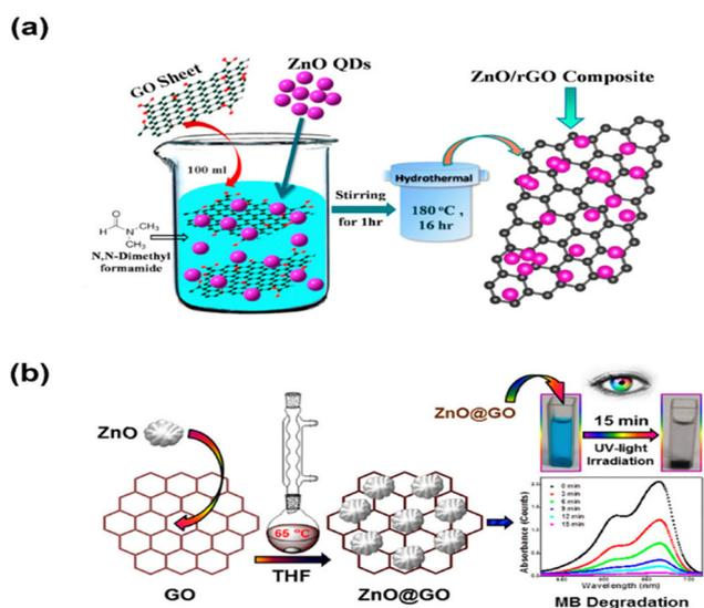
Fig. 22 Synthesis of graphene based hybrid material: (a) hydrothermal synthesis of  $\text{ZnO}/\text{GO}$  nanocomposites (reprinted from ref. 251, copyright@2016, Elsevier) and (b) solvothermal synthesis of  $\text{ZnO}/\text{GO}$  nanocomposites (reprinted from ref. 252, copyright@2024, MDPI).
