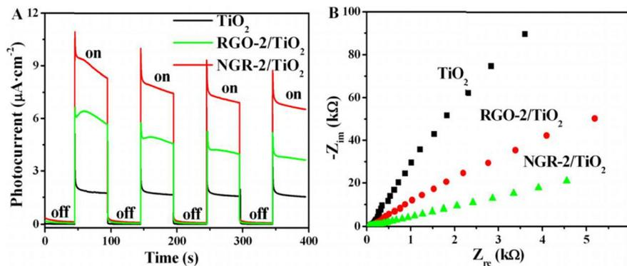
Fig. 21 (A) Transient photocurrent of  $\text{TiO}_2$ ,  $\text{RGO}/\text{TiO}_2$  and  $\text{NGR}/\text{TiO}_2$  to chopped light irradiation. (B) Nyquist plot of the electrochemical impedance spectra for  $\text{TiO}_2$ ,  $\text{RGO}/\text{TiO}_2$  and  $\text{NGR}/\text{TiO}_2$ . Reprinted from ref. 242, copyright@2025, Elsevier.
