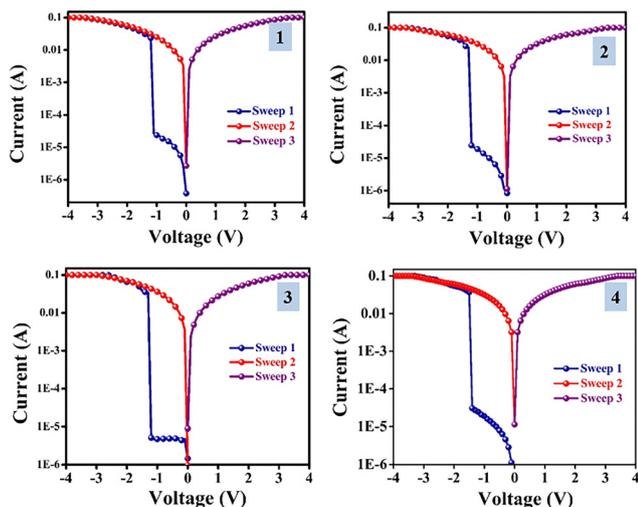
Fig. 7 Current–voltage ( $I$ – $V$ ) characteristics of the A– $\pi$ –D– $\pi$ –A-based devices (ITO/**1–2**/Ag) and D– $\pi$ –A-based devices (ITO/**3–4**/Ag).
