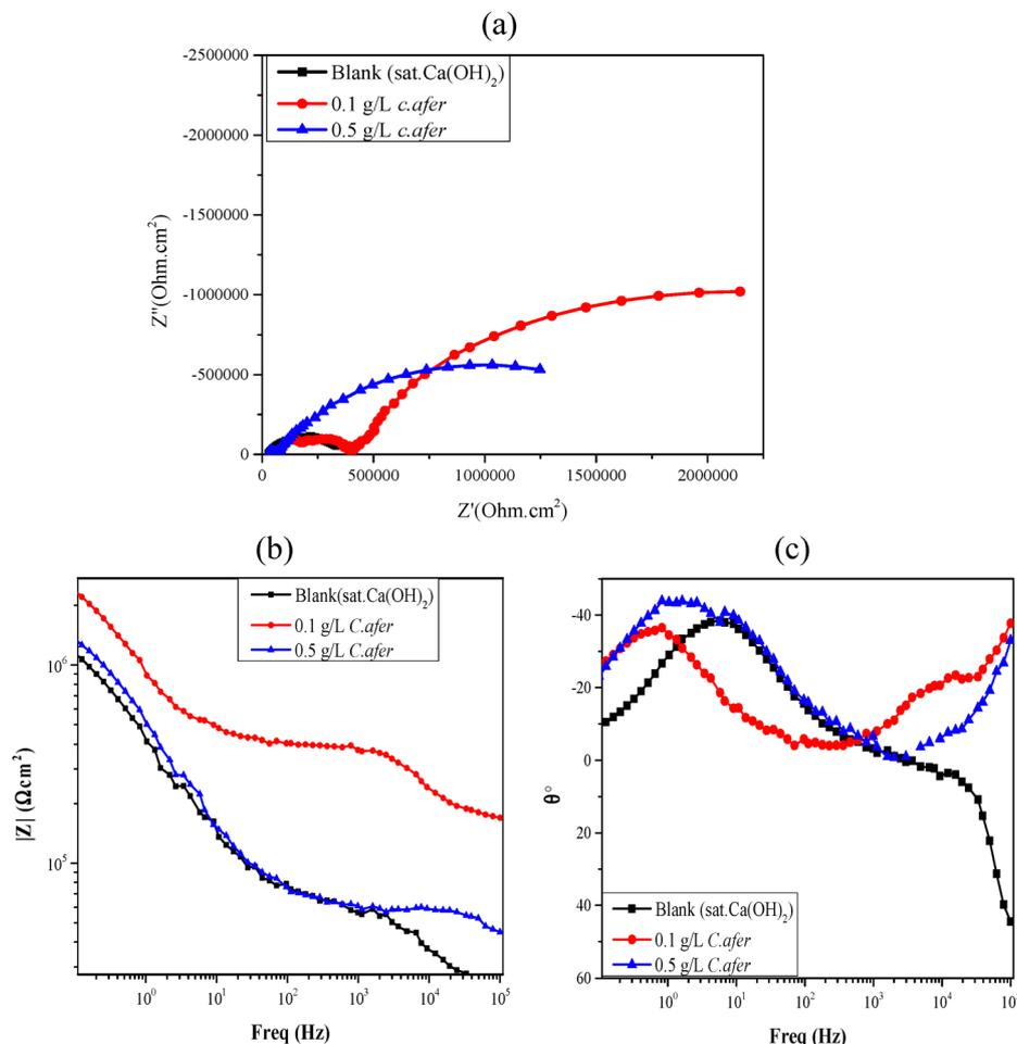
Fig. 4 (a) Nyquist, (b) Bode modulus, and (c) Bode phase angle plots of mild steel immersed in Ca(OH)<sub>2</sub> with different concentrations of *C. afer*.
