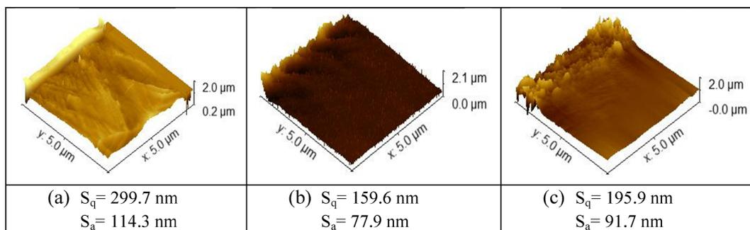
Fig. 7 3D AFM topographic view of the coupons immersed in (a) uninhibited Ca(OH)<sub>2</sub>, (b) Ca(OH)<sub>2</sub> with 0.5 g L<sup>-1</sup> of *C. albidum* ethanol extract and (c) Ca(OH)<sub>2</sub> with 0.5 g L<sup>-1</sup> of *C. afer* ethanol extract.
