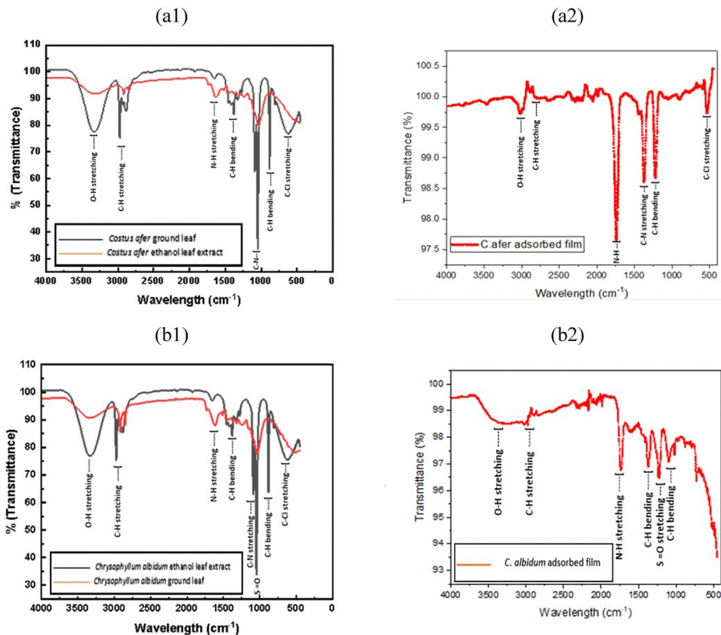
Fig. 6 FTIR spectra of the leaf powders and ethanol extract and corrosion products of (a1) (a2) *C. afer* and (b1) (b2) *C. albidum*.
