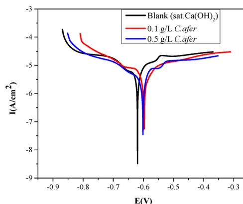
Fig. 2 Potentiodynamic polarization plots of mild steel exposed in saturated Ca(OH)<sub>2</sub> solution without and with different concentrations of *C. afer*.
