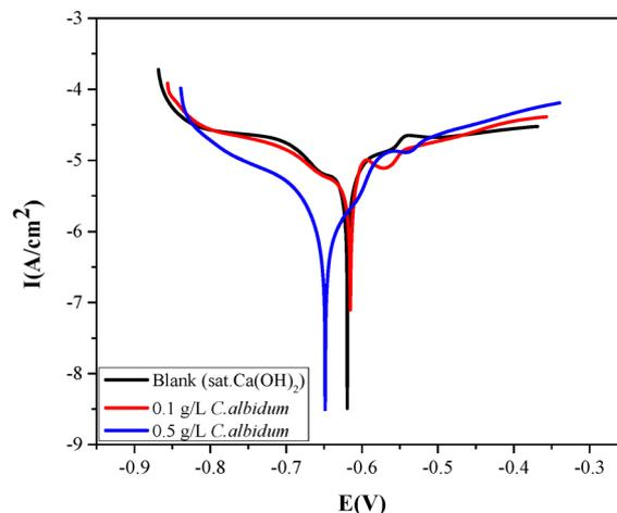
Fig. 3 Potentiodynamic polarization plots of mild steel exposed in saturated Ca(OH)<sub>2</sub> solution without and with different concentrations of *C. albidum*.
