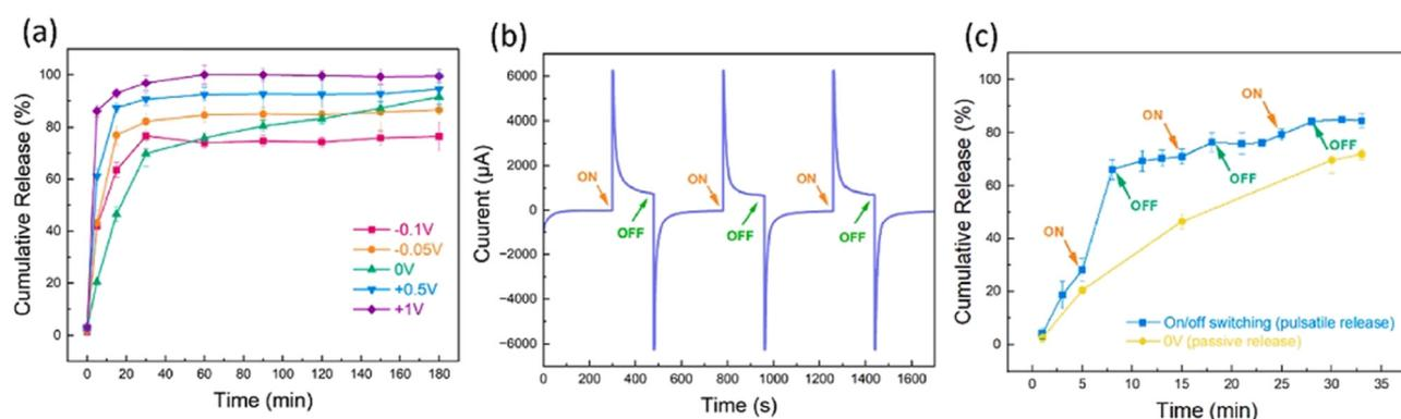
Fig. 8 (a) Cumulative release profiles of MB upon stimulation at  $-1.0$ ,  $-0.5$ ,  $+0.5$ , or  $+1.0$  V and without stimulation ( $0.0$  V). (b) Current–time response during the chronoamperometry experiment. (c) Pulsatile release profile of MB with on/off switching compared with its passive release ( $0.0$  V). Reproduced from ref. 86 licensed under Creative Commons CC-BY.
