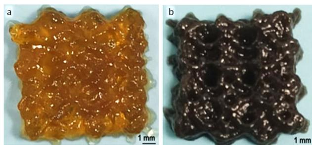
Fig. 7 Optical images of the 4D-bioprinted constructs (a) without magnetic nanoparticles (MNPs) as a control and (b) with MNPs (5 mg mL<sup>-1</sup>). Reproduced from ref. 36 licensed under Creative Commons CC-BY.
