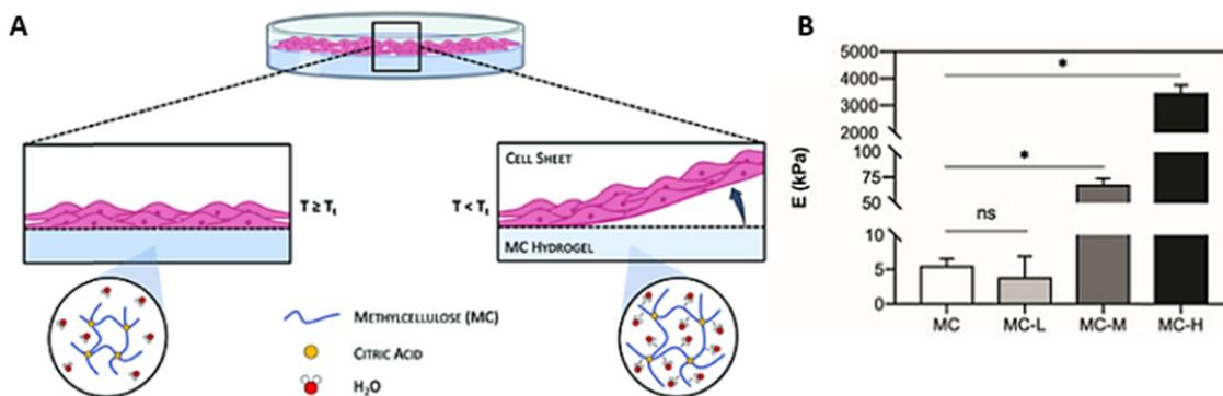
**Fig. 3** (A) Thermoresponsive methylcellulose (MC) hydrogels crosslinked with citric acid (CA) at  $T < T_t$  are in the sol (hydrophilic) state, and those at  $T \geq T_t$  are in the gel (hydrophobic) state. (B) Young's modulus ( $E$ ) of CA-crosslinked MC hydrogels. \* =  $p < 0.05$ . MC-L, MC-M, and MC-H indicate low, medium, and high degrees of crosslinking, respectively. Reproduced from ref. 29 licensed under Creative Commons Attribution (CC BY).
