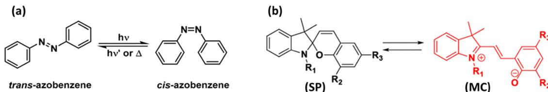
Fig. 6 Photoresponsive materials: (a) reversible photopolymerization of azobenzene in two states. Reproduced from ref. 55 licensed under Creative Commons Attribution (CC BY). (b) Reversible interconversion between ring-closed spiropyran (SP) and ring-opened merocyanine (MC). Reproduced from ref. 56 licensed under CC-BY-NC-ND 4.0.
