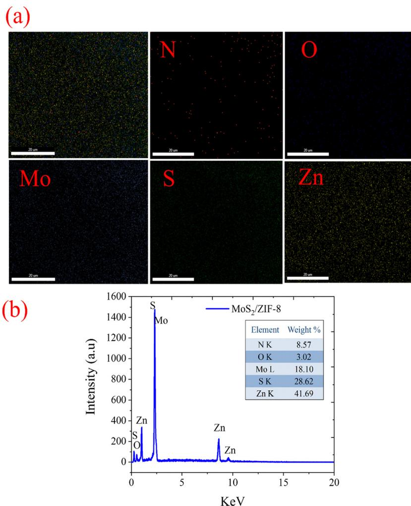
Fig. 3 (a) EDX-mapping and (b) EDX-line for the MoS<sub>2</sub>/ZIF-8 composite.
