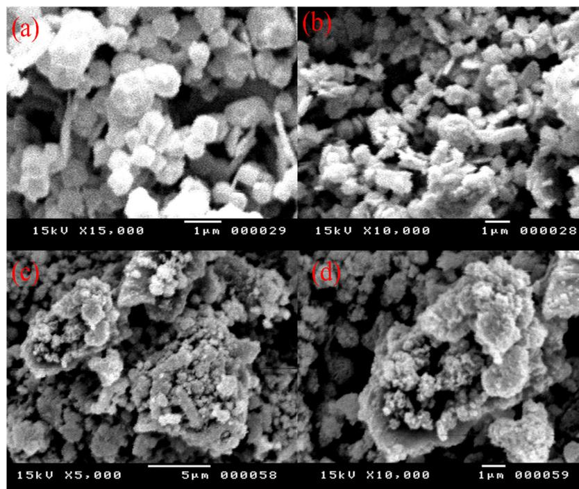
Fig. 2 SEM of (a) and (b) ZIF-8 and (c) and (d) the MoS<sub>2</sub>/ZIF-8 composite.
