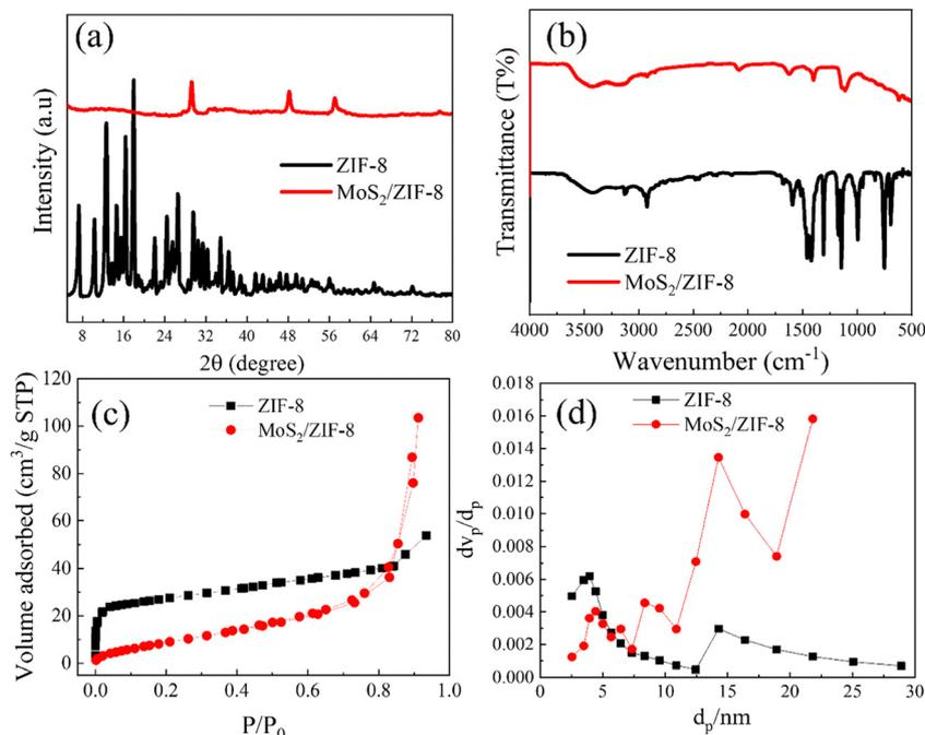
Fig. 1 (a) XRD pattern, (b) FT-IR spectra, (c) nitrogen adsorption–desorption isotherms, and (d) pore size distribution of ZIF-8 and the MoS<sub>2</sub>/ZIF-8 composite.
