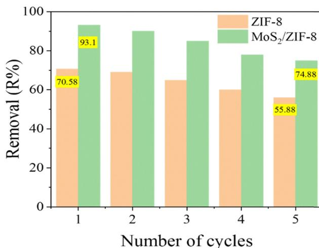
Fig. 12 The reusability of ZIF-8 and the MoS<sub>2</sub>/ZIF-8 composite toward MB adsorption.
