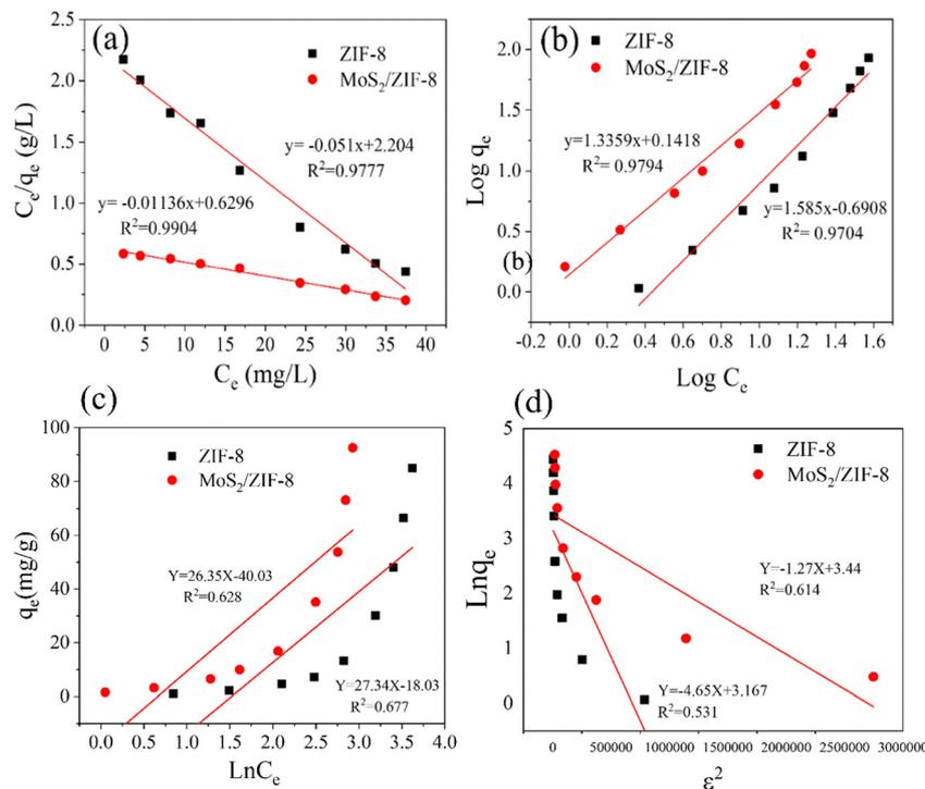
Fig. 9 Isotherm plots for the adsorption of MB onto ZIF-8 and the MoS<sub>2</sub>/ZIF-8 composite: (a) Langmuir, (b) Freundlich, (c) Temkin, and (d) Dubinin-Radushkevich (D-R) isotherm models.
