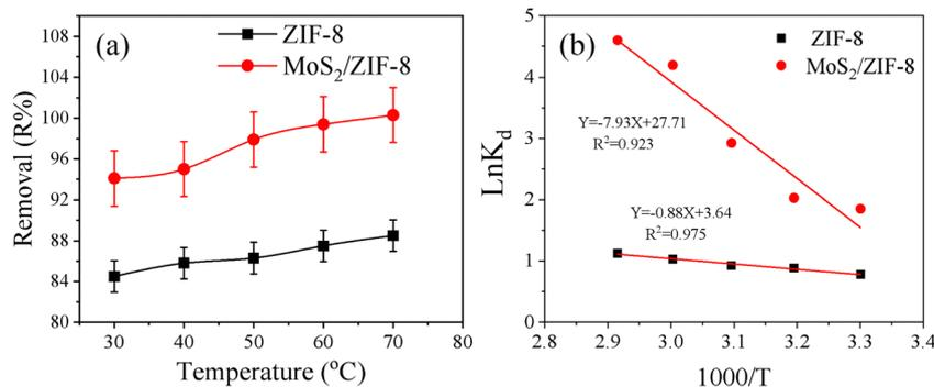
Fig. 11 (a) Effect of temperature on the removal of MB from aqueous solution and (b) Van't Hoff plots.
