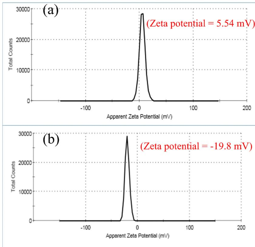
Fig. 5 Zeta potential the (a) ZIF-8 and (b) MoS<sub>2</sub>/ZIF-8 composite before MB adsorption.
