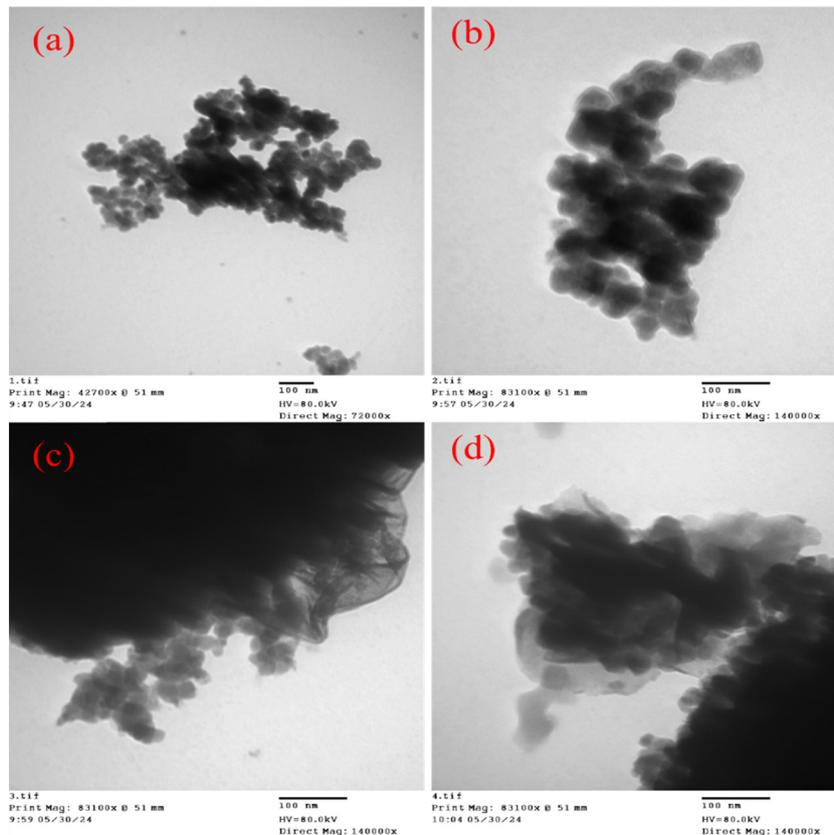
Fig. 4 TEM of (a) and (b) ZIF-8 and (c) and (d) the MoS<sub>2</sub>/ZIF-8 composite.
