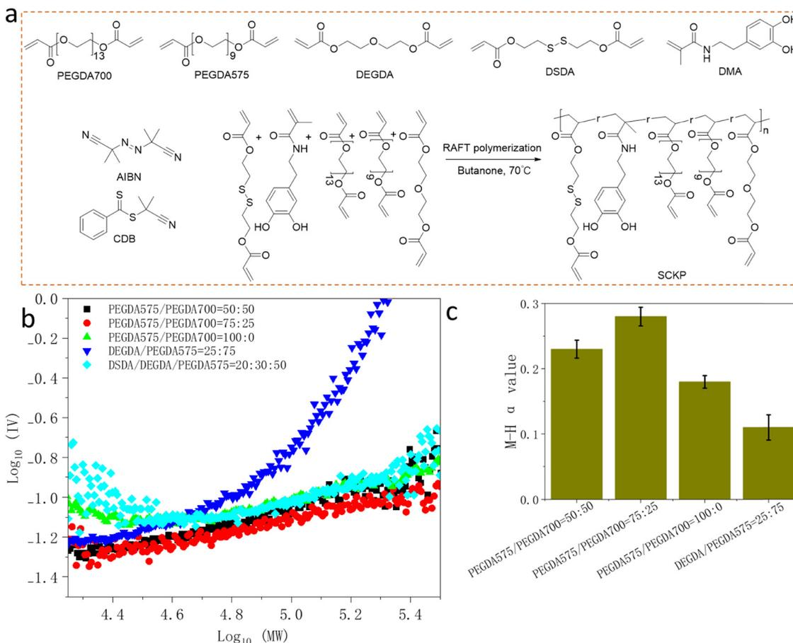
**Fig. 1** Synthesis and characterization of SCKPs. (a) Monomer and multivinyl monomers are copolymerized via RAFT polymerization to synthesize SCKPs. (b) The Mark–Houwink (M–H) plots for various SCKPs. (c) The  $\alpha$  values from the M–H plots for different SCKPs.
