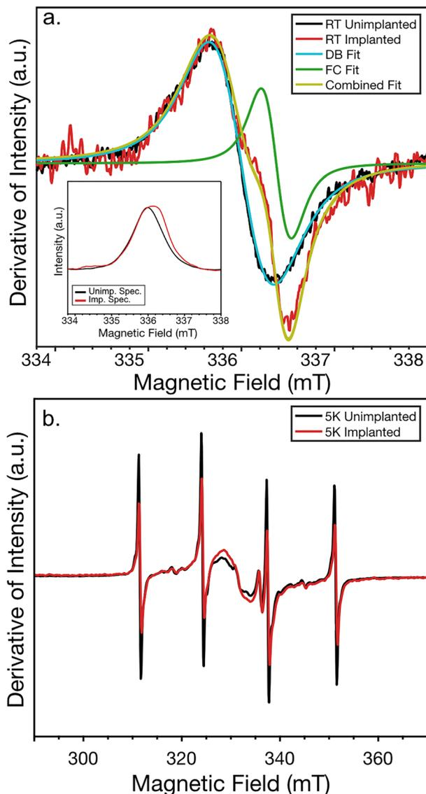
Fig. 8 (a) Room and (b) low (5 K) temperature CW-EPR of the  $\text{Na}_x\text{Si}_{136}$  film before implantation (black) and after  $10^{15}$  ions  $\text{cm}^{-2}$  fluence implantation and annealing (red). The spectra were acquired under the same parameters at 9.44 GHz over 40 scans at room temperature and 10 scans at low temperature and scaled by sample weight. The insets showing the integrated absorption spectra.
