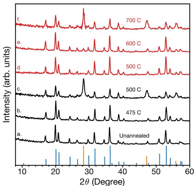
Fig. 4 XRD patterns  $\text{Na}_x\text{Si}_{136}$  film that were annealed at different conditions. The blue and orange lines represent the reference peaks of type II Si clathrate (ICDD 98-024-8181) and diamond silicon respectively. (a) Unannealed sample, (b) and (c) annealed in RTA and allowed to cool to room temperature under flowing argon, and (d)–(f) annealed in RTA and removed from annealer immediately and allowed to cool to room temperature in the atmosphere.
