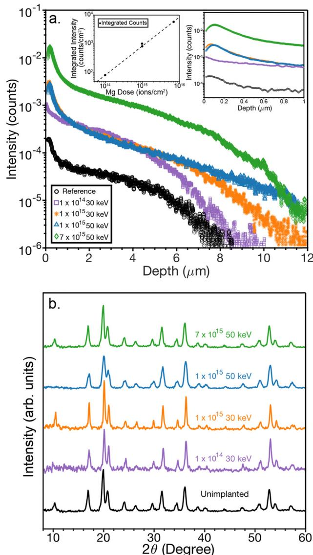
Fig. 5 (a) TOF-SIMS of broad beam implanted  $\text{Na}_x\text{Si}_{136}$  film samples. The right inset shows the first micron and left inset shows the integrated intensity as a function of fluence. (b) XRD of broad beam Mg implants of a  $\text{Na}_x\text{Si}_{136}$  film sample. The unimplanted sample is shown in black. As implant energy and fluence increases there is no noticeable change in phase to type I clathrate, a-Si, or d-Si.
