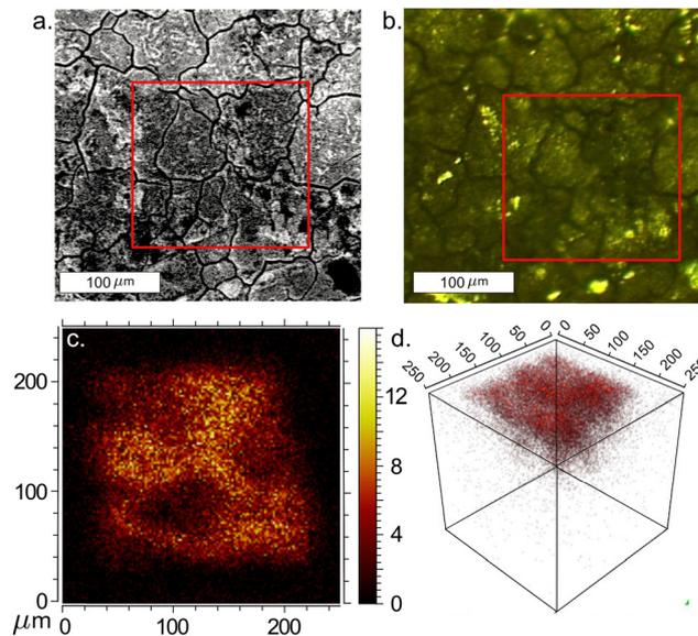
Fig. 2 (a) SEM image of Mg implantation into a Na<sub>x</sub>Si<sub>136</sub> film with high fluence (10<sup>15</sup> ions cm<sup>-2</sup>) outlined in red. (b) Raman confocal microscope image of the same area with the red box indicating grains used for matching locations for large area scans. (c) and (d) TOF-SIMS Mg intensity profile 2D and 3D image of the Mg implants.
