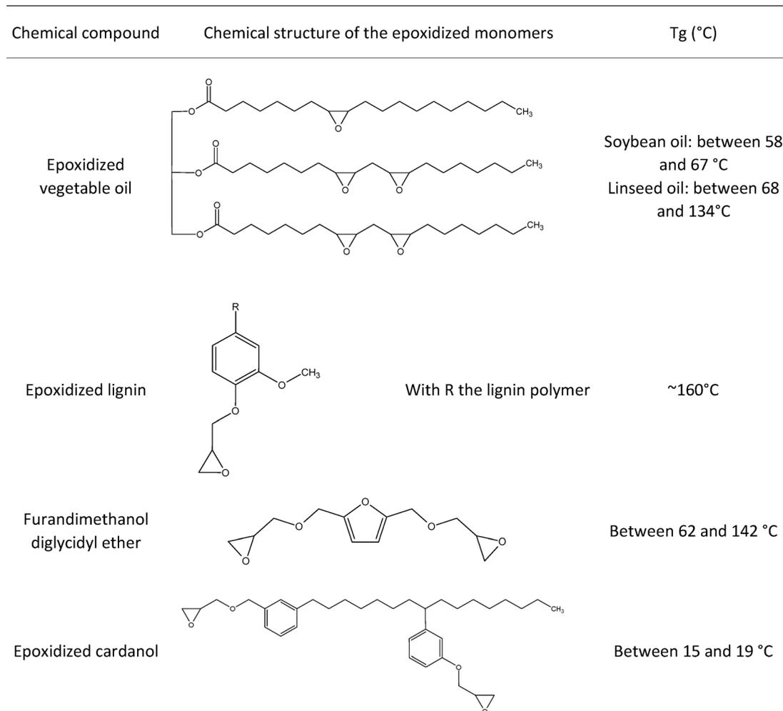
Fig. 4 Main bio-based epoxy systems.<sup>40,41</sup>
