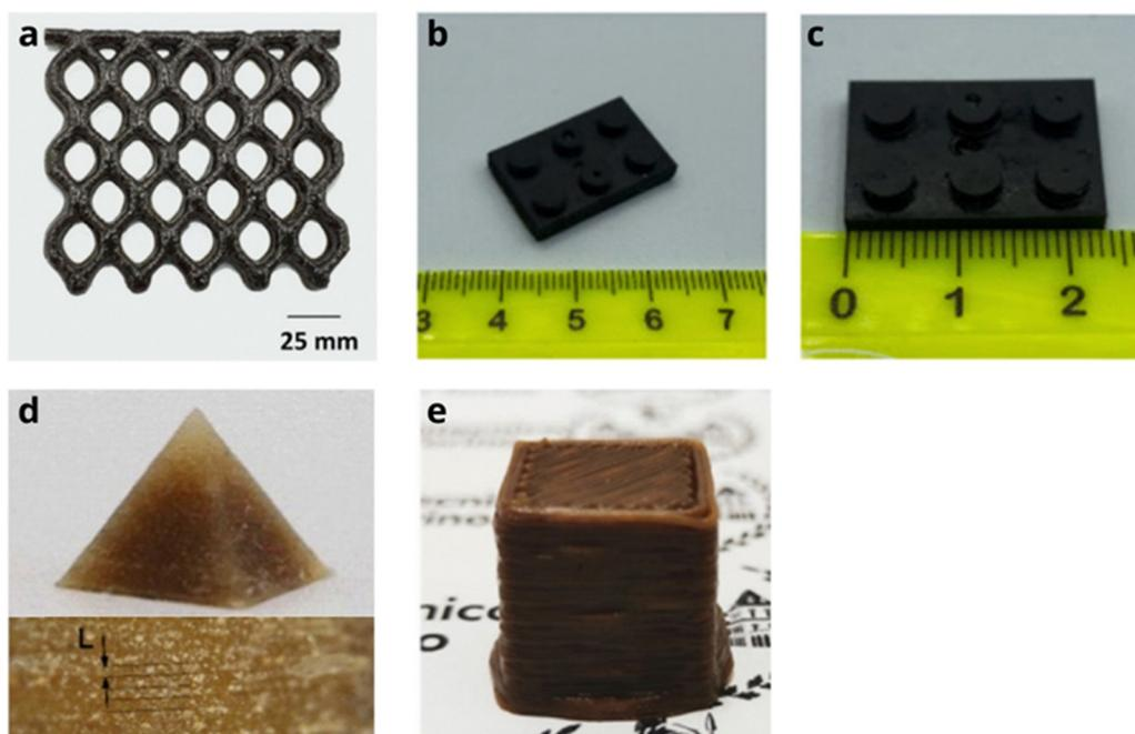
Fig. 5 (a) Commercial bio-epoxy resin print<sup>20</sup> (b) Resorcinol epoxy resin print Reproduced with permission from Elsevier, copyright 2022<sup>34</sup> (c) Furan dimethanol epoxy resin print Reproduced with permission from Elsevier, copyright 2022<sup>34</sup> (d) Linseed oil epoxy resin print and its optical analysis<sup>28</sup> (e) Cardanol epoxy resin print Reproduced with permission from Elsevier, copyright 2023.<sup>18</sup>
