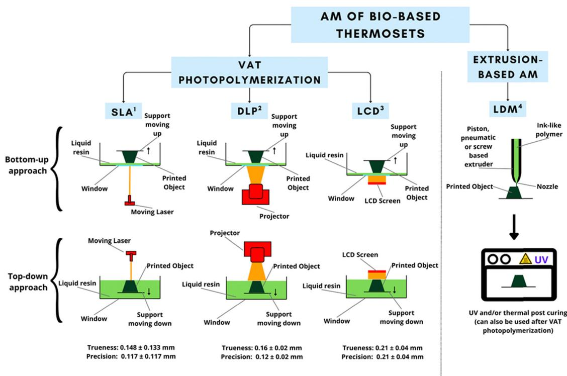
Fig. 1 Schematic representation of the different additive manufacturing techniques currently used for bio-based thermosets.<sup>1</sup> SLA: stereolithography,<sup>2</sup> DLP: digital light processing,<sup>3</sup> LCD: liquid-crystal display,<sup>4</sup> LDM: liquid deposition modelling.
