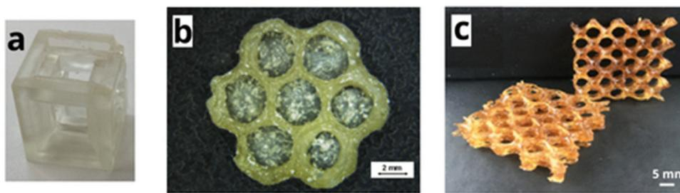
Fig. 9 (a) Levoglucosan thiol-ene resin print Reproduced with permission from American Chemical Society, copyright 2024<sup>61</sup> (b) Levoglucosan thiol-ene resin print<sup>57</sup> (c) Limonene thiol-ene resin print Reproduced with permission from American Chemical Society, copyright 2022.<sup>59</sup>
