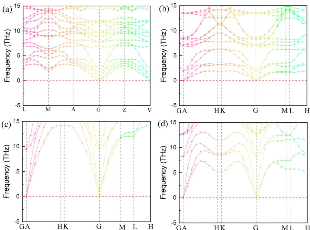
Fig. 2 Phonon spectra of (a) optimized, (b) -H, (c) -OH and (d) -CH<sub>3</sub> decorated 2-(111) planar T-carbons.
