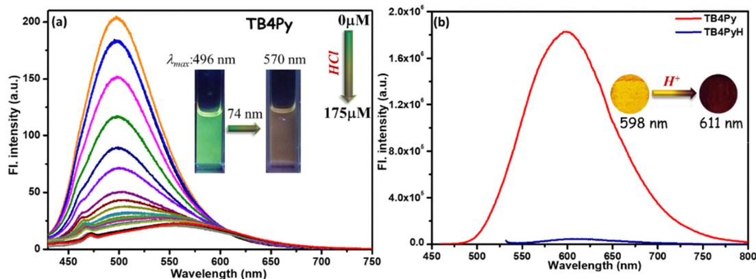
Fig. 4 The emission spectra of **TB4Py** in (a) solution (10  $\mu$ M in 1,4-dioxane) upon the gradual addition of  $10^{-2}$  M HCl [ $\lambda_{\text{ex}} = 407$  nm] and (b) the solid state before and after exposure to 50  $\mu$ L of HCl vapor for 30 minutes in a closed vial.
