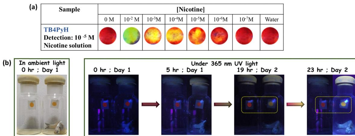
Fig. 9 (a) Images taken after treating **TB4PyH** dye-dispersed paper with various nicotine concentrations under a 365 nm UV lamp, (b) application of the probe in detecting the freshness of fish and chicken.
