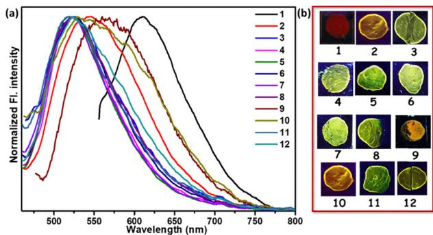
Fig. 6 (a) Normalized FL spectra of **TB4PyH** thin film before and after exposure to different amine vapors ( $\lambda_{\text{exc}}$ : 432 nm). (b) Emission change in the thin film state (1) **TB4PyH**; after exposing to (2) ammonia; (3) butylamine; (4) ethylenediamine; (5) 1,3-DAP; (6) PUT; (7) CAD; (8) 1,6-diaminohexane; (9) 2-phenylethylamine; (10) *N*-ethyl diisopropylamine; (11) SPM; and (12) spermine; All the images were taken under a 365 nm UV lamp.
