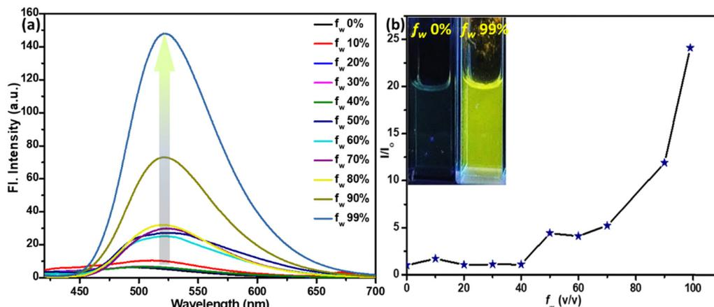
Fig. 3 (a) The emission spectra of **TB4Py**,  $\lambda_{\text{ex}} = 406$  nm; (b) the  $I/I_0$  plot [ $I_0$ : FL intensity before the addition of water,  $I$ : FL intensity after the addition of water]. The concentration of the probe is  $10 \mu\text{M}$ . Inset: the image was taken at  $f_w = 0\%$  and  $f_w = 99\%$  for **TB4Py** under a 365 nm UV lamp.
