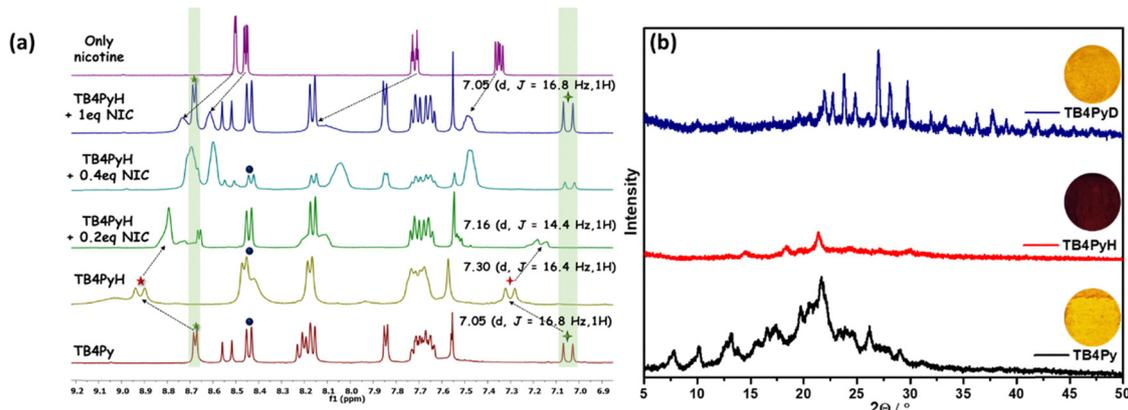
Fig. 7 (a) The partial  $^1\text{H}$ -NMR spectra (only aromatic part) of **TB4Py**, **TB4PyH**, and after the addition of 0.2 equiv., 0.4 equiv., and 1 equiv. of NIC, dissolved in  $\text{DMSO}-d_6$ ; (b) changes in the PXRD pattern of **TB4Py** before and after HCl and PUT vapor exposure for 15 minutes.
