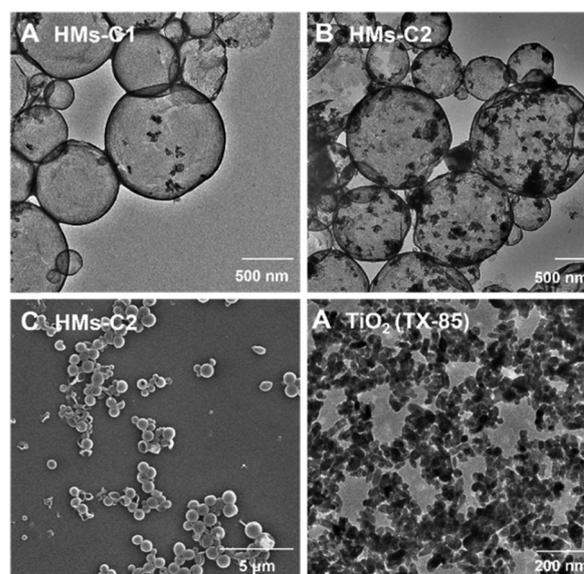
**Fig. 8** (A) TEM images of CNCs/TiO<sub>2</sub> hollow microspheres. (B) TEM images of Cin-CNCs/TiO<sub>2</sub> hollow microspheres. (C) SEM images of Cin-CNCs/TiO<sub>2</sub> hollow microspheres. (D) TEM images of TiO<sub>2</sub> nanoparticles (refer to Table S1 for more details).
