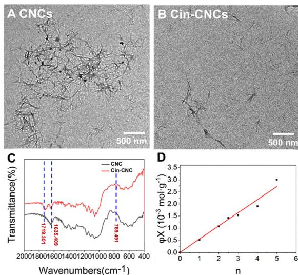
**Fig. 2** TEM images of (A) pristine CNCs and (B) Cin-CNCs. (C) FTIR spectra of pristine CNCs and Cin-CNCs synthesized at a weight ratio of CNCs to cinnamoyl chloride of 2:5. (D) Correlation between the parameter “ $n$ ” and the grafting fraction “ $\phi X$ ”.
