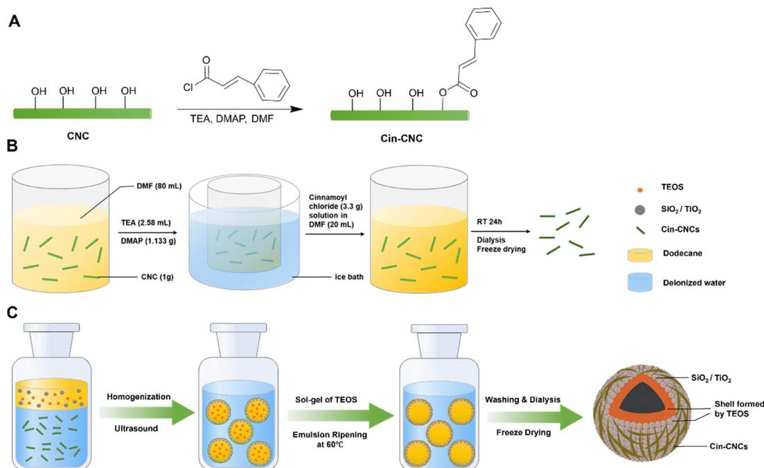
**Fig. 1** (A) Synthesis of a Cin-CNCs-based Pickering emulsifier *via* acylation of cellulose nanocrystals (CNCs) with cinnamoyl chloride; (B) schematic of the synthetic route for Cin-CNCs. (C) Formation mechanism of hollow microspheres co-stabilized by Cin-CNCs and SiO<sub>2</sub> (or TiO<sub>2</sub>) nanoparticles.
