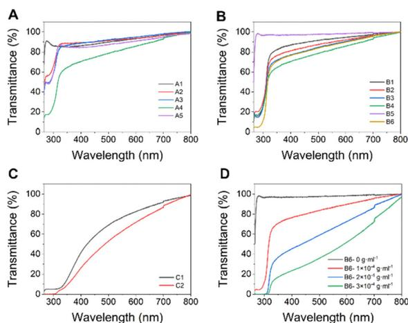
Fig. 9 (A) and (B) UV-vis transmittance spectra of Cin-CNCs/SiO<sub>2</sub> hollow microspheres. (C) UV-vis transmittance spectra of Cin-CNCs/TiO<sub>2</sub> hollow microspheres (the concentration of hollow microspheres was  $1 \times 10^{-4} \text{ g mL}^{-1}$ ). (D) Effect of the Cin-CNCs/SiO<sub>2</sub> hollow microsphere concentration on the optical transmittance at different UV wavelengths.
