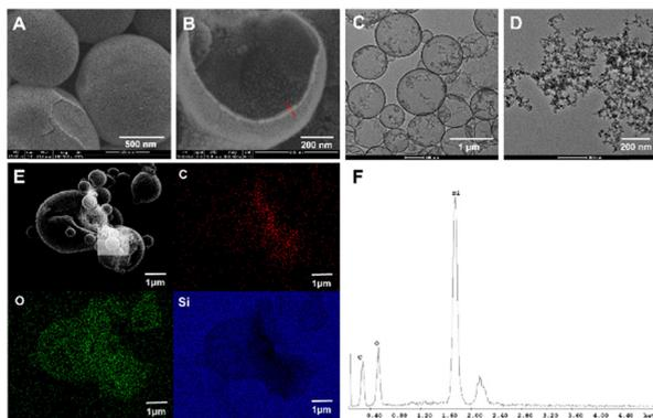
Fig. 4 (A) and (B) SEM images and (C) TEM images of Cin-CNCs/SiO<sub>2</sub> hollow microspheres. (D) TEM images of SiO<sub>2</sub> nanoparticles (Aerosil R974). (E) EDX elemental scanning and mapping, and (F) EDX spectrum plots of Cin-CNCs/SiO<sub>2</sub> hollow microspheres.
