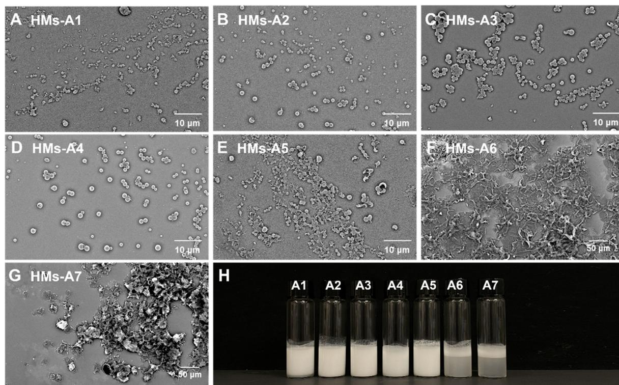
Fig. 6 (A)–(G) SEM images and (H) appearance photos of Cin-CNCs/SiO<sub>2</sub> hollow microspheres prepared using pristine CNCs (A1) and Cin-CNCs with six different grafting fractions (A2: 0.17; A3: 0.36; A4: 0.47; A5: 0.51; A6: 0.63; A7: 1.00) and equal amounts of SiO<sub>2</sub> nanoparticles (refer to Table S1 for more details).
