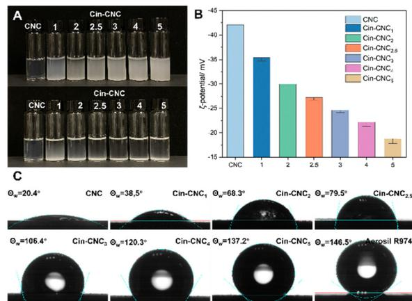
**Fig. 3** (A) Optical images of CNC and Cin-CNC dispersions ( $1 \times 10^{-3} \text{ g mL}^{-1}$ ) in water immediately after preparation and after 2 hours. (B) Zeta potentials of CNCs and Cin-CNCs with different grafting fractions at identical pH values. (C) Contact angles of SiO<sub>2</sub> nanoparticles (Aerosil R974), CNCs, and Cin-CNCs with varying grafting fractions.
