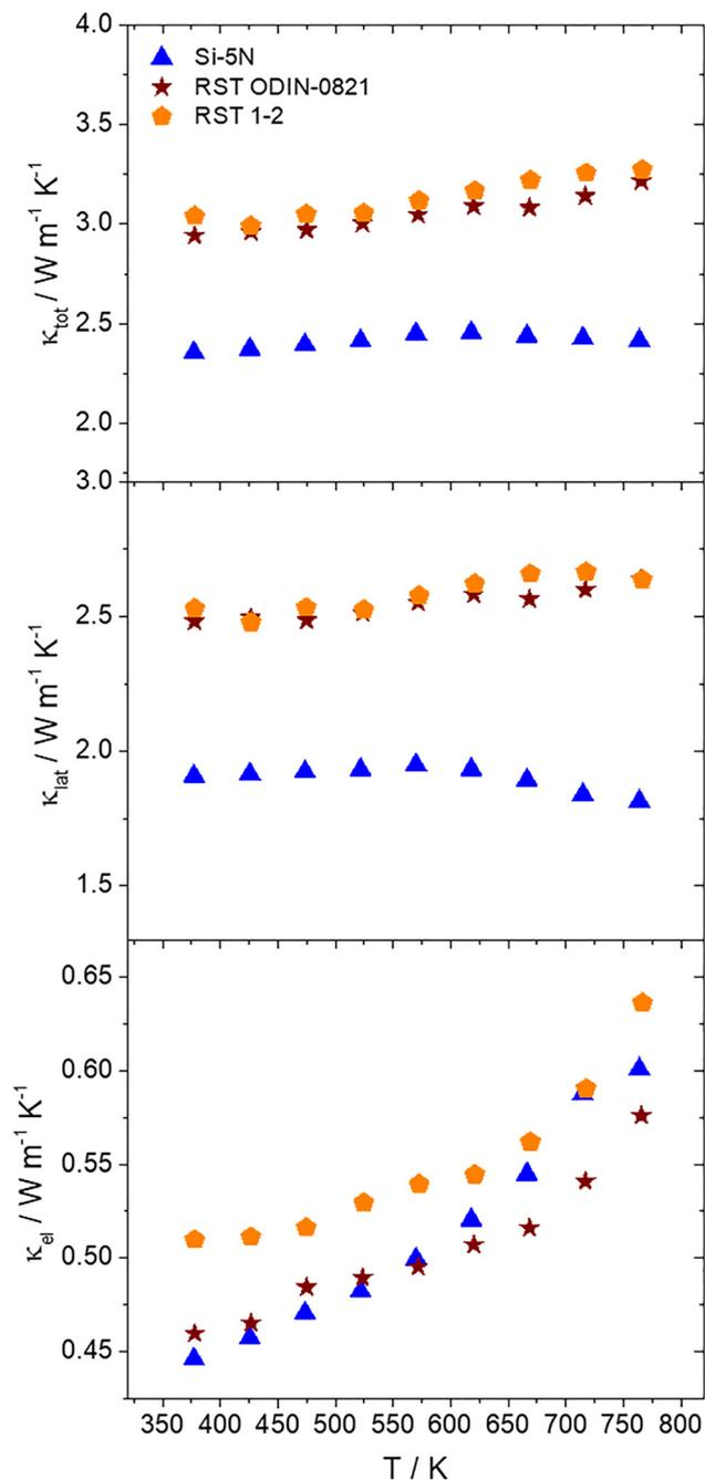
Fig. 13 Total ( $\kappa_{\text{tot}}$ ), lattice ( $\kappa_{\text{lat}}$ ) and electronic ( $\kappa_{\text{el}}$ ) thermal conductivities as a function of temperature for the  $\text{Mn}(\text{Si}_{0.975}\text{Al}_{0.025})_{1.75}$  phases based on Si-5N and the two Si kerfs, RST ODIN-0821 and RST 1–2.
