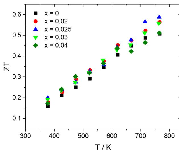
Fig. 9  $ZT$  as a function of temperature for the  $\text{Mn}(\text{Si}_{1-x}\text{Al}_x)_{1.75}$  phases ( $0 \leq x \leq 0.04$ ).
