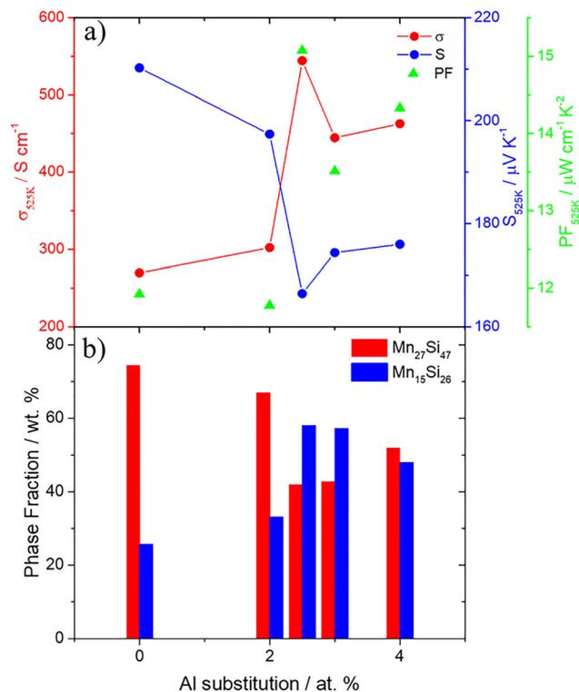
Fig. 7 (a) Electrical conductivity, Seebeck coefficient and PF at a constant temperature of 525 K as a function of Al substitution and (b) evolution of phase fraction of two phases,  $\text{Mn}_{27}\text{Si}_{47}$  and  $\text{Mn}_{15}\text{Si}_{26}$ , with Al substitution, as derived from the Rietveld refinements.
