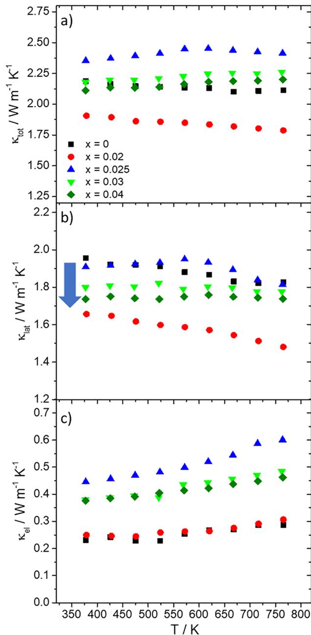
Fig. 8 (a) Total ( $\kappa_{\text{tot}}$ ), (b) lattice ( $\kappa_{\text{lat}}$ ) and (c) electronic ( $\kappa_{\text{el}}$ ) thermal conductivity as a function of temperature for the  $\text{Mn}(\text{Si}_{1-x}\text{Al}_x)_{1.75}$  phases ( $0 \leq x \leq 0.04$ ).
