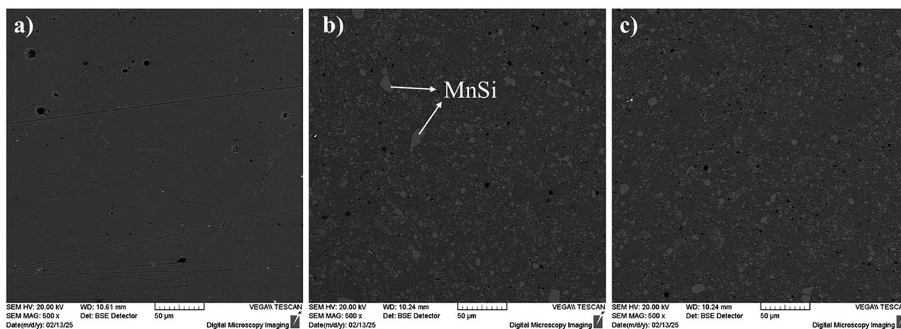
**Fig. 11** Backscattering SEM images for the  $\text{Mn}(\text{Si}_{0.975}\text{Al}_{0.025})_{1.75}$  phases based on (a) Si-5N, (b) RST 1–2 and (c) RST ODIN-0821. The scale bar in these images is 50  $\mu\text{m}$ .
