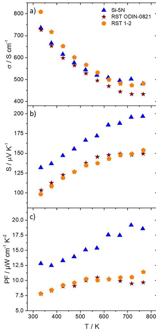
Fig. 12 (a) Electrical conductivity, (b) Seebeck coefficient and (c) PF as a function of temperature for the  $\text{Mn}(\text{Si}_{0.975}\text{Al}_{0.025})_{1.75}$  phases based on Si-5N and the two Si kerfs, RST ODIN-0821 and RST 1–2.
