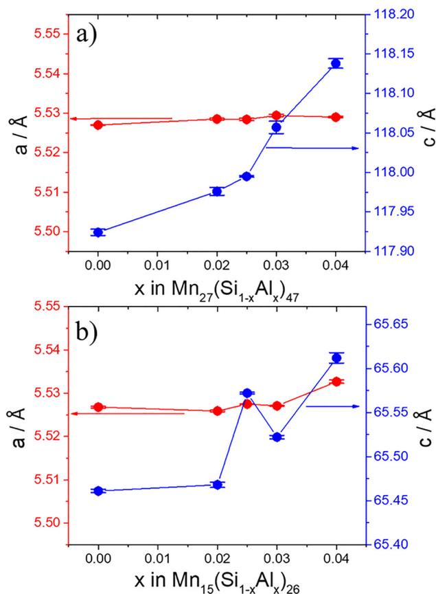
**Fig. 4** Refined lattice constants as a function of Al content for the two NCL phases of (a)  $\text{Mn}_{27}(\text{Si}_{1-x}\text{Al}_x)_{47}$  ( $0 \leq x \leq 0.04$ ) and (b)  $\text{Mn}_{15}(\text{Si}_{1-x}\text{Al}_x)_{26}$  ( $0 \leq x \leq 0.04$ ), derived from the powder XRD Rietveld refinements of the phase mixture model.
