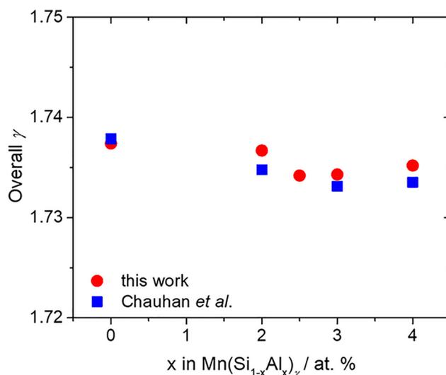
**Fig. 5** Calculated overall  $\gamma$  (red spheres) across the  $\text{Mn}(\text{Si}_{1-x}\text{Al}_x)_\gamma$  series derived by the quantitative Rietveld analysis of the phase mixture model as a function of Al content in comparison with the results obtained from the work of Chauhan *et al.* (blue squares).<sup>28</sup>
