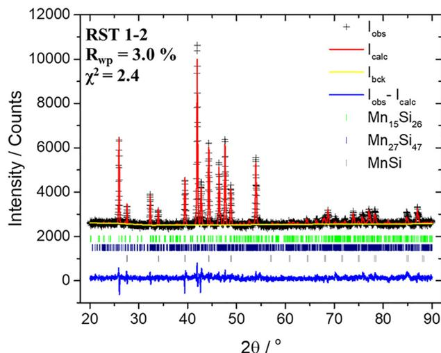
**Fig. 10** Powder XRD Rietveld refinement profile of  $\text{Mn}(\text{Si}_{0.975}\text{Al}_{0.025})_{1.75}$  based on RST 1–2 silicon kerf for the phase mixture structural model. Final observed (black crosses), calculated (red solid line), calculated background (yellow line) and difference (blue line). Reflection positions for the  $\text{Mn}_{15}\text{Si}_{26}$ ,  $\text{Mn}_{27}\text{Si}_{47}$  and  $\text{MnSi}$  phases are marked with green, navy and gray colors, respectively.
