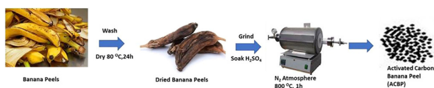
Scheme 1 Schematic diagram of the synthesis of activated carbon banana peels (ACBP).
