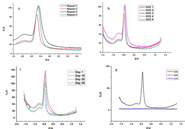
**Fig. 8** DPV response of 1 mM CPX on GCE/ACBP-BiVO<sub>4</sub> in PBS (a) repeatability for 4 successive measurements, (b) reproducibility and (c) long-term storage stability, (d) interference studies on 1 mM CPX on GCE/ACBP-BiVO<sub>4</sub> in PBS DPV parameters:  $E_{\text{start}} = -1.6$  V;  $E_{\text{end}} = 1.3$  V; pulse amplitude = 50.0 mV;  $E_{\text{step}} = 4$ , pulse time = 10 ms, scanrate = 100 mV s<sup>-1</sup>, equilibrium time = 5 s.
