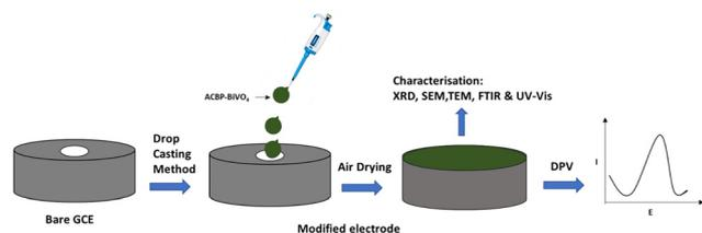
**Scheme 3** Modification of GCE electrode with ACBP-BiVO<sub>4</sub> by drop casting method.
