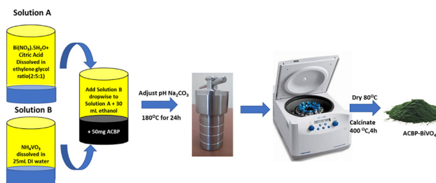
Scheme 2 Schematic diagram of the synthesis of activated carbon bismuth vanadate (ACBP- \text{BiVO}_4 ).
