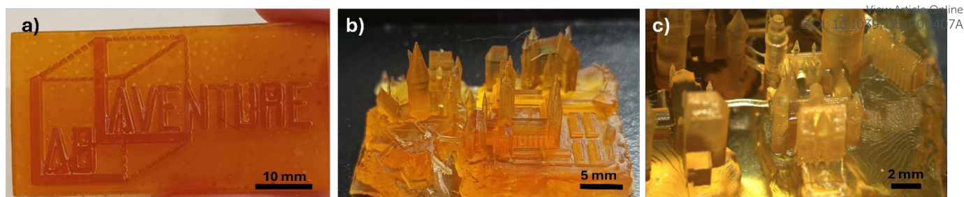
Figure 7. 3D printing of a) Lab Laventure logo, b) and c) Hogwarts castle.
