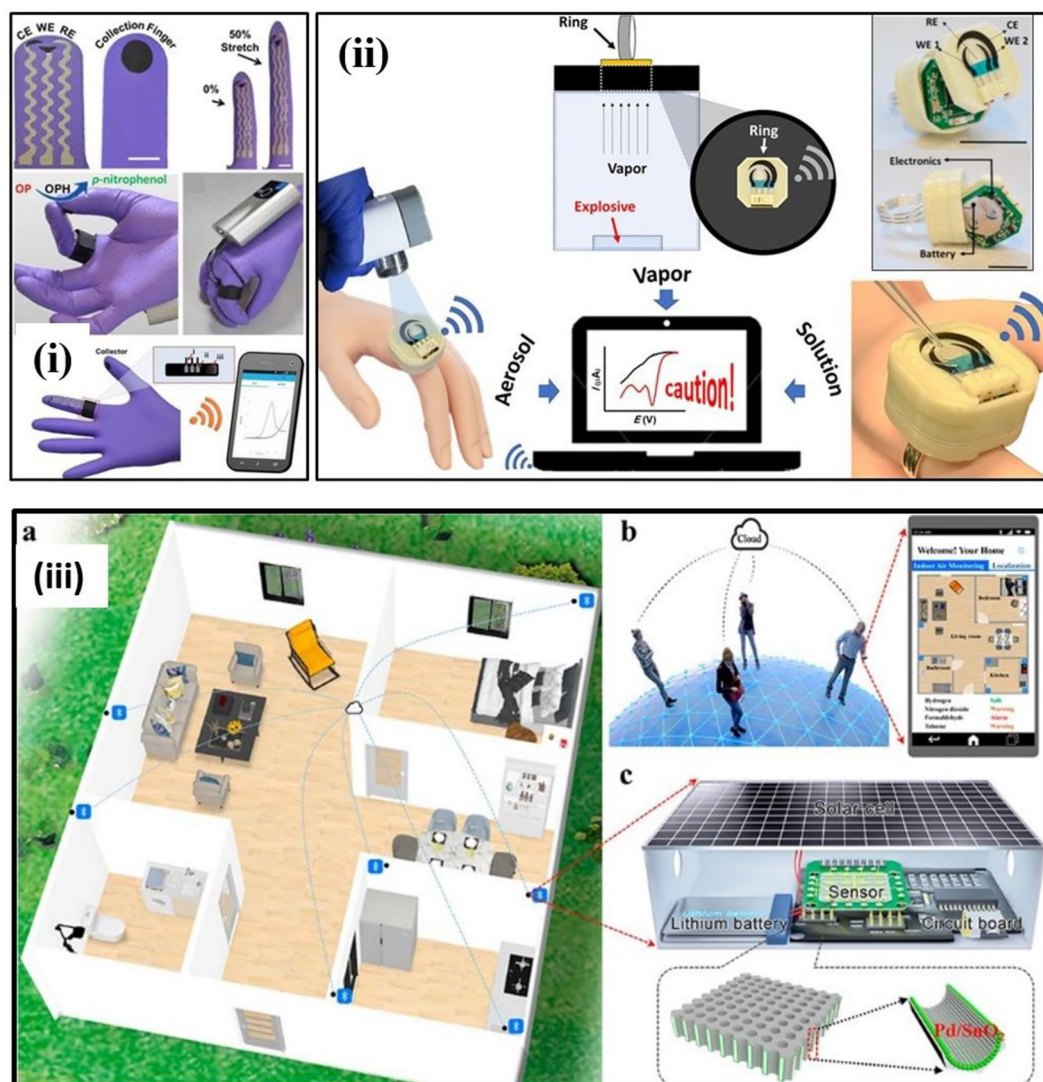
Fig. 12 (i) Schematic of a wearable glove biosensor system featuring screen-printed stretchable electrodes, a swipe-based sampling pad, and a flexible wireless electrochemical module for real-time detection of organophosphate compounds. 178 (Reproduced with permission from Mishra et al. , ACS Sens. , 2017, 2, 553–560. https://pubs.acs.org/doi/10.1021/acssensors.7b00051 ); (ii) schematic of a ring-type wearable sensor with flexible polymer substrate and integrated wireless module for real-time detection. 179 (Reproduced with permission from Sempionatto et al. , ACS Sens. , 2017, 2, 1470–1478. https://pubs.acs.org/doi/10.1021/acssensors.7b00603 Copyright © 2017 American Chemical Society.) (iii) Illustrates the layout and components of the SINGOR system (a) shows the spatial deployment of the sensor array within a smart home environment for real-time gas leakage detection. (b) depicts remote gas monitoring through a smartphone interface enabled via Bluetooth. (c) highlights the modular integration of key components, including a solar energy module, lithium-ion battery, and a 3D Pd/SnO 2 gas sensor array. 180 (Adapted with permission from Song et al. , ACS Nano , 2021, Copyright 2021 American Chemical Society.)
