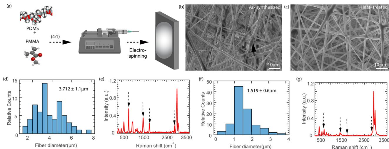
**Fig. 1** Electrospinning of PDMS (ePDMS). (a) Schematic showing the electrospinning of PDMS using PMMA as the carrier polymer. (b) SEM micrograph of the AS-ePDMS. (c) SEM micrograph of the HT-ePDMS membranes. Mean fiber diameter of the (d) AS-ePDMS membranes and (f) HT-ePDMS. Raman analysis of the ePDMS membranes: (e) AS-ePDMS, (g) HT-ePDMS. The arrows in (e) and (g) correspond to the Raman spectrum of PMMA.
